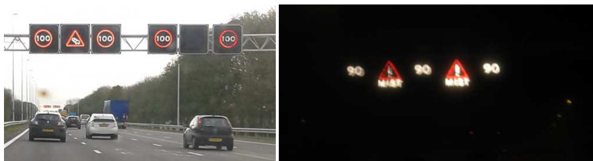
Figure 2.4 Example of two additional information signs (left: traffic jam ahead, right: attention; fog) mounted on gantries above the motorway between MSI with speed limits.
