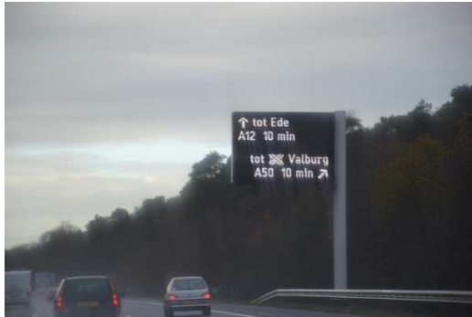
Figure 2.8 Example of a roadside DRIP showing travel times.
