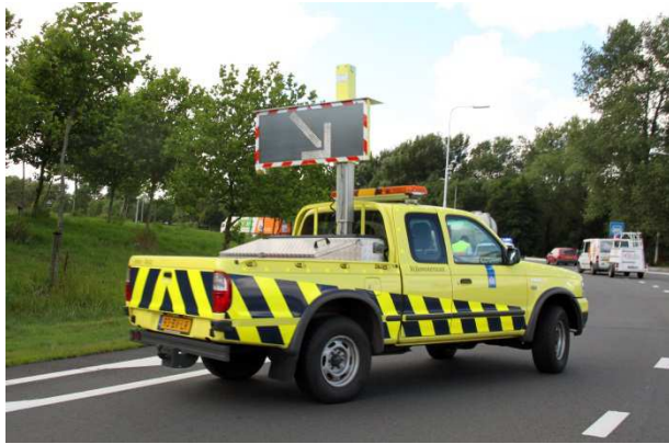
Figure 2.11 Example of a car DRIP mounted on a road inspector vehicle from Rijkswaterstaat.
