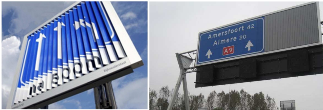
Figure 2.6 Examples of multisigns (rotary prism signs) alongside the road (left) and above the road (right).
