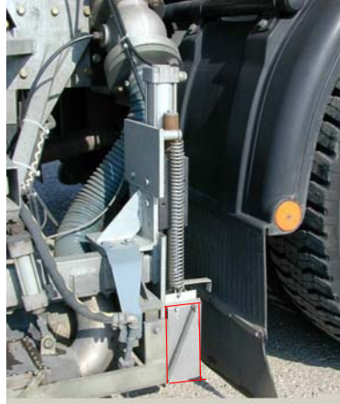
Figure 5: The texture measurement device as part of the Austrian RoadSTAR road and pavement monitoring vehicle, which also performs measurements of skid resistance, longitudinal and transversal evenness
