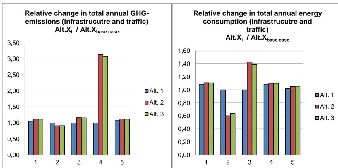
Figure 7: The five scenarios that give the biggest change in total GHG-emissions and energy consumption (infrastructure and traffic). The relative change from the base case scenario is displayed:  $Alt.X_i / Alt.X_{base\ case}$ , where  $Alt.X_i$  is the GHG-emissions or energy consumption for scenario  $i$ , where  $i = 1-5$  corresponding to the scenarios on page 16, and  $Alt.X_{base\ case}$  is the GHG-emissions or the energy consumption in the base case scenario.
