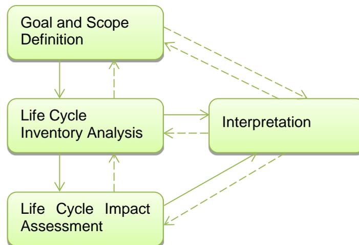
Figure 1: Overview of the LCA-procedure. The arrows indicate the order in which the procedural steps are performed. The broken arrows indicate possible iterations (adapted from Baumann and Tillman, 2004).
