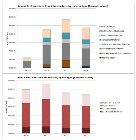
*Figure 7: Illustration of a potential outcome of a comparison between three road alternatives using LICCER.*
