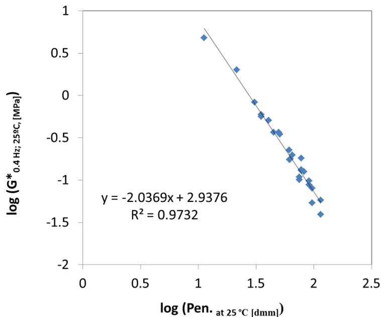
Figure 4.24 Correlation between the complex modulus at 25 °C and 0.4 Hz and Pen. Value for six binder groups (in total 19 binders)
