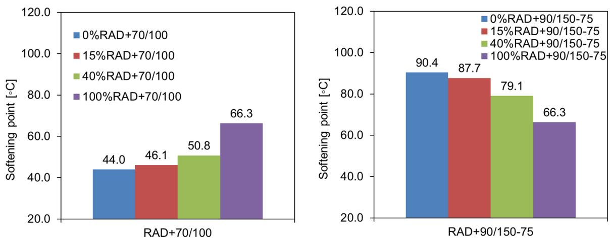
Figure 4.8 Softening point for binder groups of RAD+70/100 (left) and RAD+90/150-75 (right)
