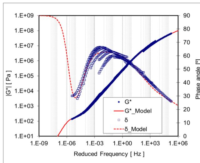
Figure 3.3 Master curves of PMB KR and its MHS model
