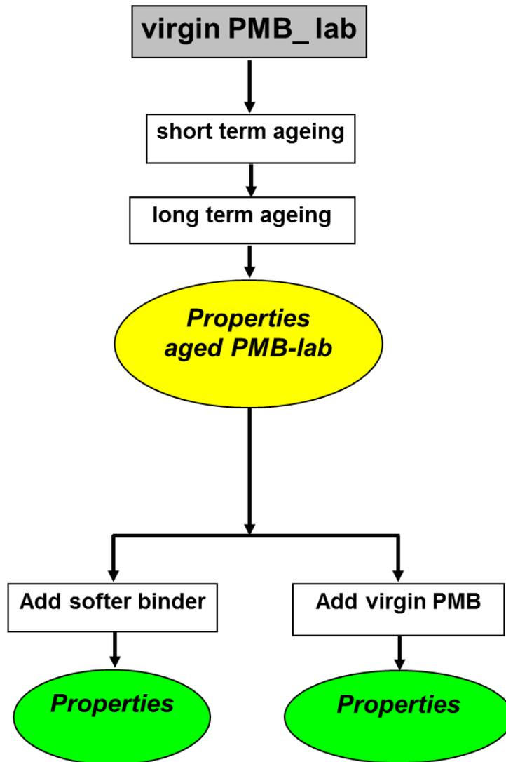
Figure 1.1 Flow chart for the research on PMB\_RA
