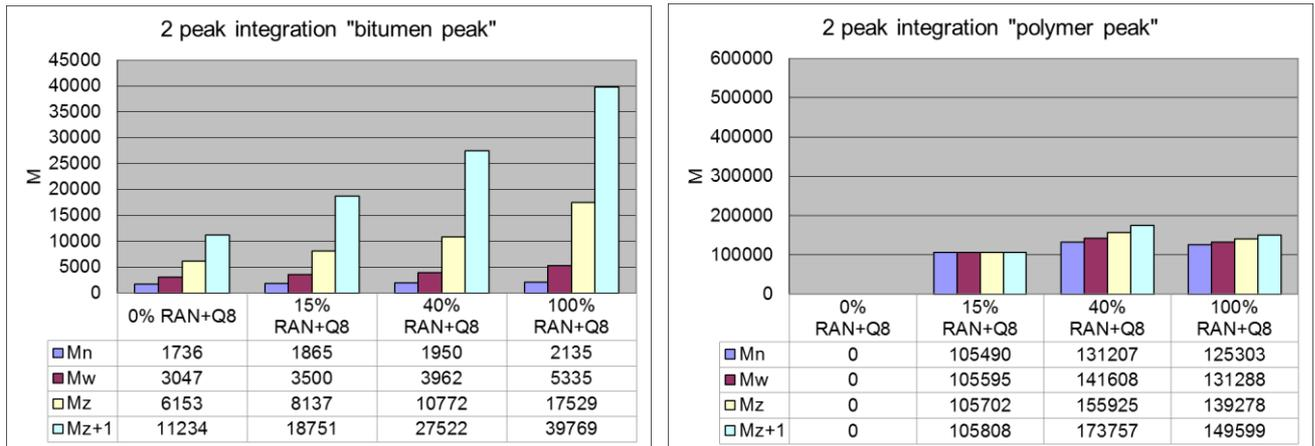
Figure 4.32 Molecular weights of RAN+Q8 for bitumen part (left) and polymer part (right)
