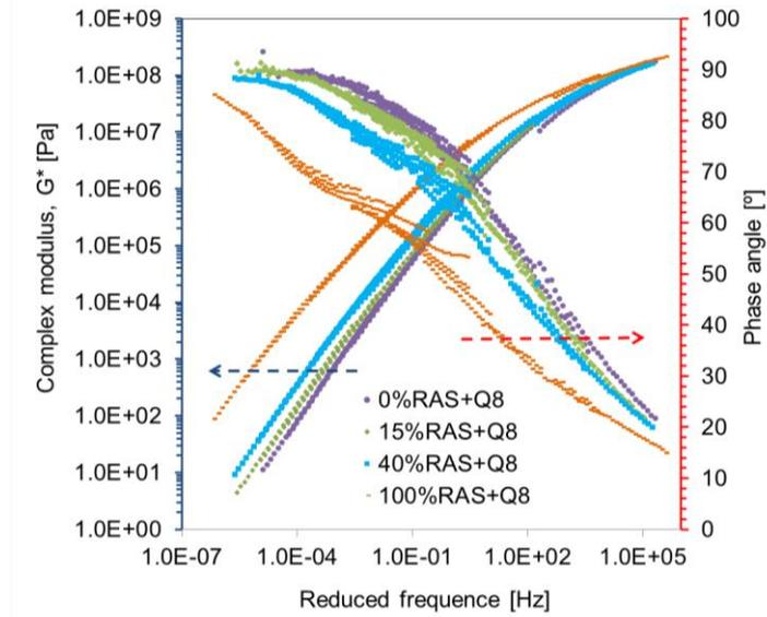
Figure 4.20 Master curves of the complex shear modulus and phase angle for binders in the RAS+Q8 group at a reference temperature of 25 °C
