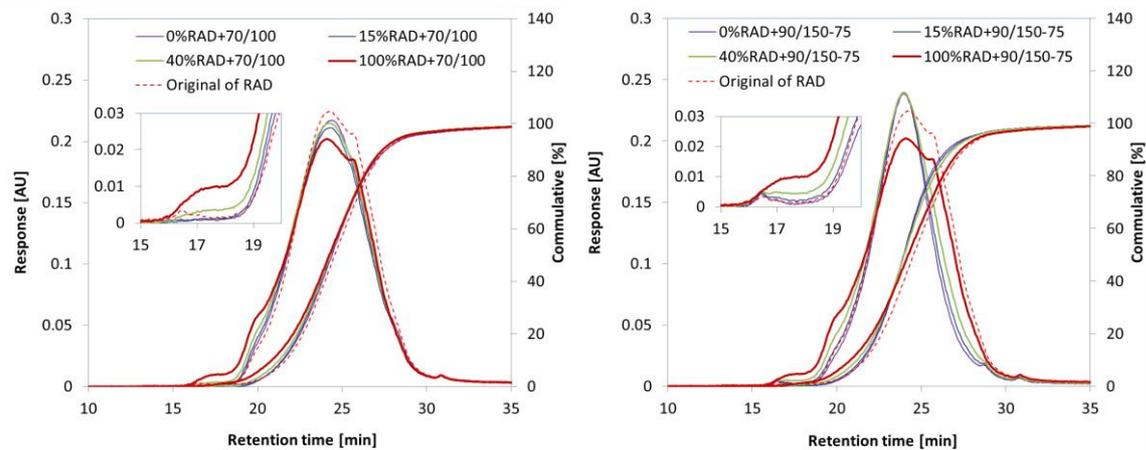
Figure 4.28 Molecular weight distribution of RAD+70/100 group (left) and RAD+90/150-75 group (right)
