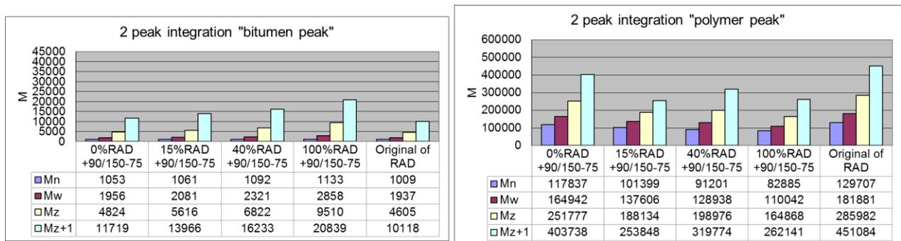
Figure 4.37 Molecular weights of RAD+90/150-75 for bitumen part (left) and polymer part (right)
