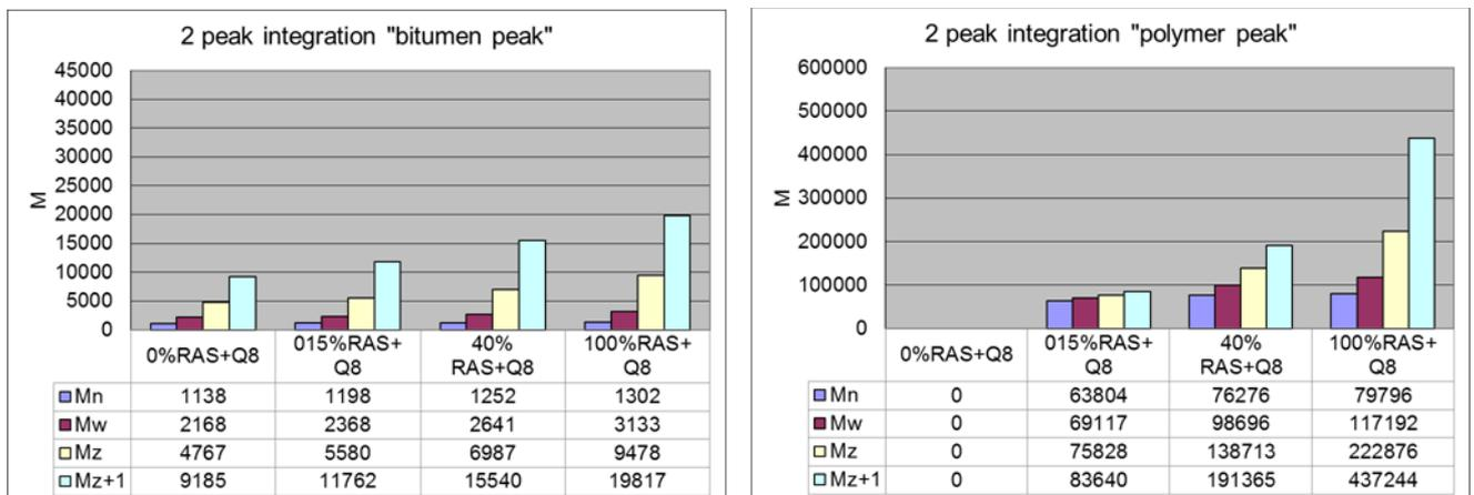
Figure 4.34 Molecular weights of RAS+Q8 for bitumen part (left) and polymer part (right)
