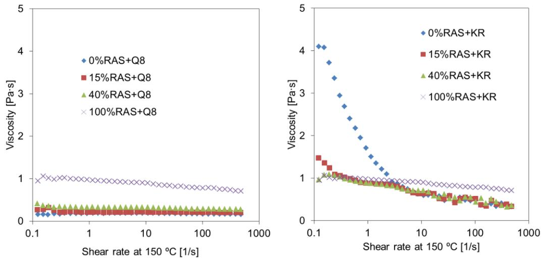
Figure 4.17 Viscosity at 150 °C as function of the shear rate measured with the cone/plate rheometer, for binder groups of RAS+Q8 (left) and RAS+KR (right)
