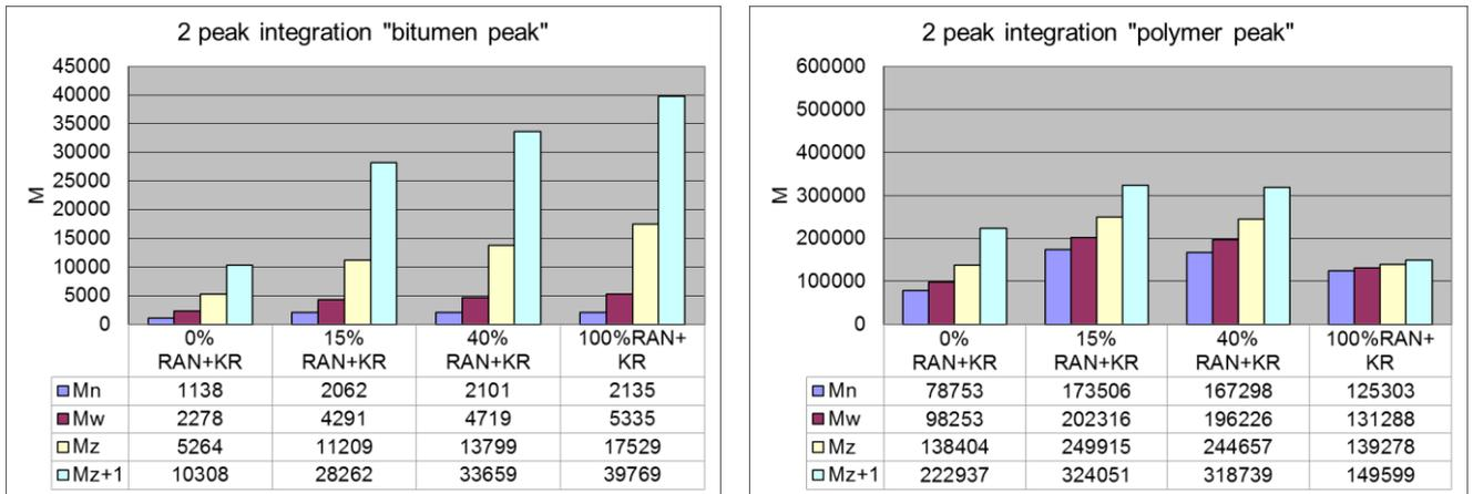
Figure 4.33 Molecular weights of RAN+KR for bitumen part (left) and polymer part (right)
