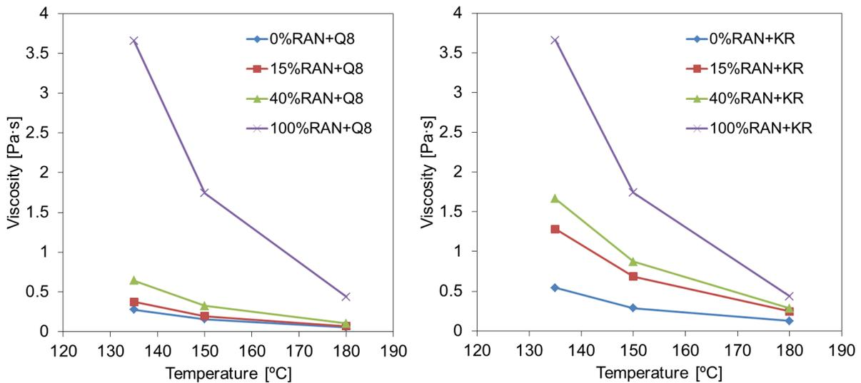
Figure 4.12 Viscosities at a shear rate 500/s and at three temperatures for binder groups of RAN+Q8 (left) and RAN+KR (right), measured with the cone/plate rheometer
