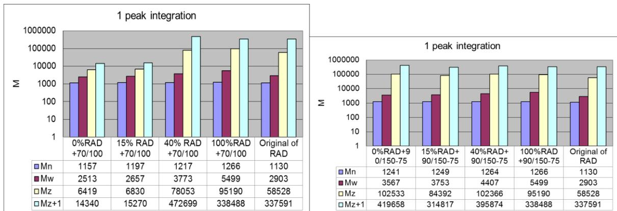
Figure 4.31 Molecular weights for RAD+70/100 group (left) and RAD+90/150-75 group (right)
