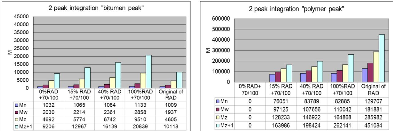
Figure 4.36 Molecular weights of RAD+70/100 for bitumen part (left) and polymer part (right)
