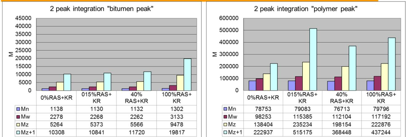
Figure 4.35 Molecular weights of RAS+KR for bitumen part (left) and polymer part (right)
