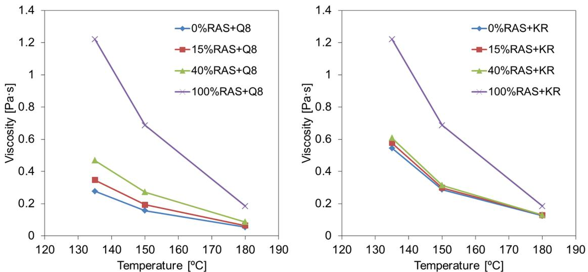
Figure 4.13 Viscosities at a shear rate 500/s and at three temperatures for binder groups of RAS+Q8 (left) and RAS+KR (right), measured with the cone/plate rheometer
