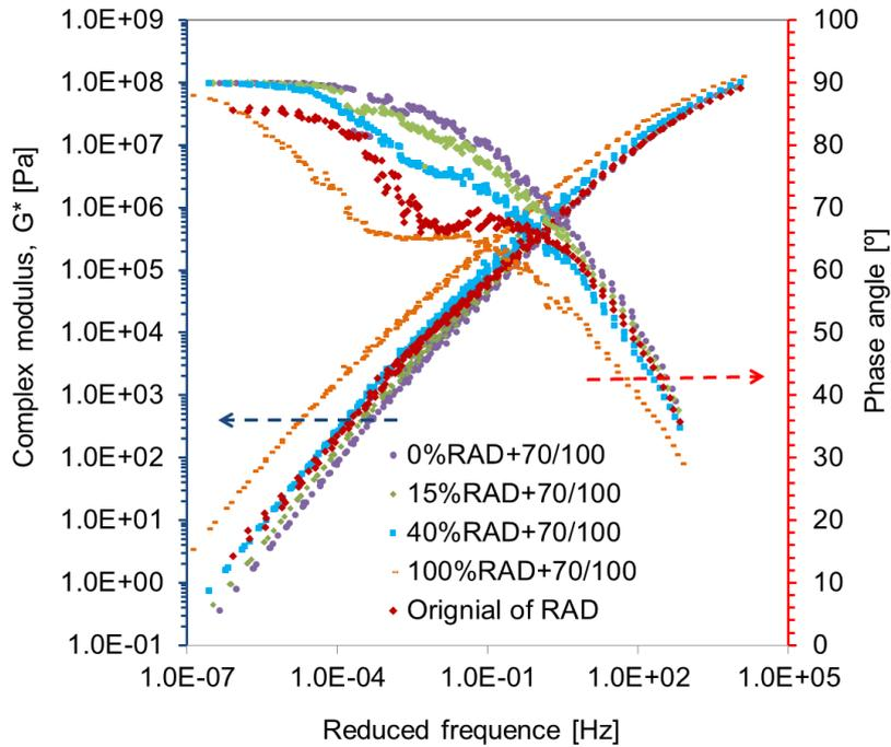
Figure 4.22 Master curves of complex modulus and phase angle for binders in the RAD+70/100 group at a reference temperature of 25 °C
