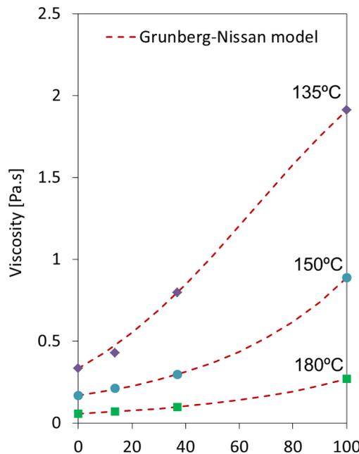
Figure 4.15 Relation between RA content and viscosity, an example for RAD+70/100 binder
