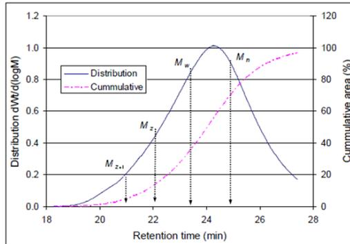
Figure 3.4 Example of the molecular weight distribution of bitumen
