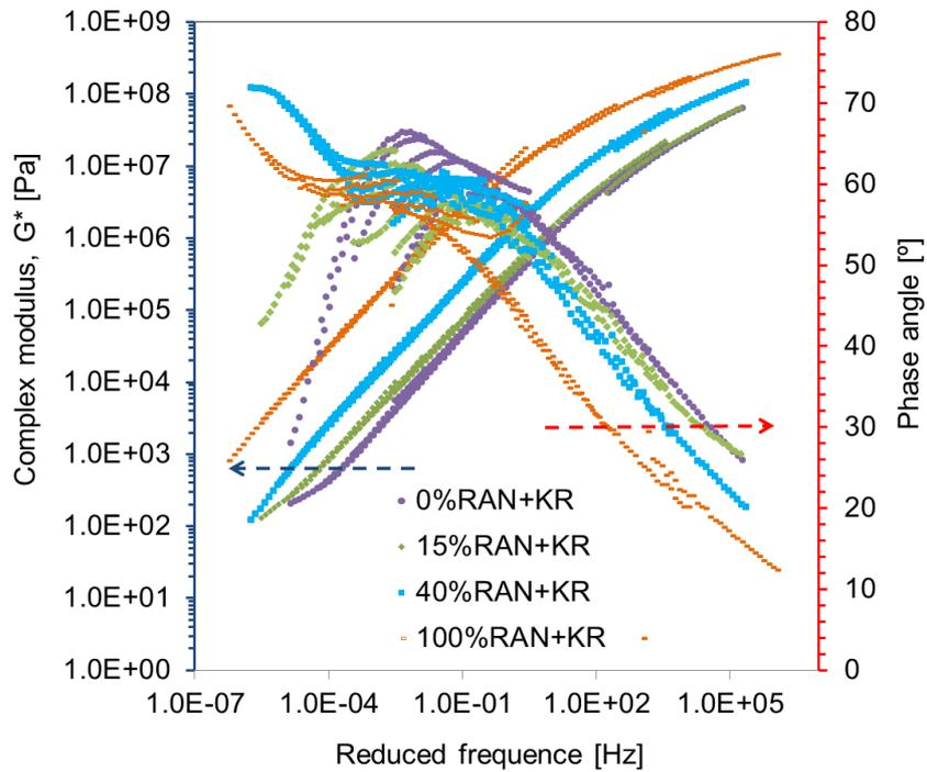
Figure 4.19 Master curves of the complex modulus and phase angle for binders in the RAN+KR group at a reference temperature of 25 °C
