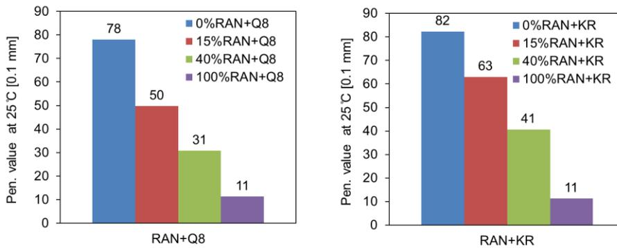
Figure 4.1 Penetration values at 25 °C for binder groups of RAN+Q8 (left) and RAN+KR (right)
