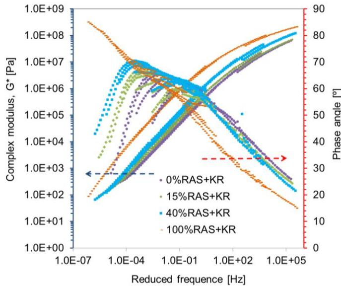
Figure 4.21 Master curves of complex modulus and phase angle for binders in the RAS+KR group at a reference temperature of 25 °C
