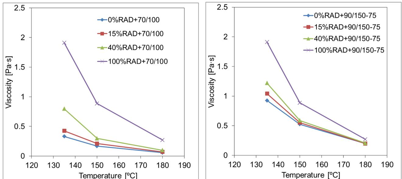
Figure 4.14 Viscosities at three temperatures for binder groups of RAD+70/100 (left) and RAD+90/150-75 (right), measured by using Brookfield rheometer
