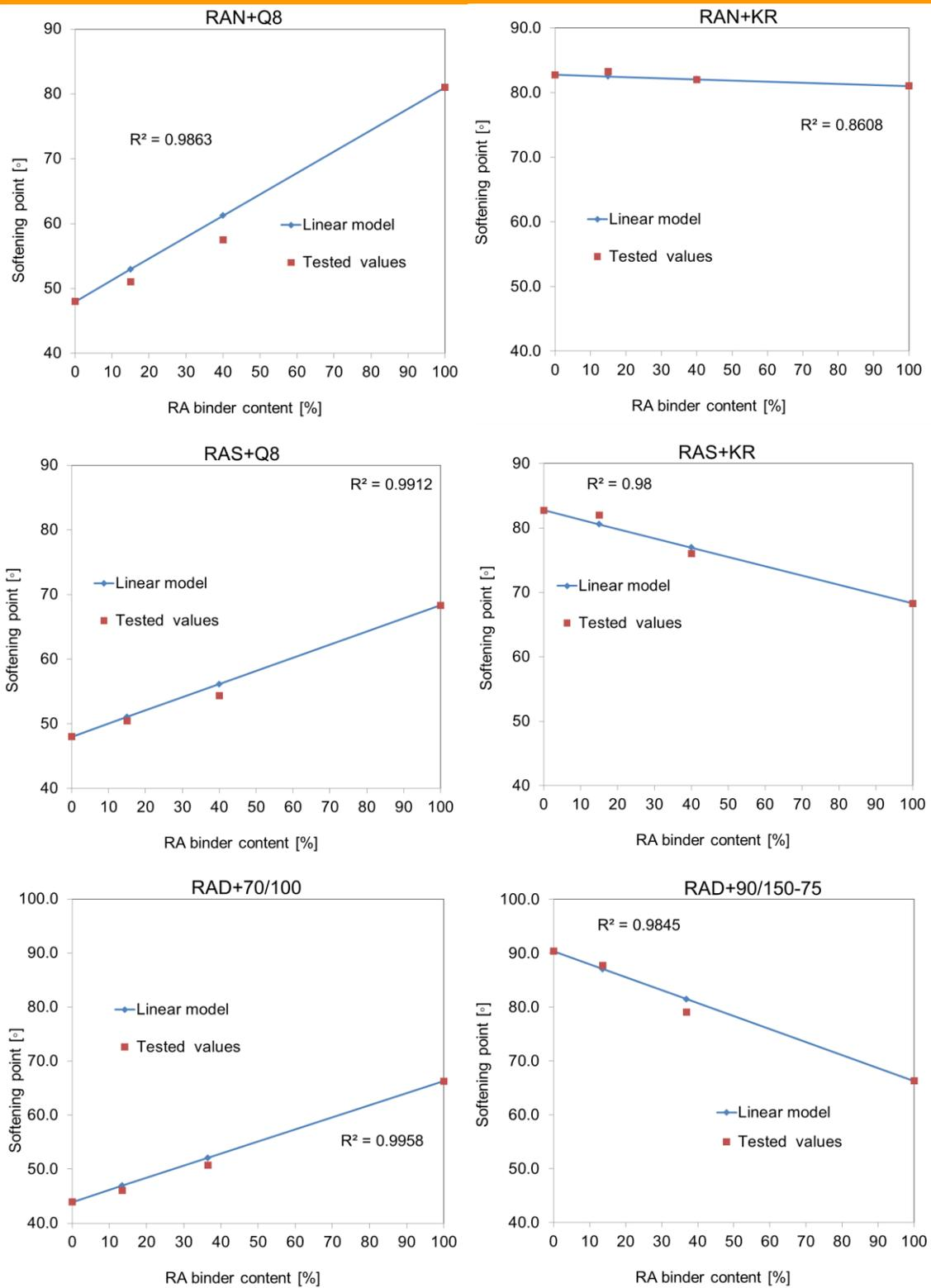
Figure 4.11 Relation between S.P. value and RA binder content for six binder groups
