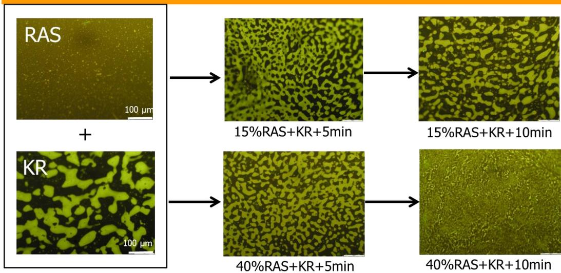
Figure 2.4 Fluorescent images of 15%RAS+KR and 40%RAS+KR before and after mixing for 5 and 10 mins
