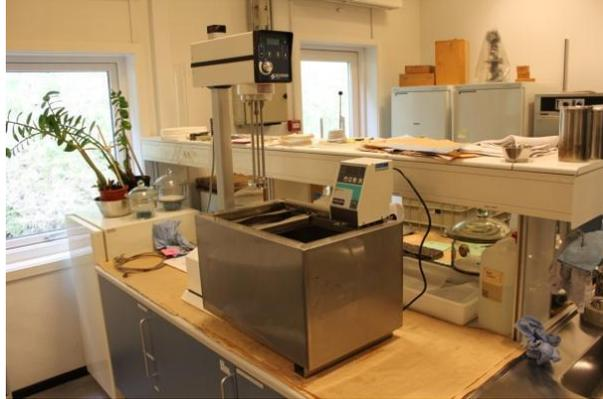
Figure 2.2 Vessel, thermostat and high shear mixer outside fuming cupboard (DRD)
