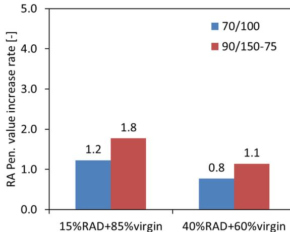
Figure 4.5 Influence of virgin binder 70/100 and 90/150-75 on the Pen. value of RAD at 15% RA content and 40% RA content
