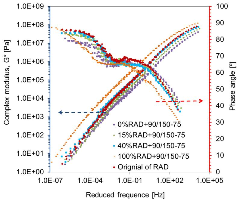
Figure 4.23 Master curves of complex modulus and phase angle for binders in the RAD+90/150-75 group
