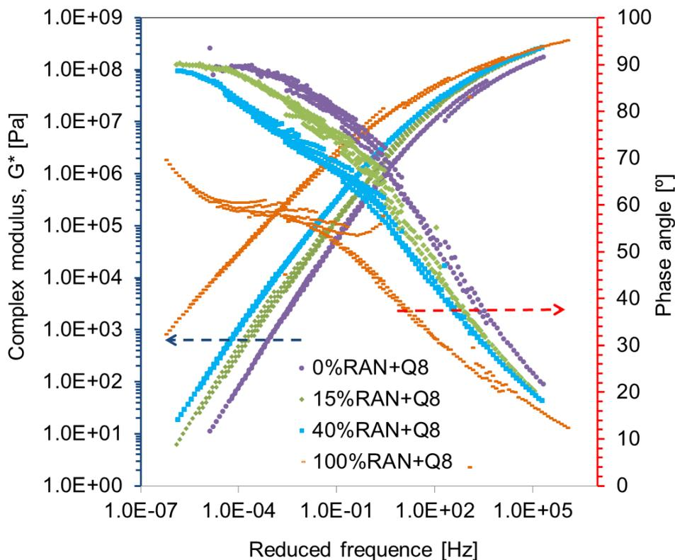
Figure 4.18 Master curves of the complex shear modulus and phase angle for binders in the RAN+Q8 group at a reference temperature of 25 °C
