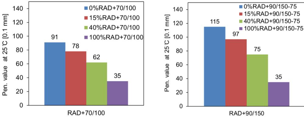
Figure 4.3 Penetration values at 25 °C for binder groups of RAD+70/100 (left) and RAD+90/150-75 (right)
