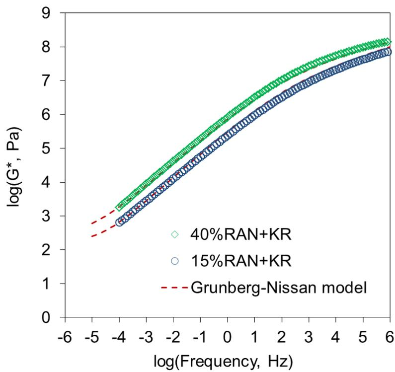
Figure 4.25 Master curves of 40%RAN+KR and 15%RAN+KR fitted by the Grunberg-Nissan model
