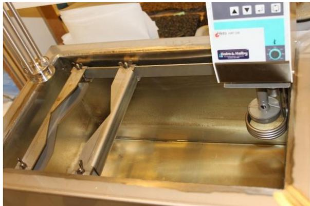
Figure 2.3 Close-up of the adjustable fixture for the blending container and the thermostat
