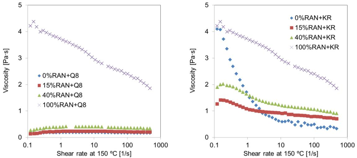
Figure 4.16 Viscosity at 150 °C as function of the shear rate measured with the cone/plate rheometer, for binder groups of RAN+Q8 (left) and RAN+KR (right)
