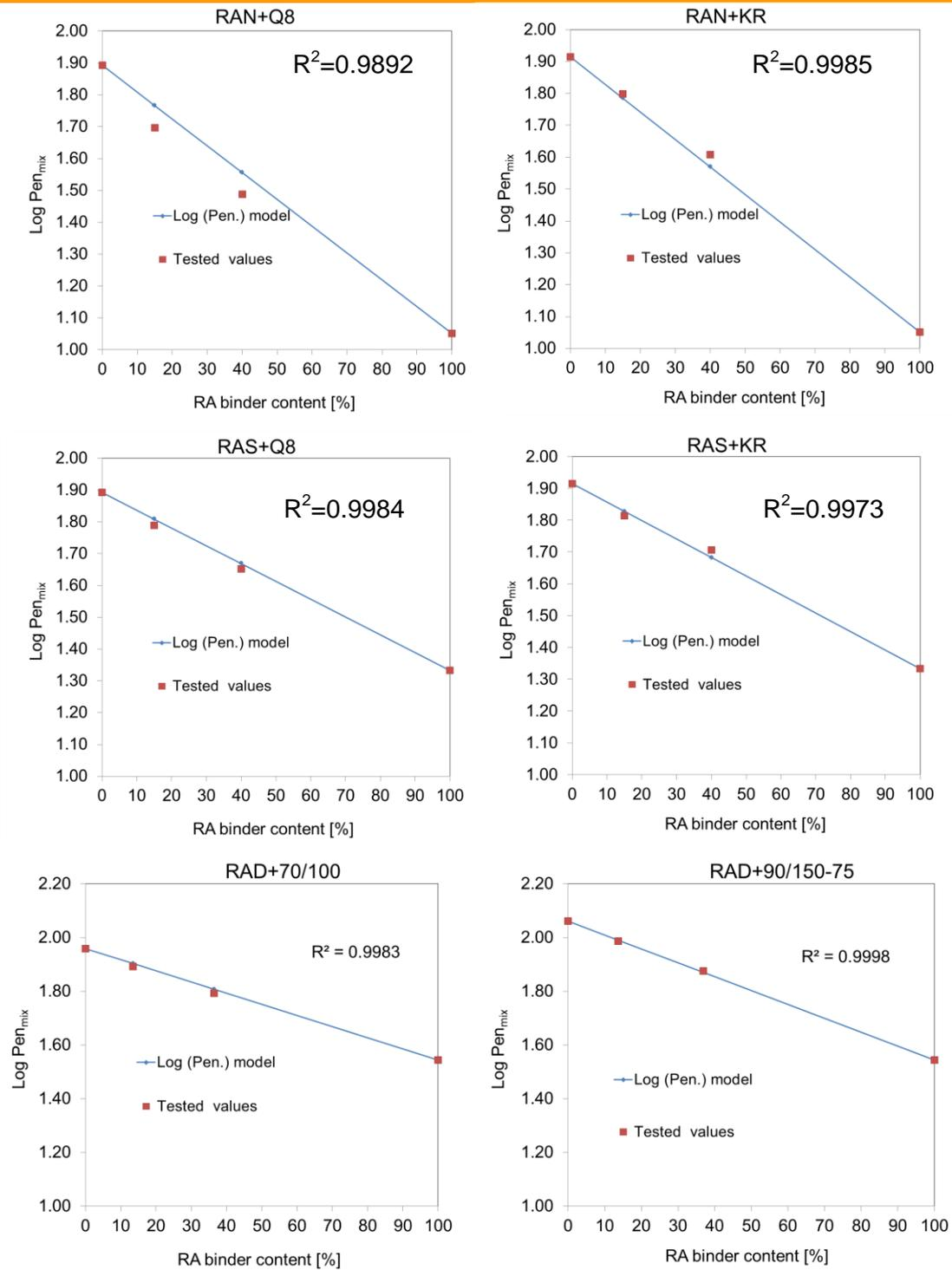
Figure 4.10 Relation between Pen. value at 25 °C and RA binder content for six binder groups
