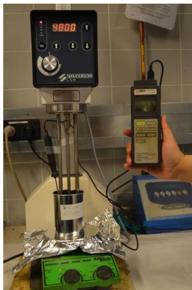
Figure 2.1 Silverson L5M high shear mixer at DUT
