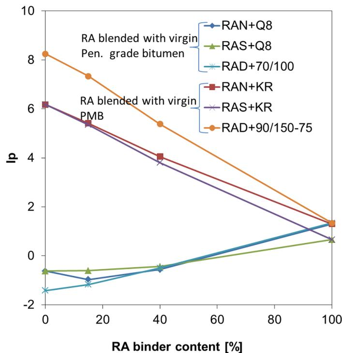
Figure 4.9 Penetration index ( $I_p$ ) of six binder groups as function of RA content and the virgin binder type
