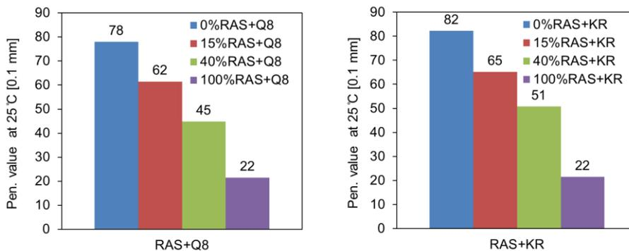
Figure 4.2 Penetration values at 25 °C for binder groups of RAS+Q8 (left) and RAS+KR (right) (same)
