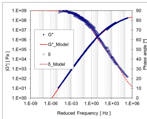
Figure 3.2 Master curves of Pen. grade bitumen Q8 and its MHS model
