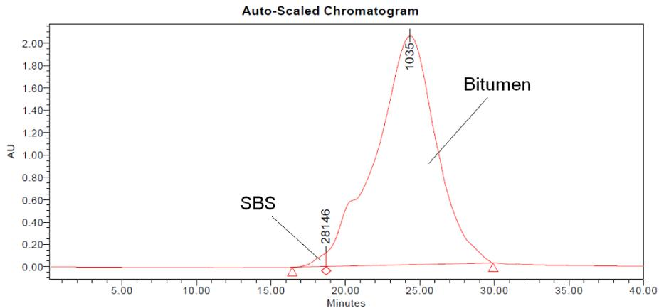
Figure 3.5 Overlap polymer and bitumen component
