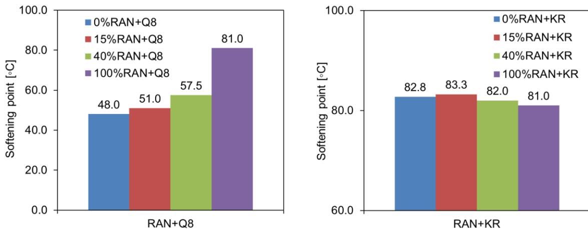
Figure 4.6 Softening point for binder groups of RAN+Q8 (left) and RAN+KR (right)
