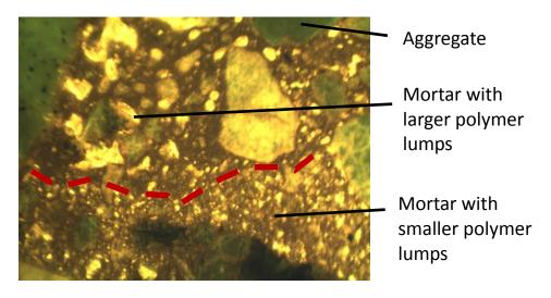
Figure 3: Details from micrograph of AC 11 with PMB and 40 % RA (Figure represents 0.80 x 1.06 mm)
