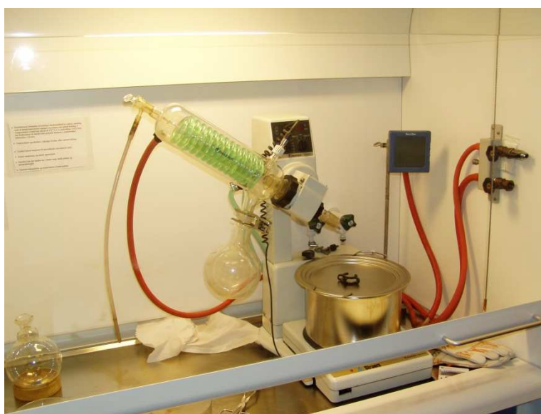
Figure 1 Rotary evaporator for recovery of binder according to EN 12697-3
