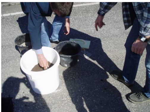
Aggregate 0/5 mm is transferred to a mixing container
