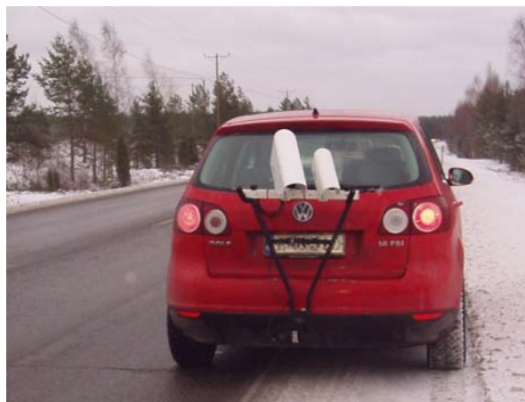
Figure 13 The first installation in 2006 using optical remote sensors Vaisala DSC111 and DST111 behind the observing vehicle. [21]
