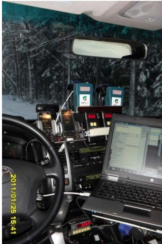
Figure 8 Instrumentation inside the monitoring vehicle with Eltrip, Gripman and smartphones with accelerometers using \mu TEC software. [15]
