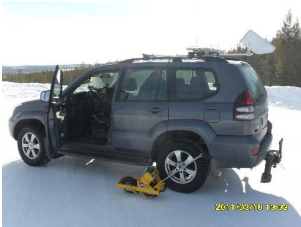
Figure 7 Monitoring vehicle used in the friction monitor comparison study. T 2 GO installed on the back wheel, optical DSC111 on the roof and RCM411 at the back. [15]
