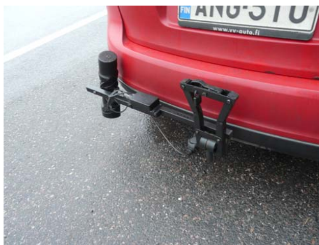
Figure 10 Optical remote sensor RWS411 for detection of road conditions. [17]
