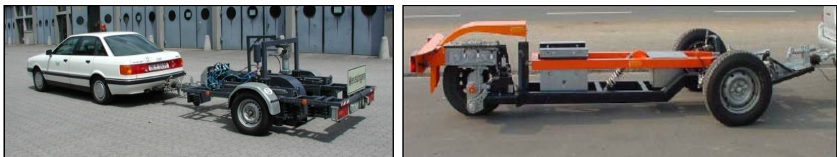
Figure 7: Different rolling resistance trailers for passenger car tyres [28]
