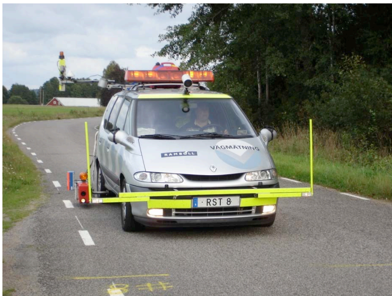
Figure 4 Ecodyn 30 measuring a broken edge line.
