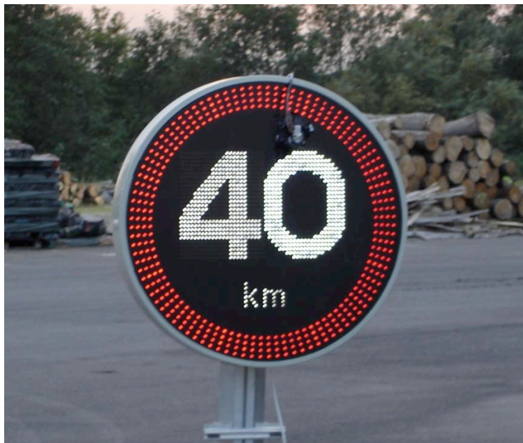
Figure 3 A Danish VMS showing the speed limit.
