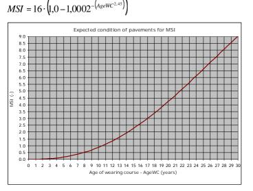
Figure 5: Expected condition of pavement, expressed with MSI
