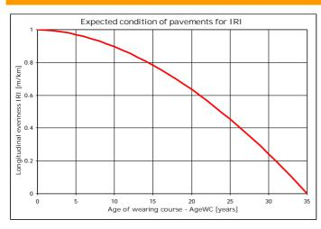
Figure 10 Normalized expected condition of pavement, expressed with IRI
