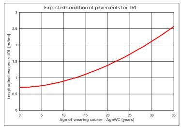
Figure 9 Expected condition of pavement, expressed with IRI
