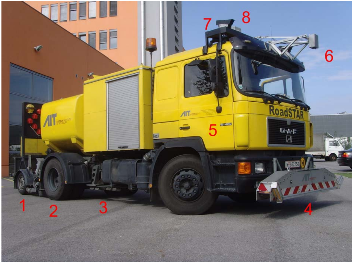
Figure 1: RoadSTAR measurement units [AIT Picture]
