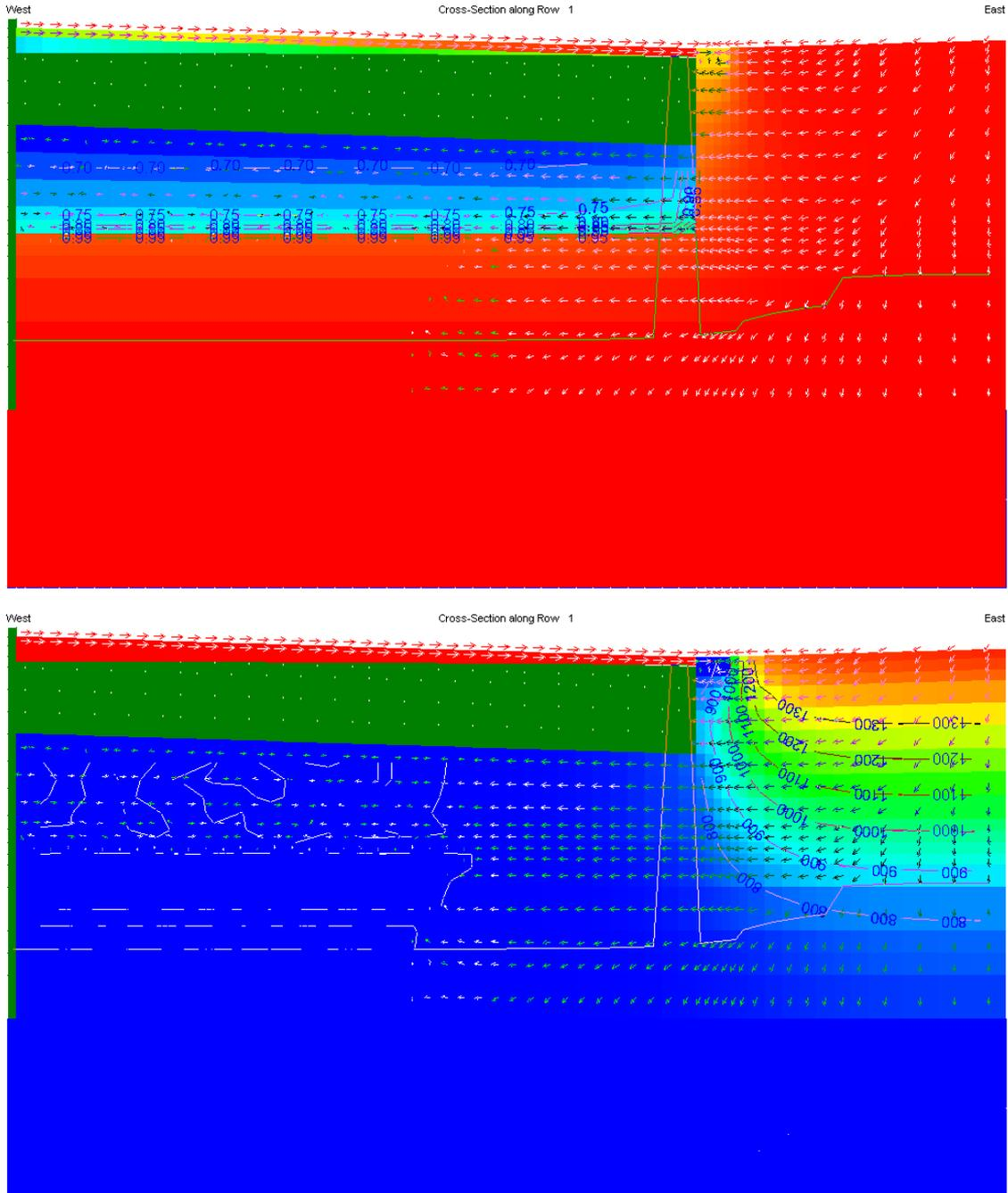
Figure 23: saturation level and head after dry period, rainfall pattern 2.
