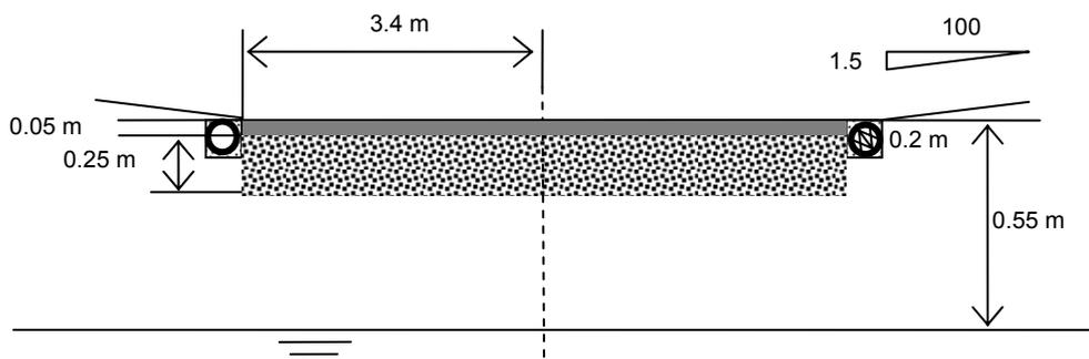
Figure 3: schematic of the secondary Nordic road simulated.
