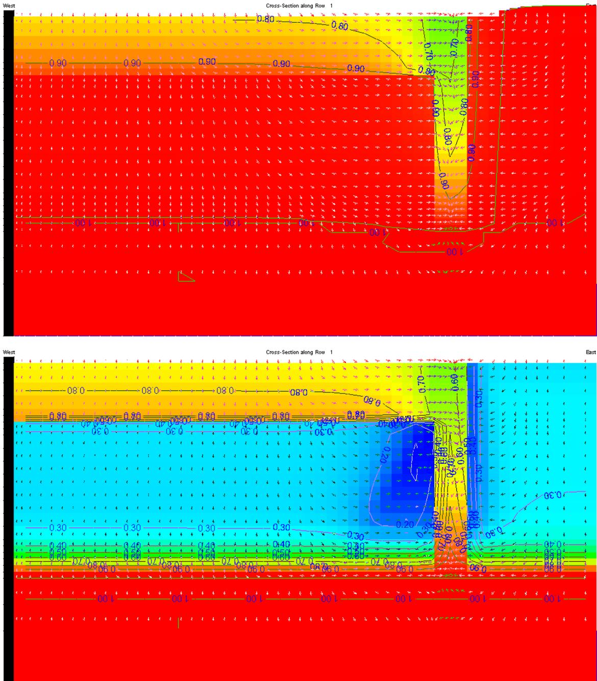
Figure 43: comparison between the saturation levels of a subbase surrounded by clay and by sand (rainfall pattern 1, after rain).
