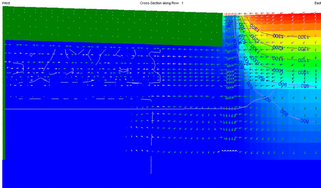
Figure 18: saturation level and head after dry period, rainfall pattern 3.
