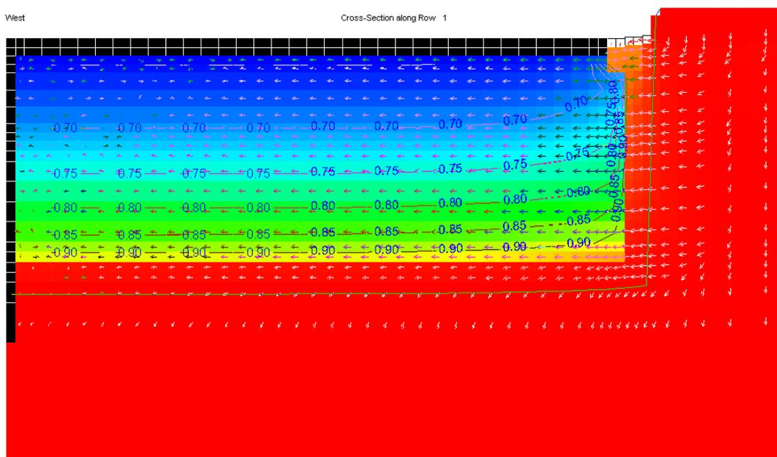
Figure 39: saturation level after a dry period (rainfall pattern n. 3).
