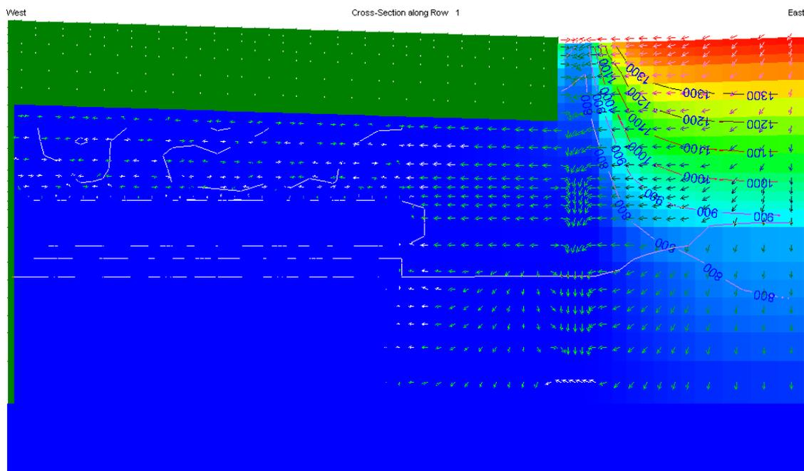
Figure 10: saturation level and head after dry period, rainfall pattern 2.
