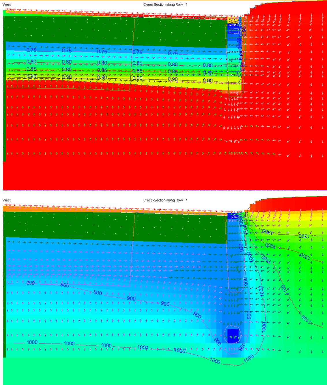
Figure 29: saturation level and head after rain (case 3), drainage layer between subbase and subgrade.
