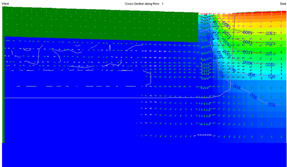
Figure 9: saturation level and head after rainfall, rainfall pattern 2.
