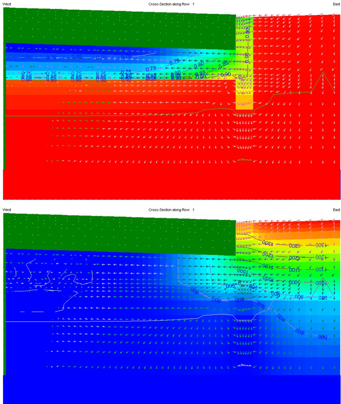
Figure 12: saturation level and heads, after dry weather, of a road where the draining materials has mixed with finer soil.
