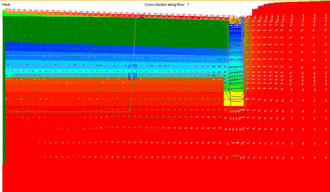
Figure 25: saturation level after rain for case 3, with a subsurface drainage system added.
