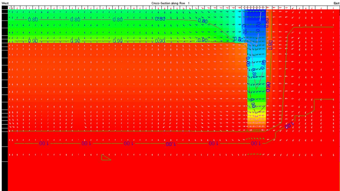
Figure 47: saturation level after rainfall and after dry period (moderate/heavy rain within short periods of time).
