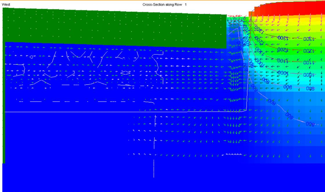
Figure 17: saturation level and head after rain, rainfall pattern 3.
