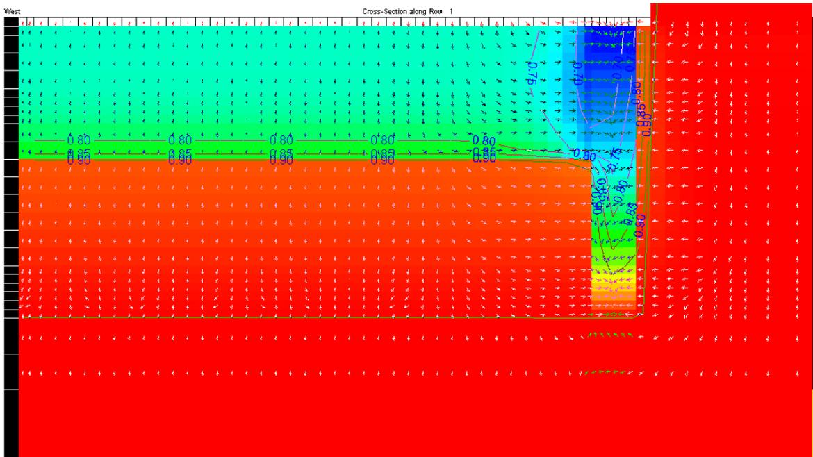
Figure 50: saturation level after rainfall (moderate/heavy rain within short periods of time), thicker subbase.
