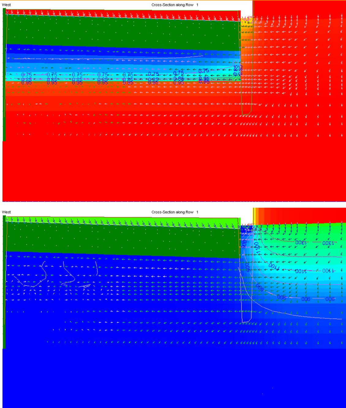
Figure 33: saturation level and head after rain, rainfall pattern 4.
