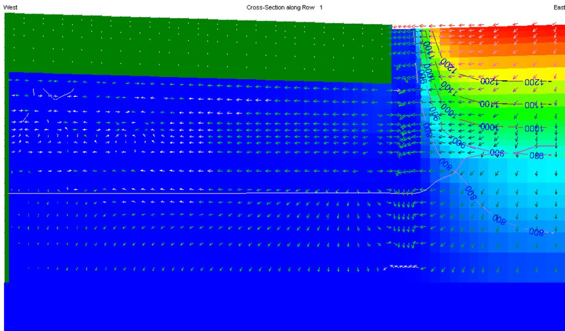
Figure 14: saturation level and head after dry period, rainfall pattern 4.
