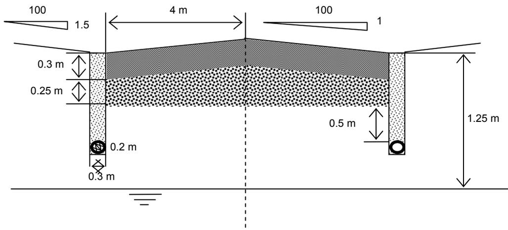
Figure 1: schematic of the high-volume traffic road simulated.
