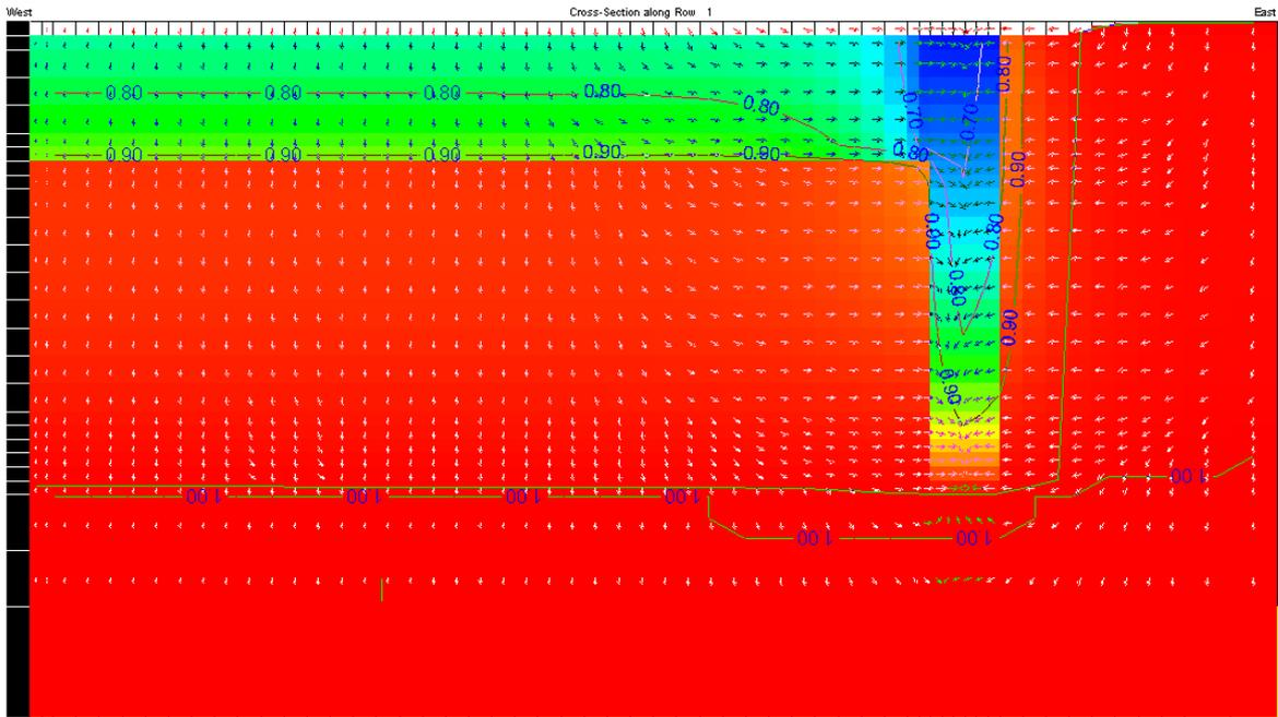
Figure 44: saturation level after a 6 hour light rain period (case 2).
