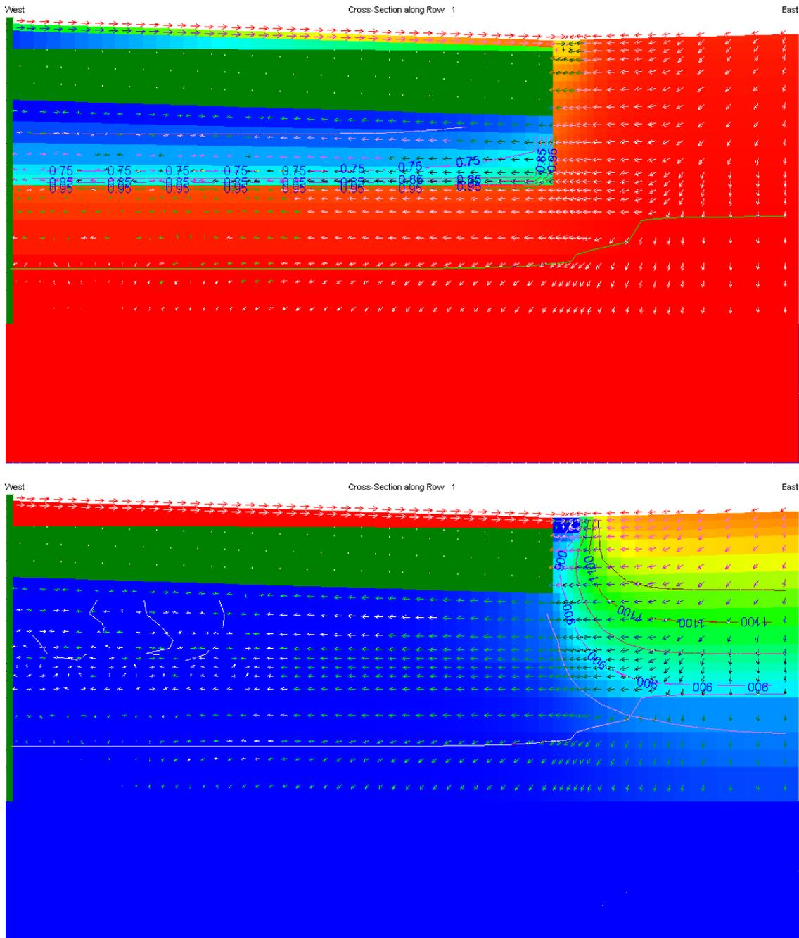
Figure 34: saturation level and head after a dry period, rainfall pattern 4.
