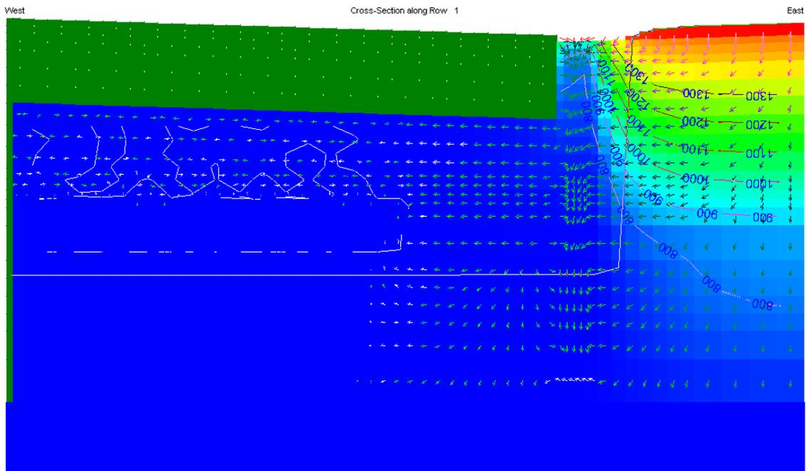
Figure 7: saturation level and head after rainfall, rainfall pattern 1.
