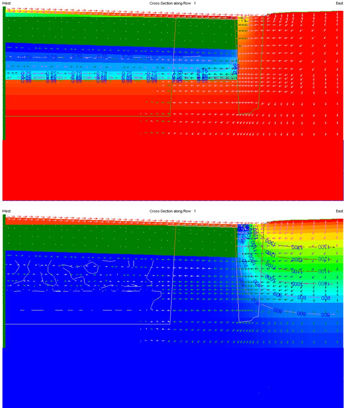
Figure 22: saturation level and head after rain, rainfall pattern 2.
