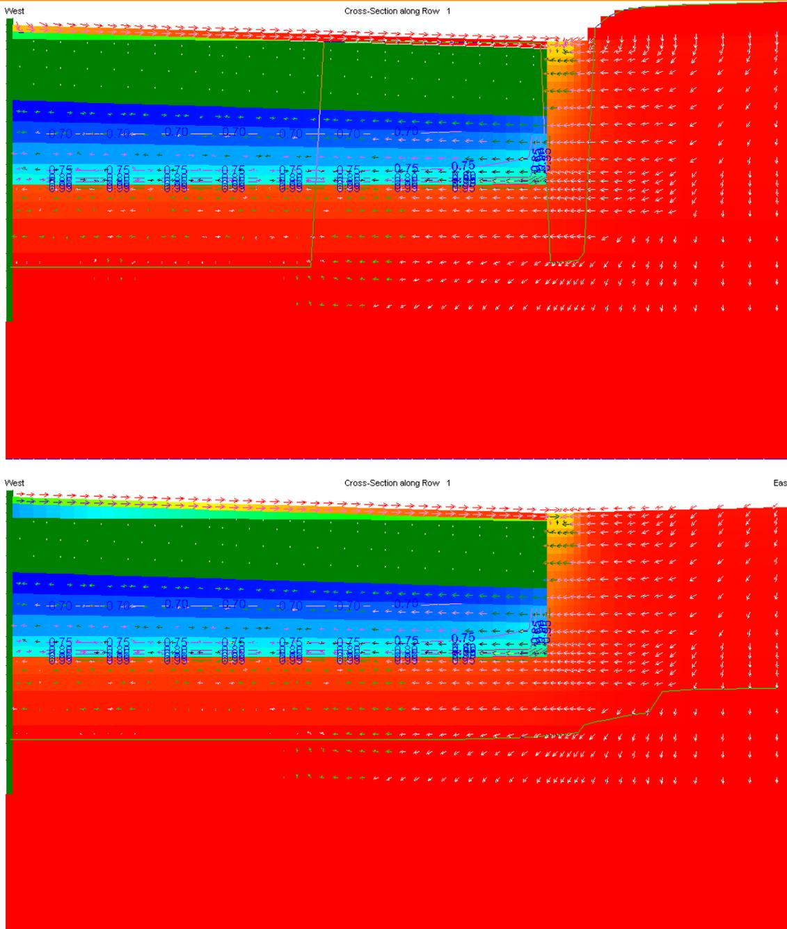
Figure 24: saturation level and head after rainfall and after dry period, rainfall pattern 3.
