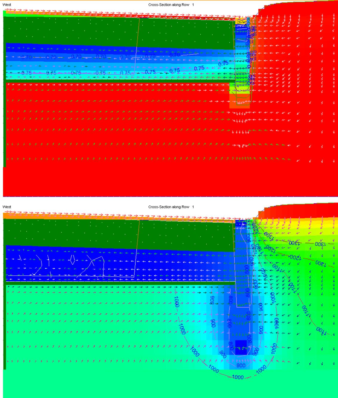
Figure 31: saturation level after a rainfall in presence of a high watertable and of an impermeable geotextile between subbase and subgrade (case 3).
