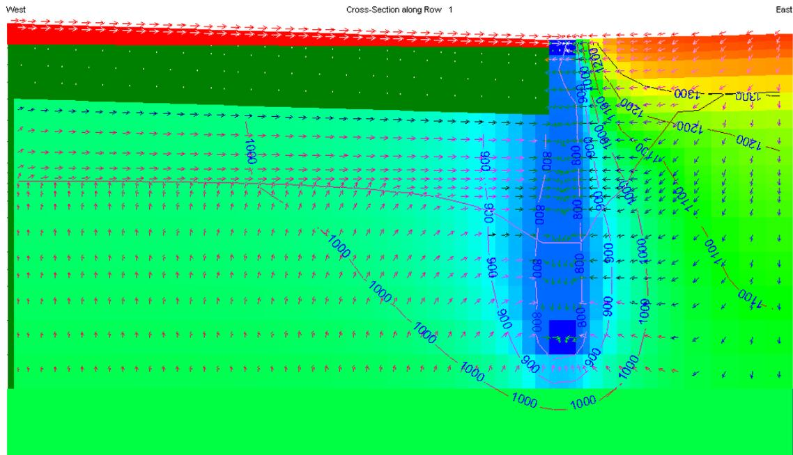
Figure 27: saturation level after a dry period in presence of a high watertable (case 3).
