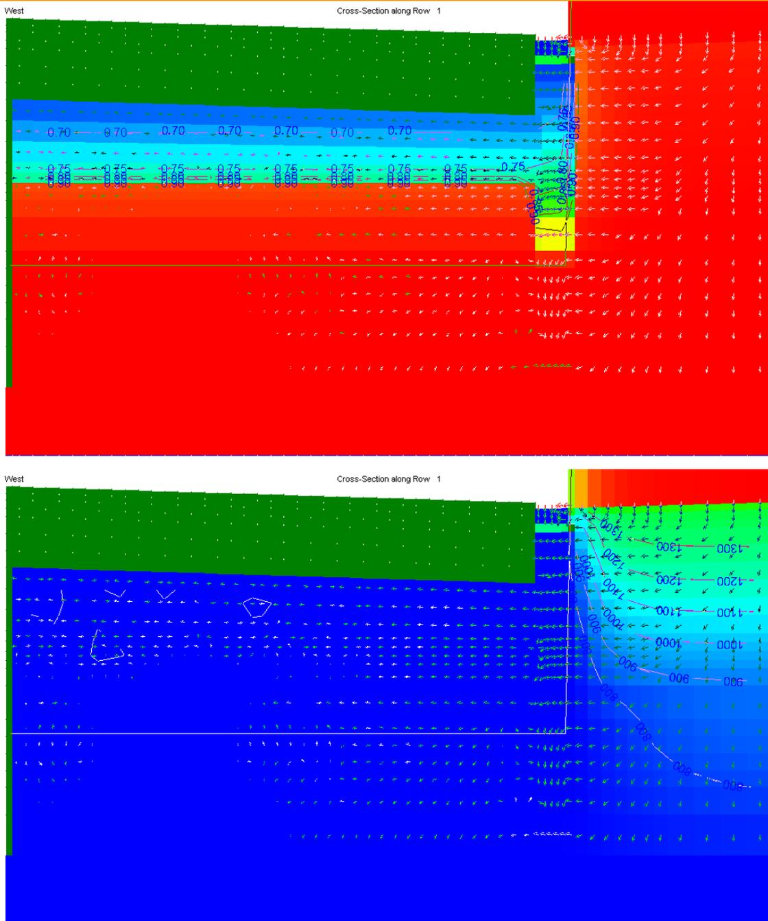
Figure 15: saturation level and head after rain, rainfall pattern 4, where a surface drain is added.
