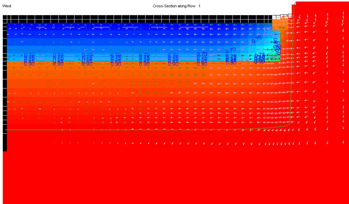
Figure 37: saturation level after 1 hour of heavy rainfall (case 3, but considering shorter “not-rain” intervals).
