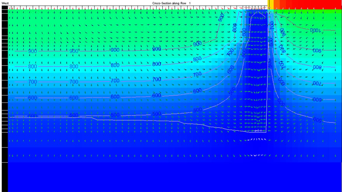
Figure 45: saturation level and head after rain, rainfall pattern 4.
