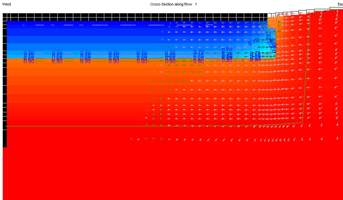
Figure 36: saturation level after a rainfall of high intensity but short duration (case 1) and after a rain of low intensity and long duration (case 2).
