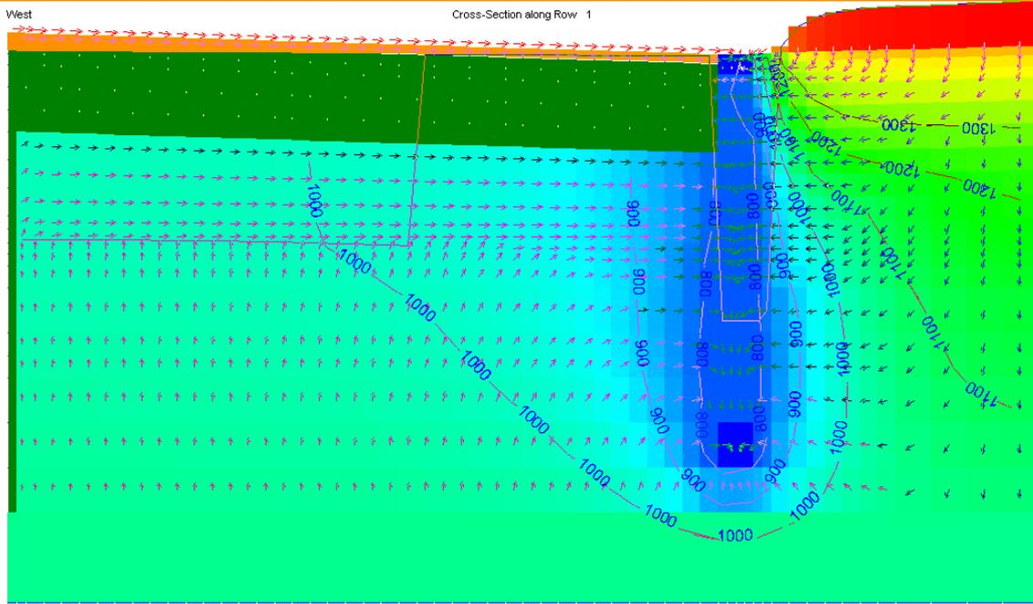
Figure 26: saturation level after rainfall in presence of a high watertable (case 3).
