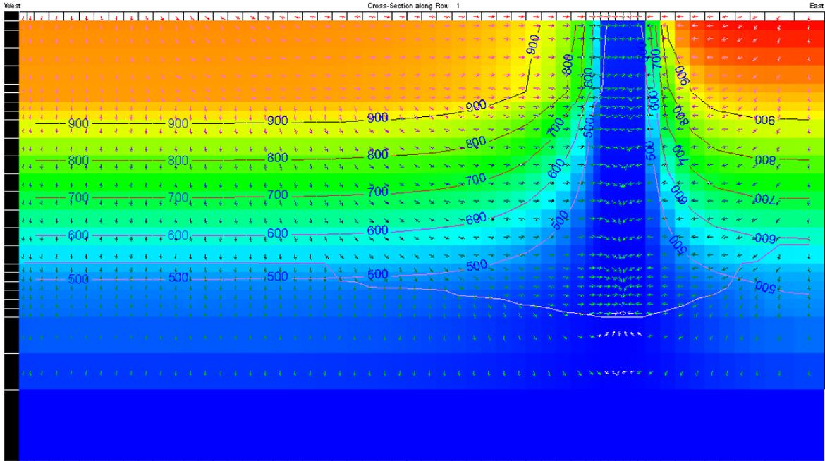
Figure 46: saturation level and head after a dry period, rainfall pattern 4.
