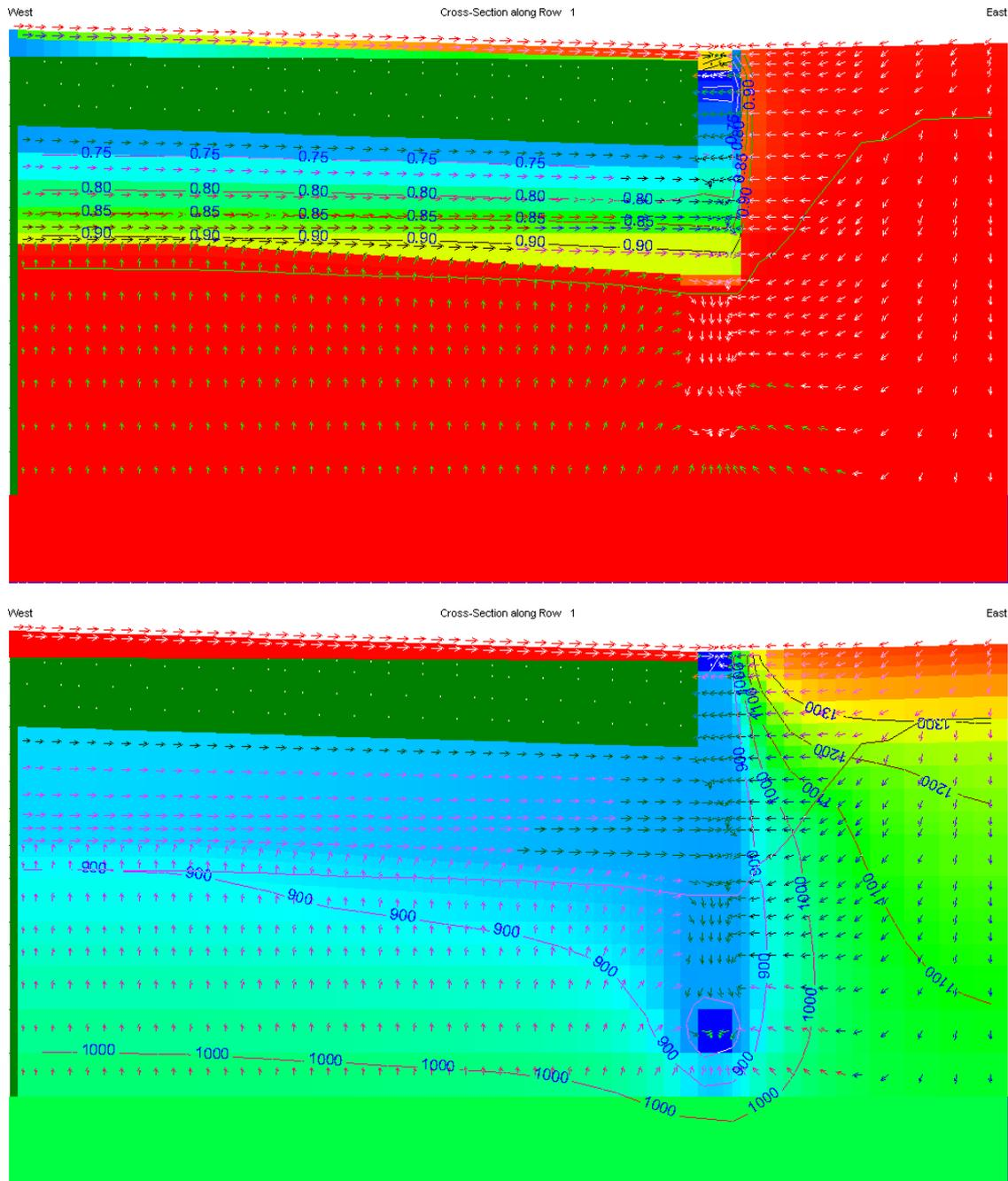
Figure 30: saturation level and head after dry period (case 3), drainage layer between subbase and subgrade.
