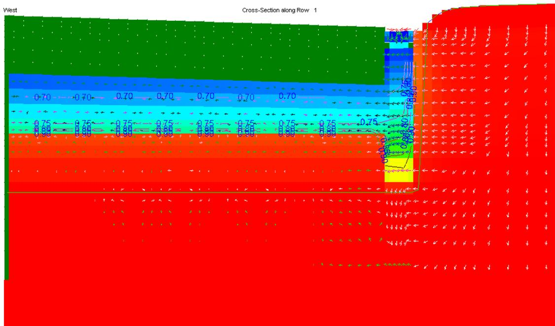
Figure 19: saturation level after rain, rainfall pattern 3, where a surface drain is added.
