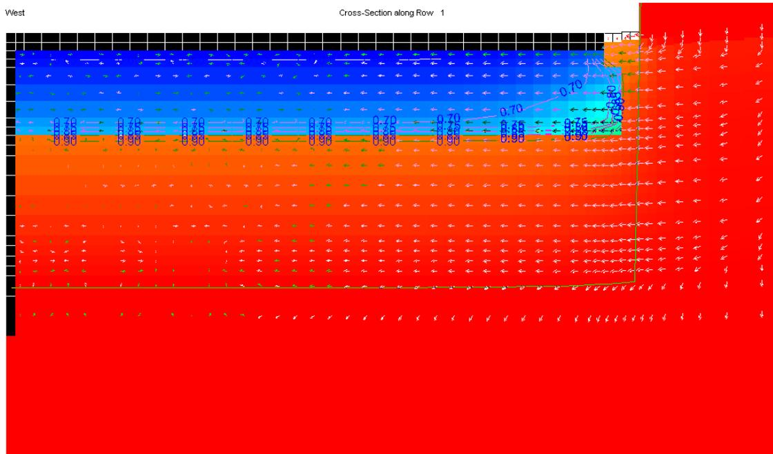
Figure 38: saturation level after 1 hour of very heavy rainfall (case 4).
