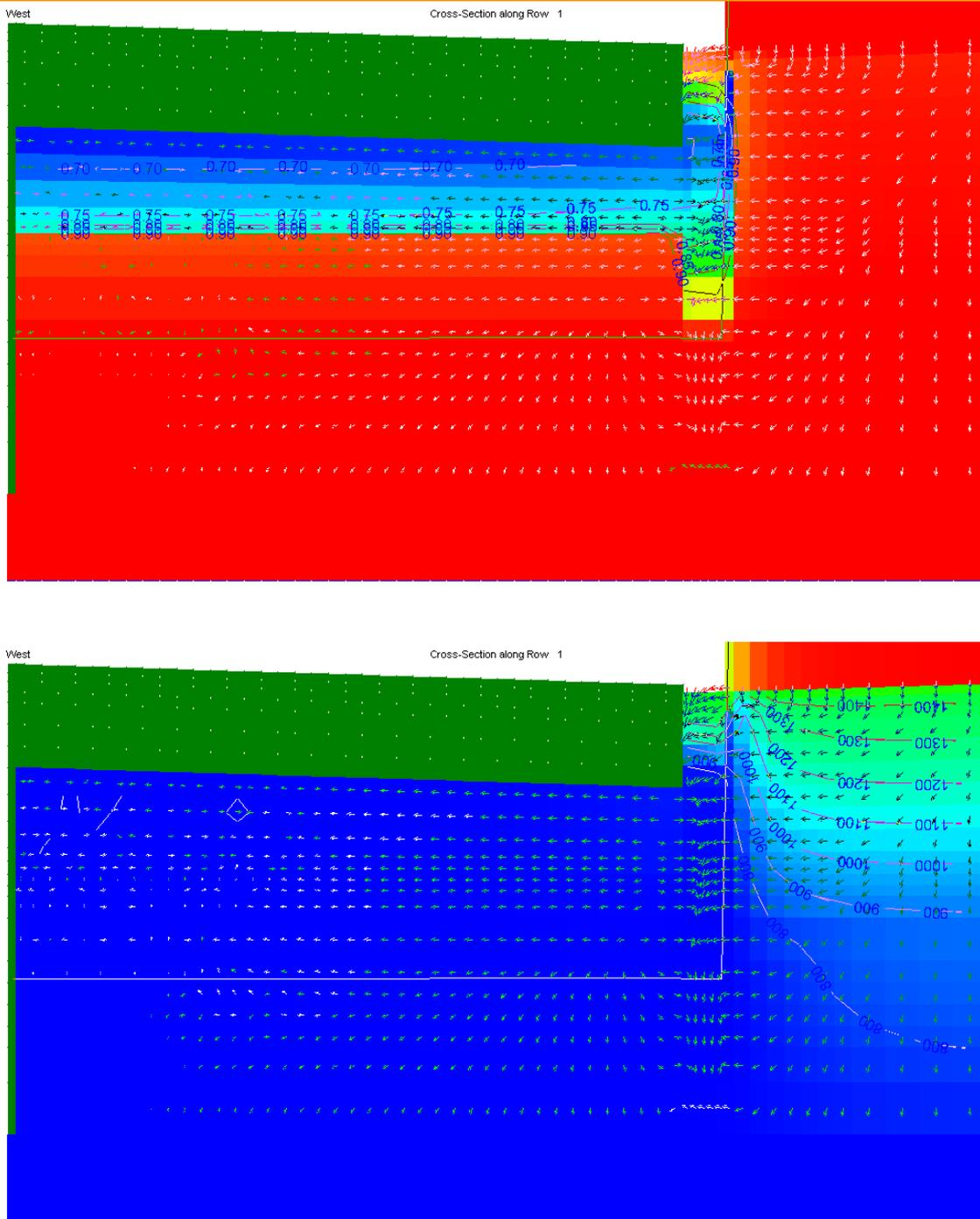
Figure 13: saturation level and head after rain, rainfall pattern 4.
