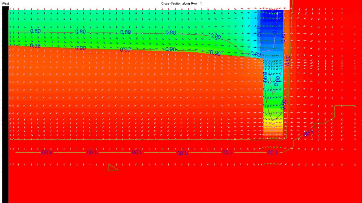
Figure 49: saturation level after rainfall (moderate/heavy rain within short periods of time), inclined subbase bed.
