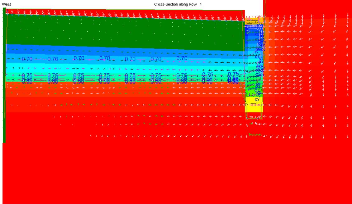
Figure 35: saturation level after rain, rainfall pattern 4, in presence of a subsurface drainage system and a larger surface drain.
