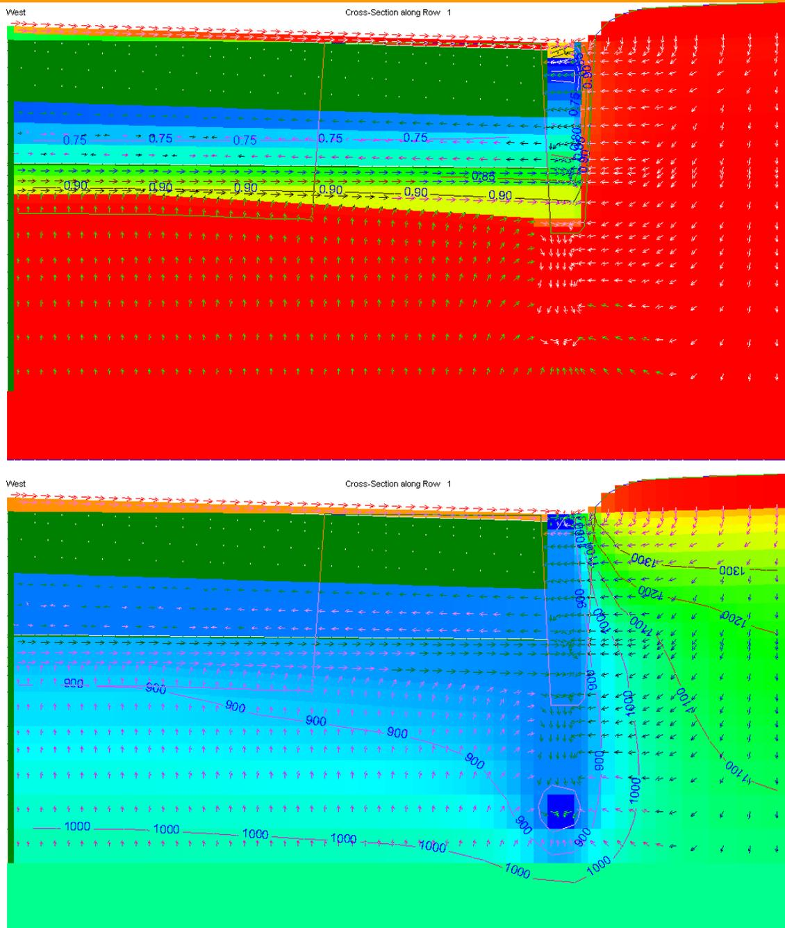
Figure 32: saturation level and head in the case of a high water table, considering a structure with both a geotextile to stop water from infiltrating into the subbase and a draining layer between the subbase and the clay to avoid water pressures accumulation.
