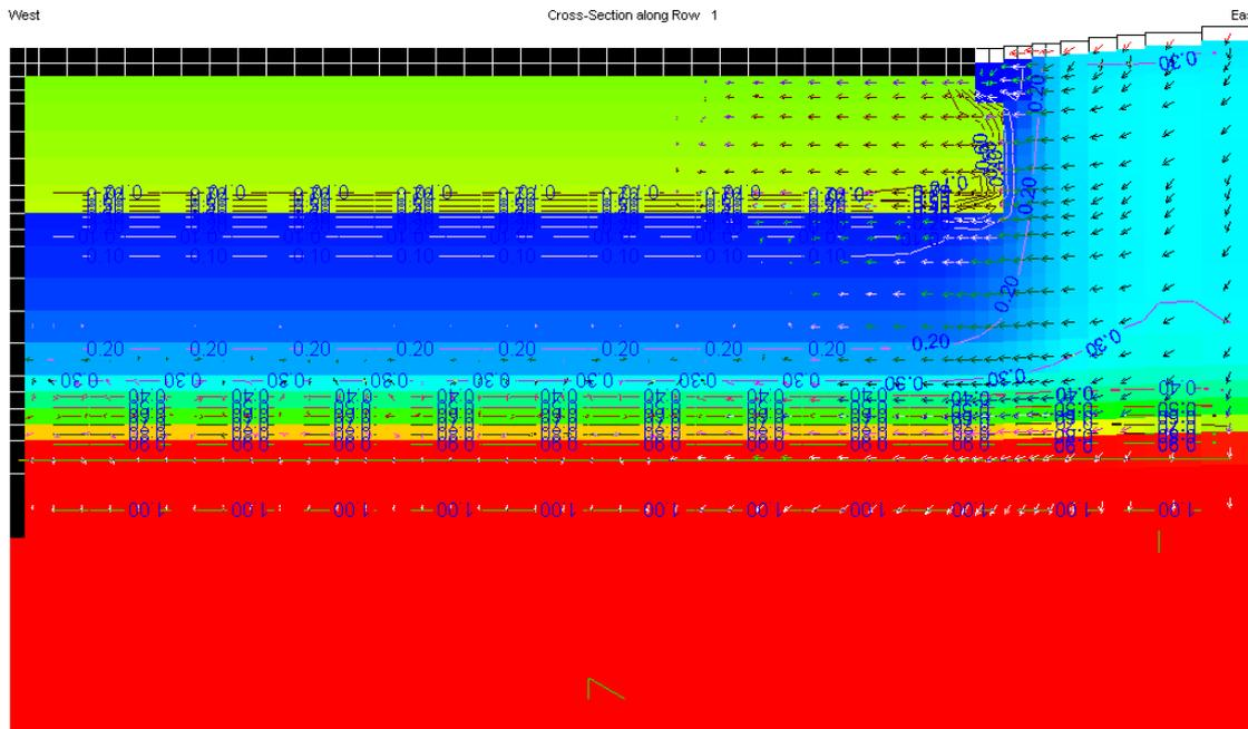
Figure 42: saturation level after rainfall (case 1), sandy soil.
