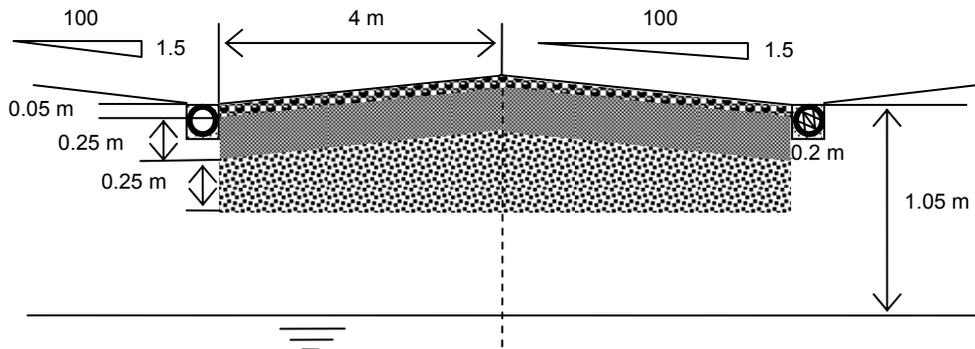
Figure 2: schematic of the porous road simulated.
