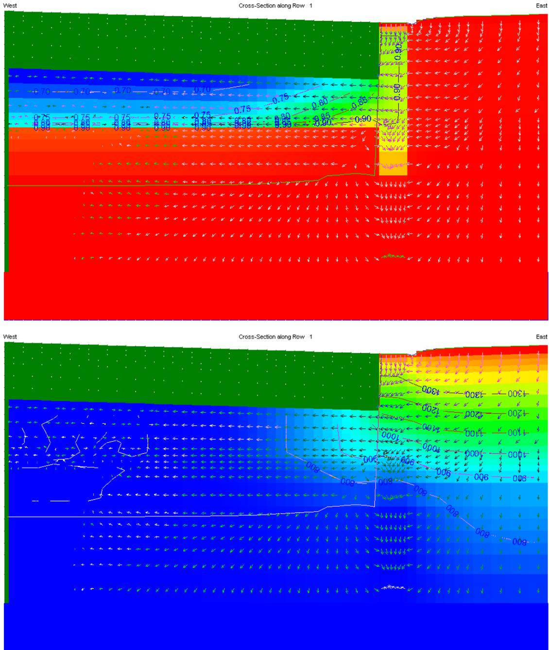
Figure 11: saturation level and heads, after rainfall, of a road where the draining materials has mixed with finer soil.
