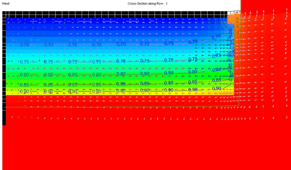
Figure 40: saturation level after rain (rainfall pattern n. 3).
