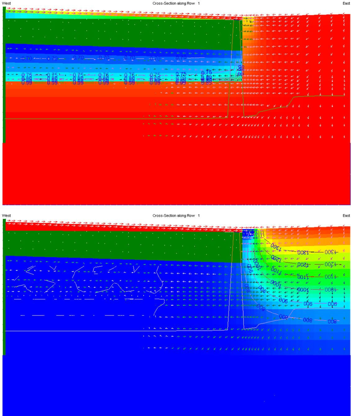
Figure 21: saturation level and head after dry period, rainfall pattern 1.
