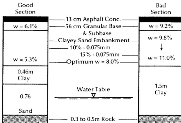
Fig. 8: Pavement distress related to soil suction: on the left, a cross section of the pavement with “good” subgrade, on the right the “bad” one (Birgisson & Ruth, 2003).
