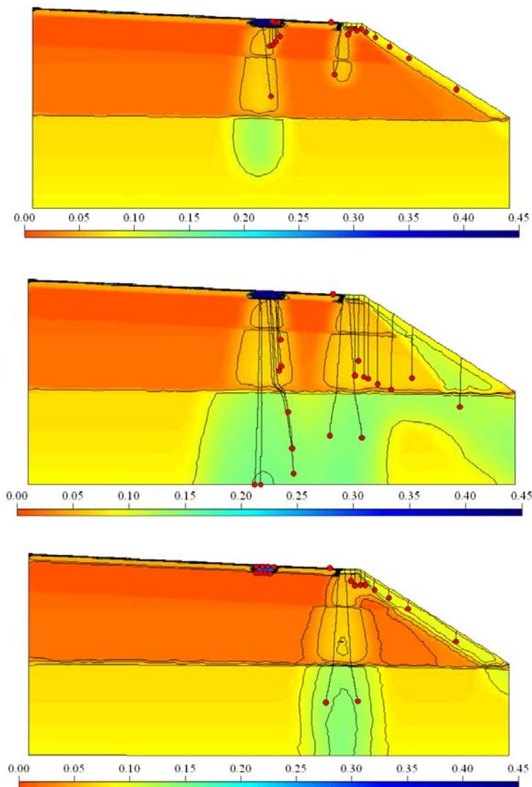
Fig. 14: The simulated volumetric water content after a light rainfall event (top), after a heavy rainfall event (middle) and after a moderate rainfall event using low fracture-zone permeability (bottom). The red dots indicate the flow paths of the infiltrated rainwater. The vertical scale is exaggerated for clarity (Hansson et al., 2005).
