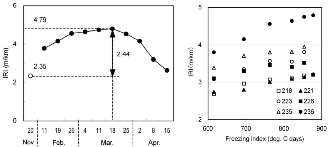
Fig. 10: Increase of IRI during the winter period (left) and its linear relationship with the freezing index (Kameyama, 2002).
