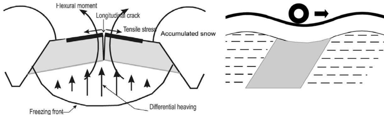
Fig. 17: Transverse and longitudinal differential heaving mechanism (Doré et al., 2002).
