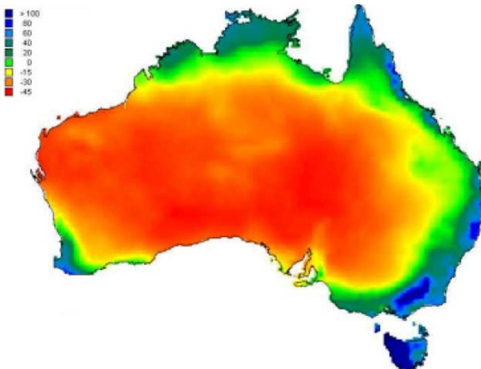
Fig. 11: Thornthwaite Moisture Index map of Australia referred to 2000 (Austroads, 2004). TMI > 100 = hyper-humid environment, 20 to 100 = humid, -20 to 20 = sub-humid, -40 to -20 = semiarid, -60 to -40 = arid environment.
