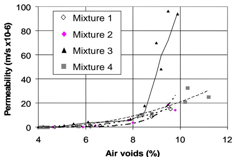
Fig. 2: Laboratory determination of the relationship between the asphalt air voids and permeability (Vivar & Haddock, 2007).
