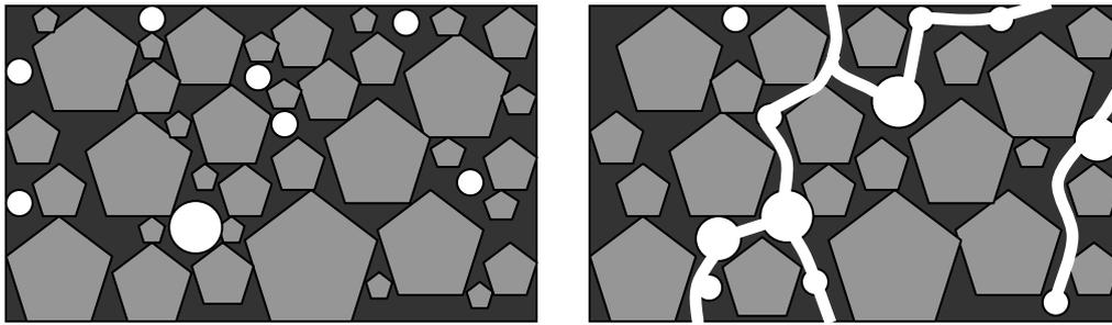
Fig. 3: If more air voids are present, they are likely to be in connection, and thus water can percolate more easily.
