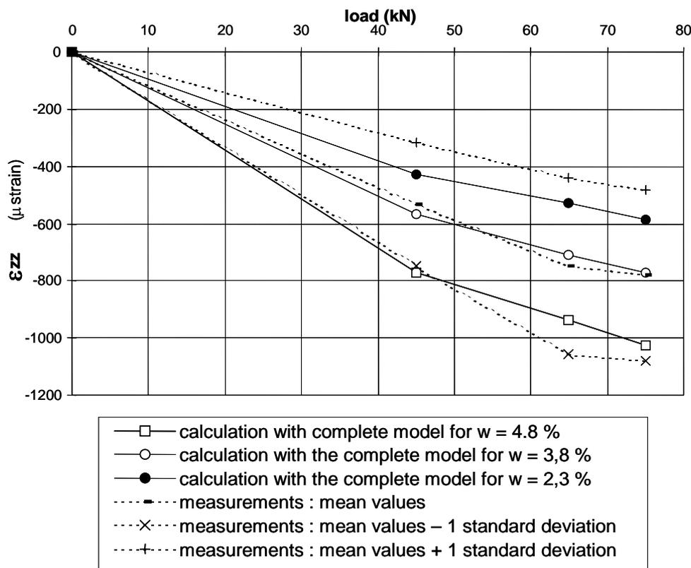
Fig. 15: Comparison of experimental and predicted maximum vertical strains at the top of the granular layer for 3 load levels (Watmove, 2008).
