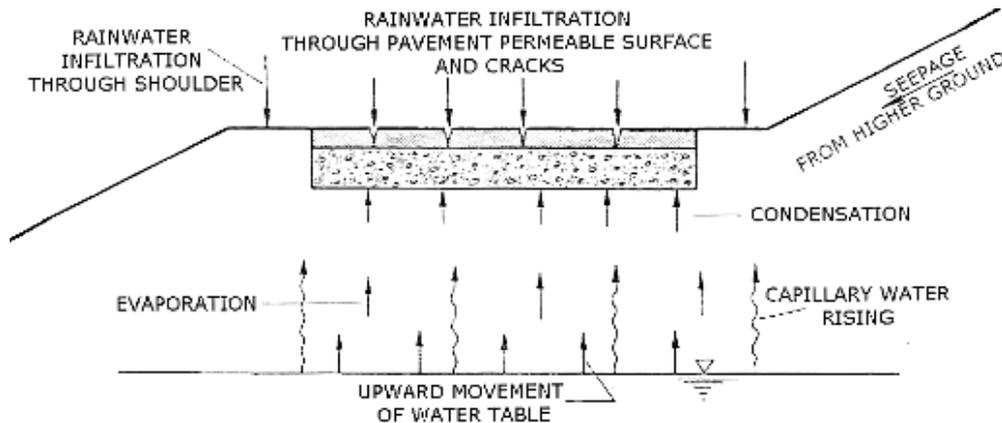
Fig. 6: Possible water movements into the pavement zone (from Moris & Gray, 1976)
