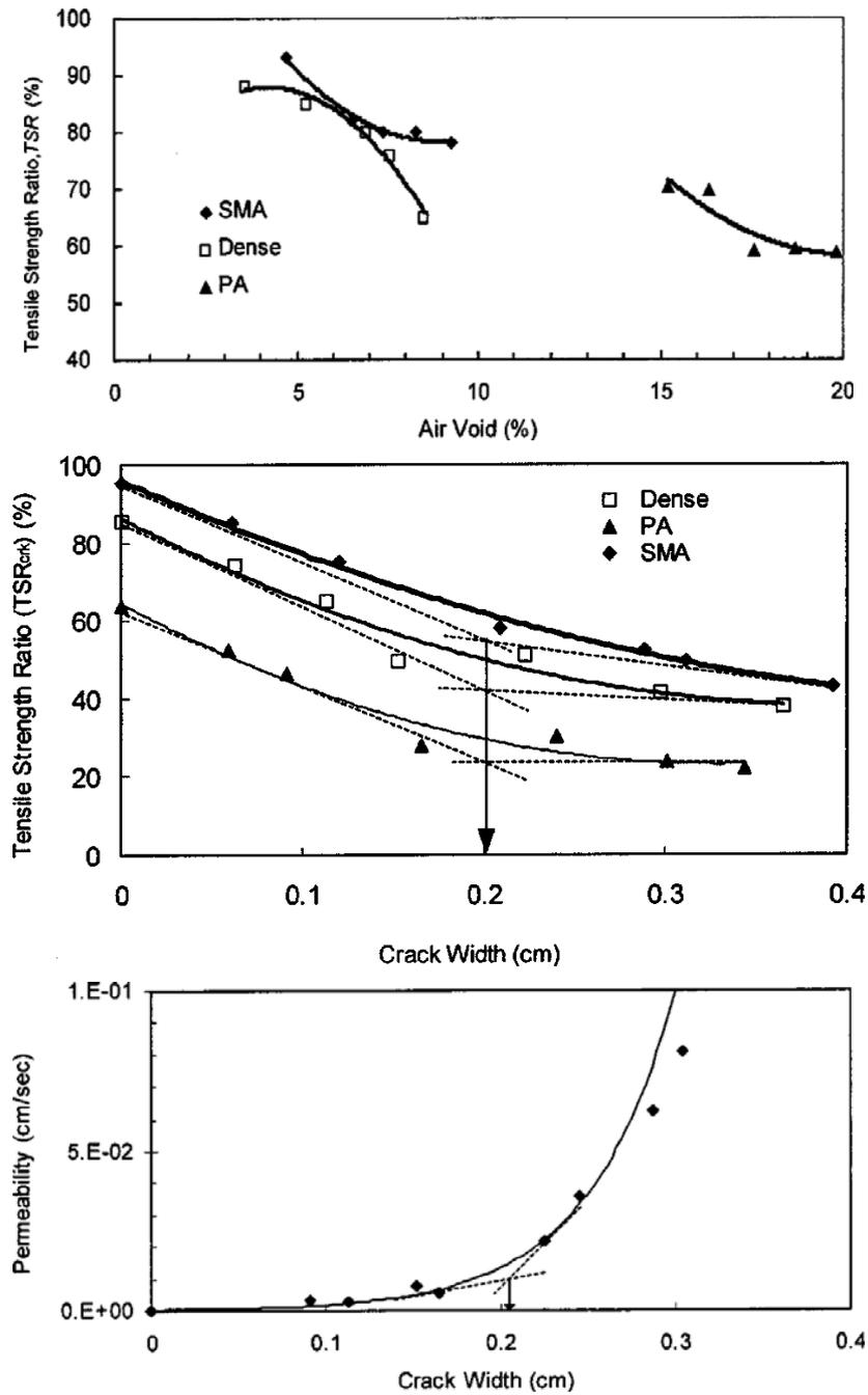
Fig. 5: From the top, tensile strength related to the air voids, to the crack width and permeability increase with the crack width (Chen et al., 2004).
