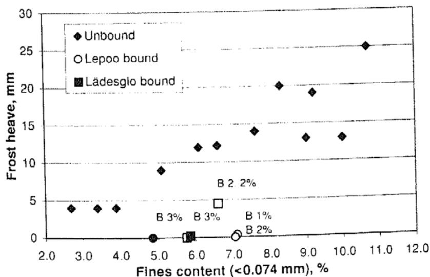
Fig. 9: Relationship between fines content and frost heave measured in the triaxial specimens during a freezing stage (Kolisoja et al., 2002).
