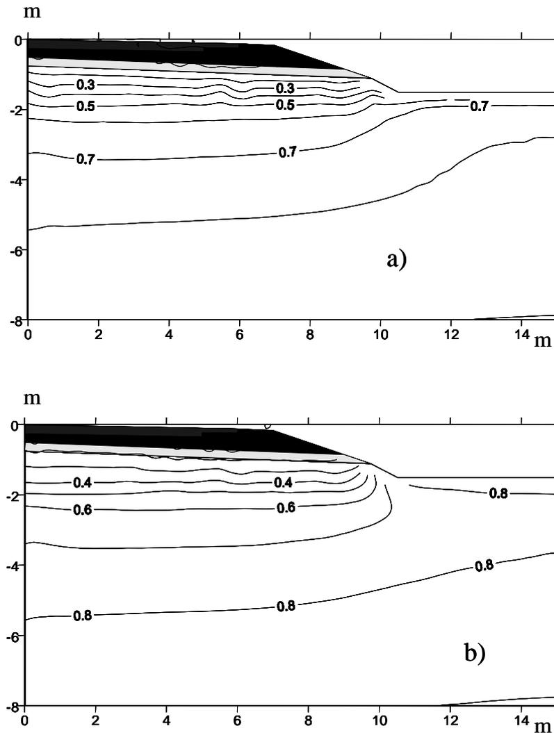
Fig. 13: Distribution of degree of saturation in a Mediterranean climate. Evaporation through pavement allowed; a) 1st July, b) 1st December (Alonso et al., 2002).
