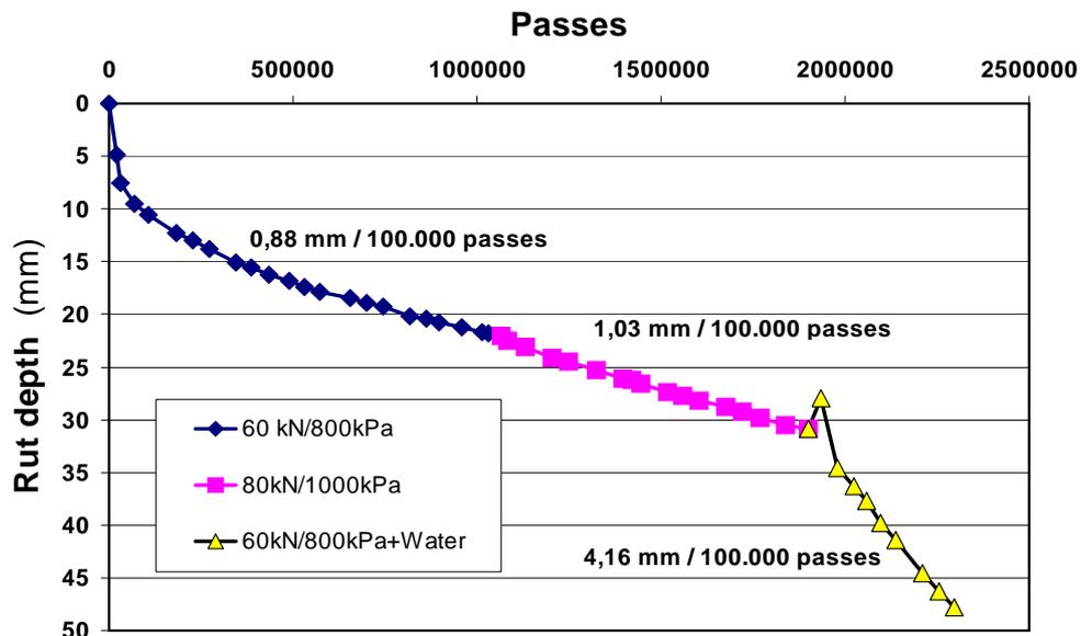
Fig. 7: Rut depth propagation rates for different conditions (from Watmove project, 2008, courtesy of L. Wiman).
