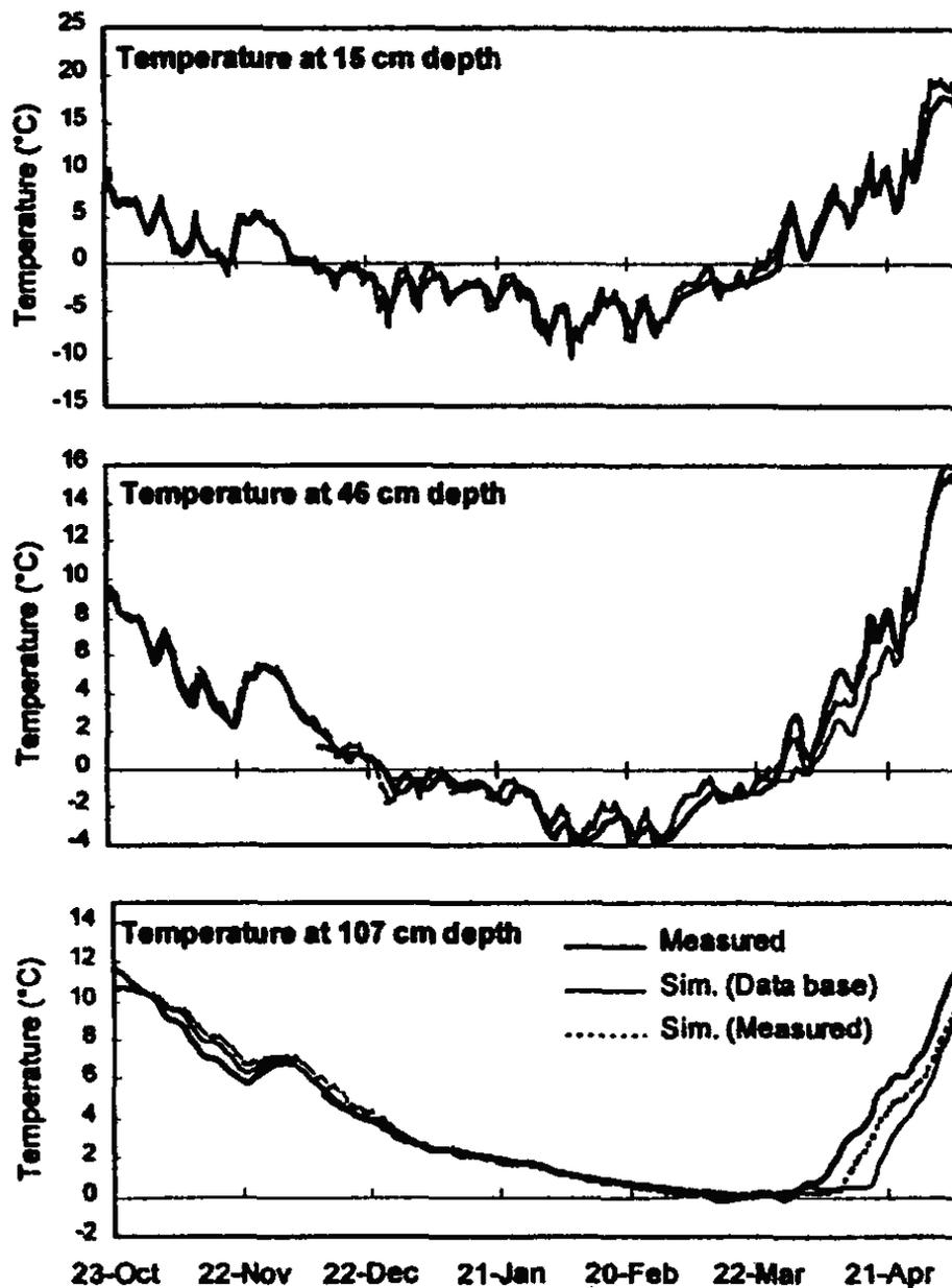
Fig. 18: Measured versus predicted temperatures (Simonsen, 1997).
