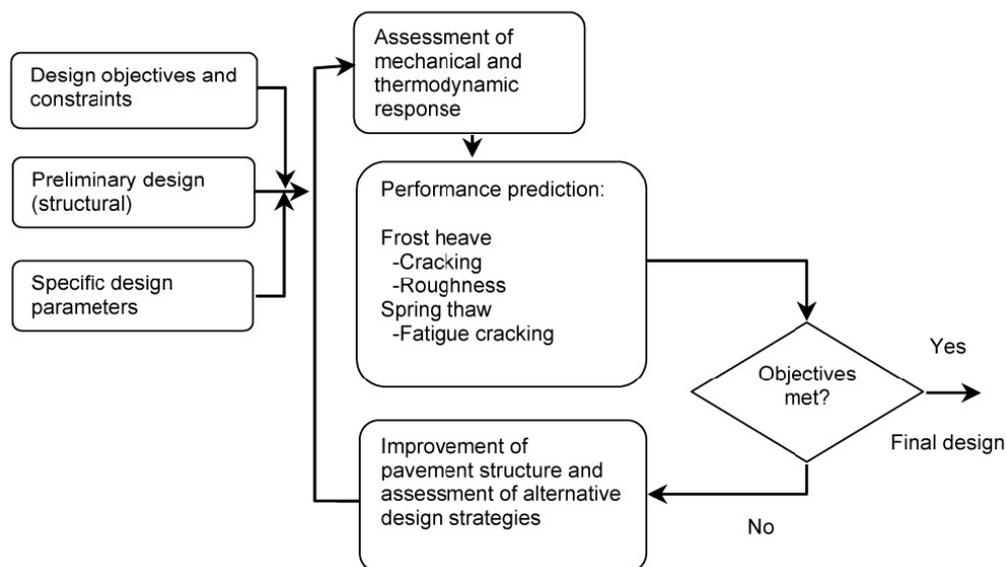
Fig. 16: Scheme of the so called “ADAAGE” procedure for the verification of pavement structures in freezing and thawing conditions (Dore’ et al., 2002).
