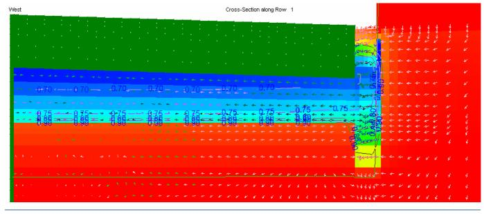
Model of an asphalt-surfaced pavement showing percolation flows at the end of a heavy rain event. Note the inability of the lateral drain to carry the run-down to the outlet pipe fast enough. Also note the undesirable movement of water from the lateral drain into the subbase. Redder = more saturated, Blue = drier.
