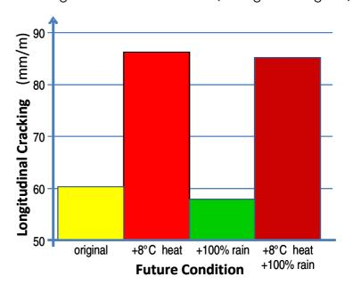
Longitudinal, top-down cracking after 20 years for a major pavement (325mm asphalt) subjected to constant 'worse-case' conditions
