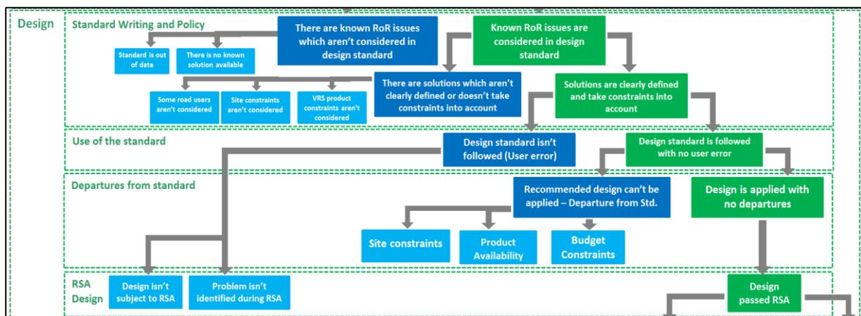
**Figure 4 – Design Phase of Roadside Safety Organisational Robustness Fault Tree**
