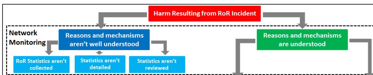
Figure 3 – Network Monitoring Phase of Roadside Safety Organisational Robustness Fault Tree
