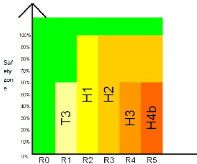
**Figure 14 – Recommended Minimum Containment Levels (Flanders) (Agency for Roads and Traffic, 2013)**
