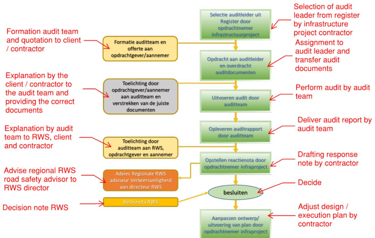
**Figure 19** – Safety Audit Flow chart including decisions and steps of the audit process (Ministry of Transport and Environment, 2018)
