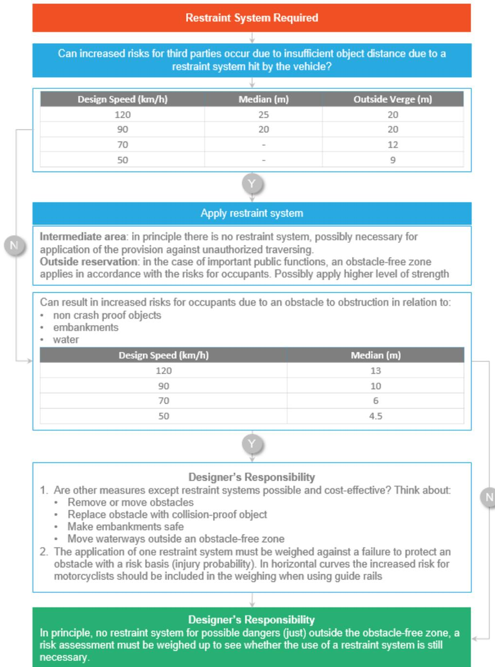
**Figure 15** – Road Restraint System Flow Chart (Dutch Ministry of Infrastructure and the Environment, 2017)
