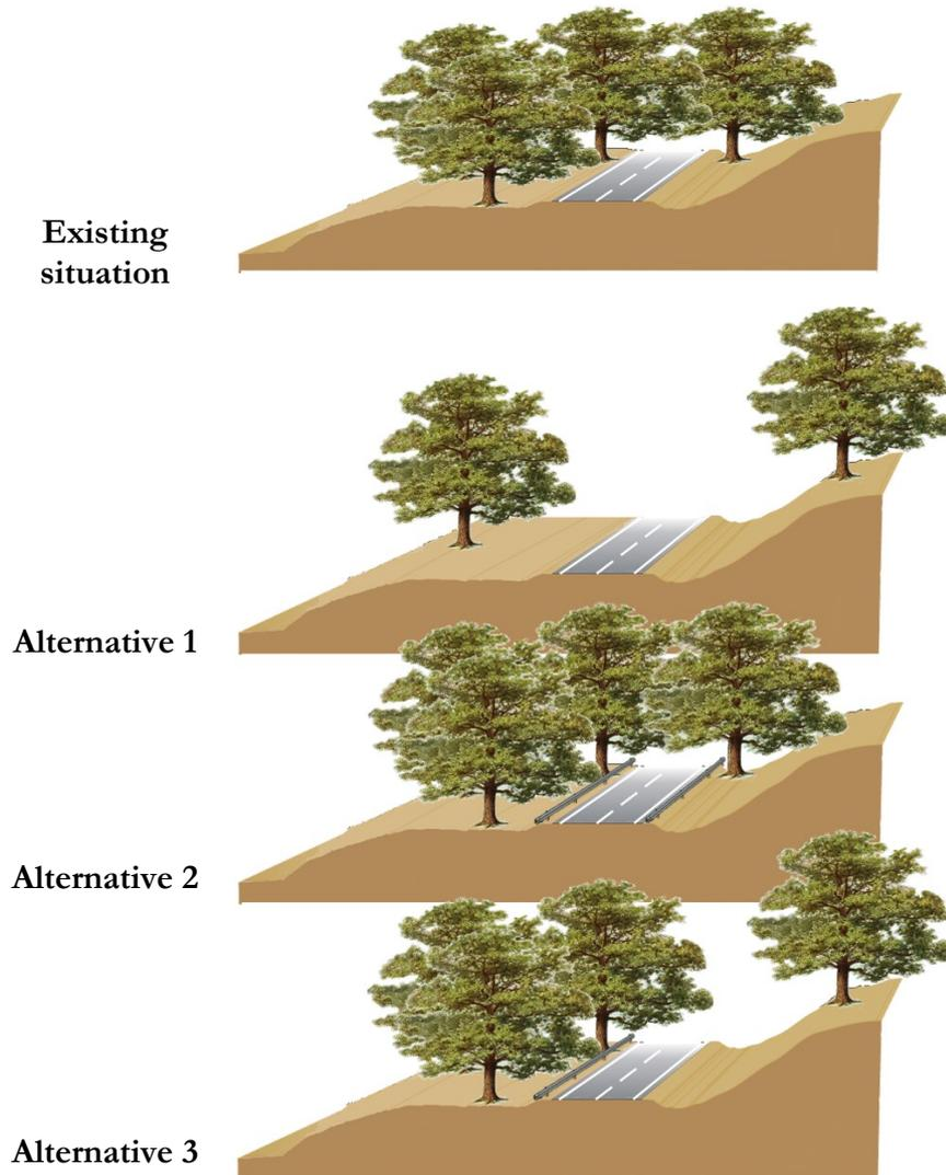
Figure 3 – Alternative roadside safety interventions (Roque and Cardoso, 2015)
