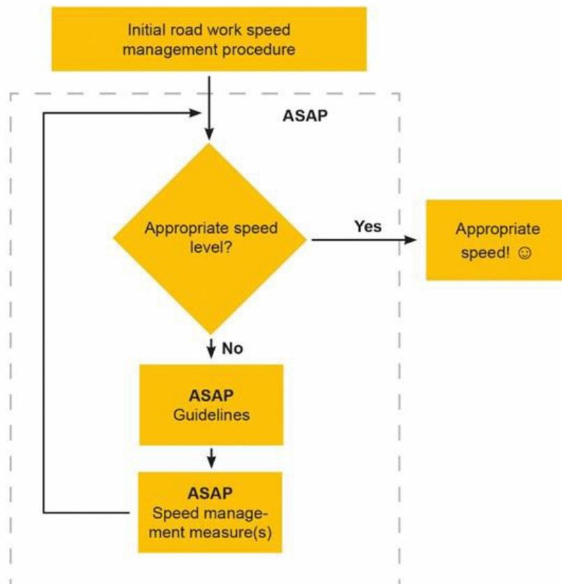
**Figure 5** – The ASAP procedure of roadwork speed management (Sorensen et al., 2015).
