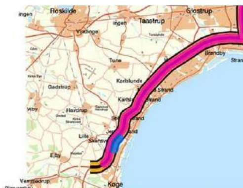
Figure 9 - The M10 motorway in Denmark; the blue marking represents a vulnerable road stretch to flooding due to low capacity of storm water runoff. (Bles, T. (2) et al. , 2015)
