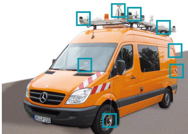
Figure 9: Integrated Road Information Scanner I.R.I.S (LEHMANN & PARTNER)
