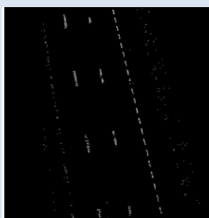
Figure 16: The detected candidate lane marking points in 3-D
