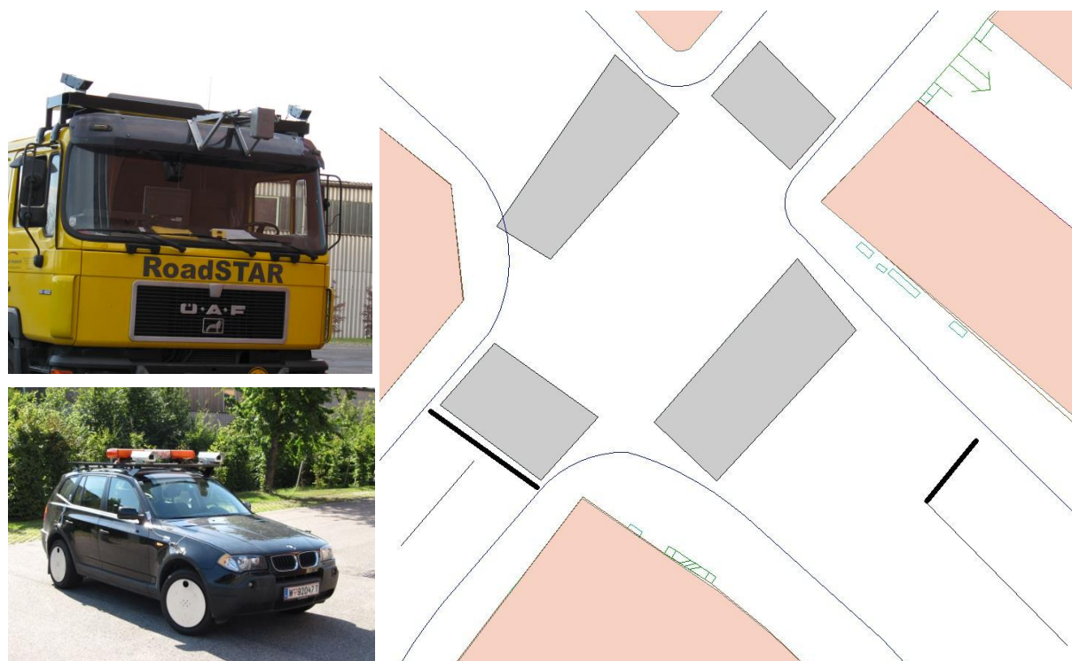
Figure 13: The two survey vehicles (truck and passenger car) (left). Example of road markings inventory derived from video survey (right)
