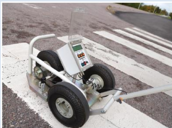
Figure 61: Portable Friction Tester, PFT. Photo: Mohammad-Reza Yahya, VTI.
