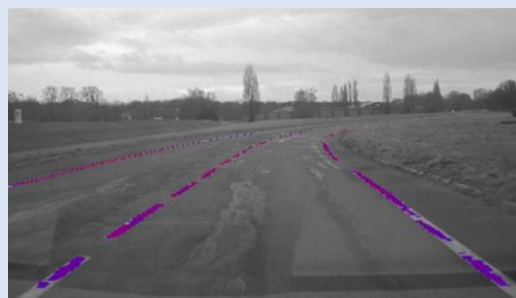
Figure 54: Road marking feature extraction
