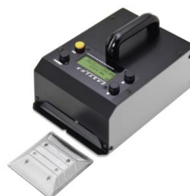
Figure 47: Hand-held reflectometer for the measurement of night time visibility of road studs (EasyLux)
