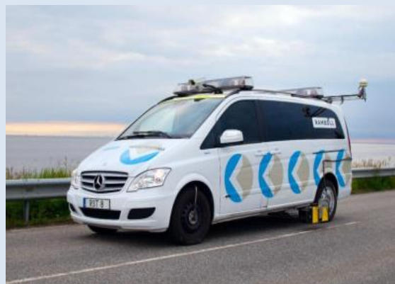
Figure 43: Mobile measurement system using LTL-M and an optocator for measurement of the road marking profile.
