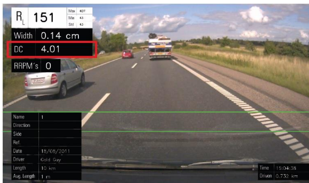
Figure 50: Day-light contrast measurement using LTL-M retroreflectometer
