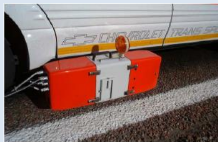
Figure 22: Mobile reflectometer Ecodyn 30
