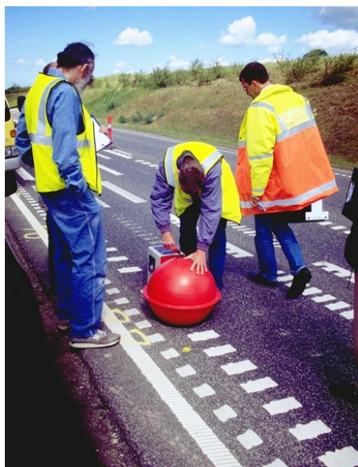
Figure 48: Hand-held reflectometer for the measurement of Q_d
