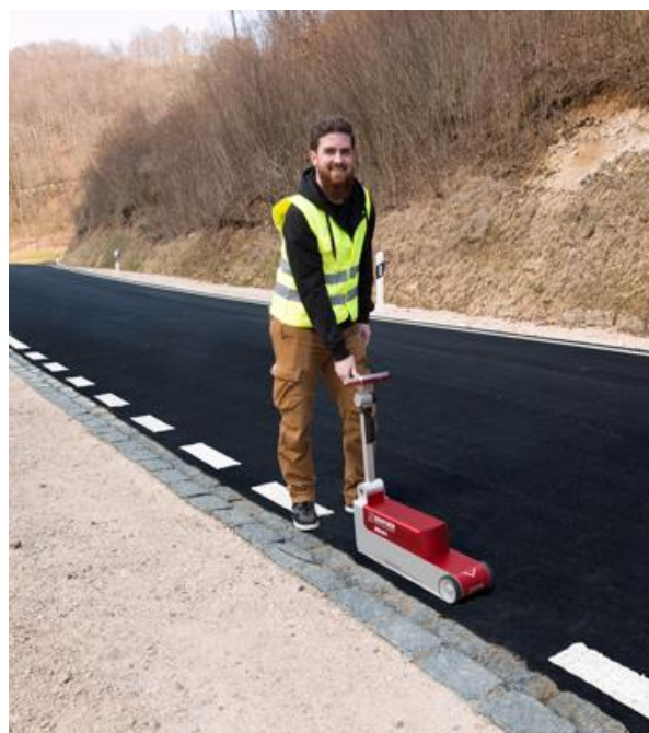
Figure 49: Hand-held reflectometer for the measurement of R_L and Q_d
