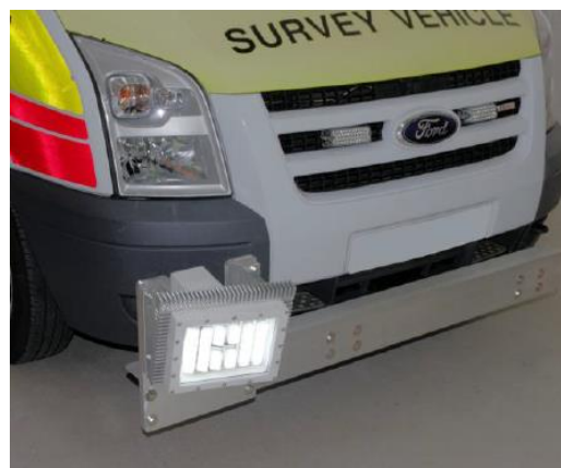
Figure 36: LED lighting system used for Marking Collector
