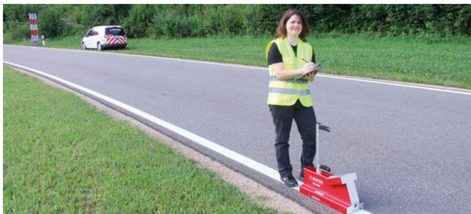
Figure 19: Measuring the night time visibility of road markings with hand-held reflectometer
