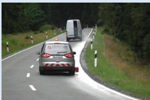
Figure 40: Equipment for wet retroreflectivity dynamic measurement
