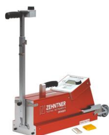
Figure 46: Hand-held reflectometer for the measurement of night time visibility of road studs (Zehntner ZRP 6030)
