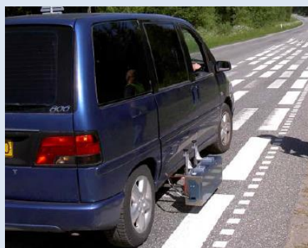
Figure 23: Mobile reflectometer LTL-M
