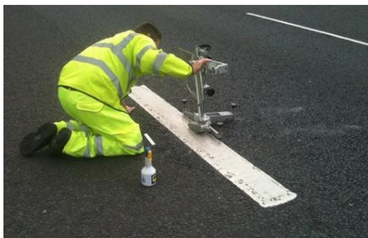
Figure 60: Measuring the Skid Resistance of road markings with portable Skid Resistance Tester
