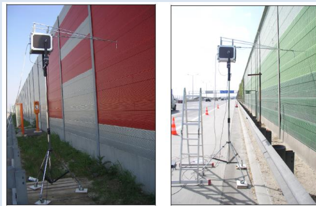
Figure 34: The measurement equipment by the new barrier (built 2005, left) and by the old barrier (built 1994, right)
