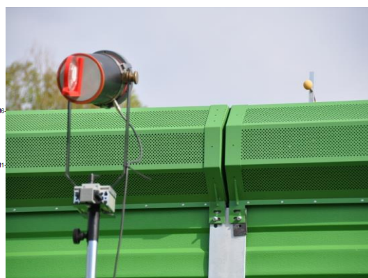
Figure 37: Standard set up of the in-situ measurement of sound diffraction
