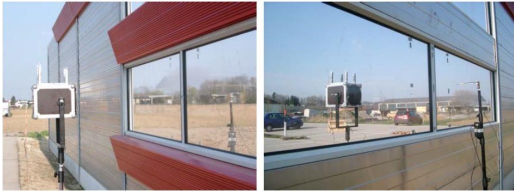
Figure 21: Standard set up of the ADRIENNE method for measurement of airborne sound insulation, using a single microphone moved around the 9 microphone positions (source AIT)
