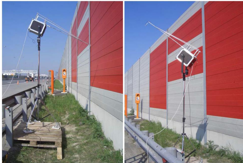
Figure 27: Standard setup of the Adrienne method: the equipment is shown during the sound absorption measurement (left) and during the free field measurement (right) according to CEN/TS 1793-5 (source AIT)
