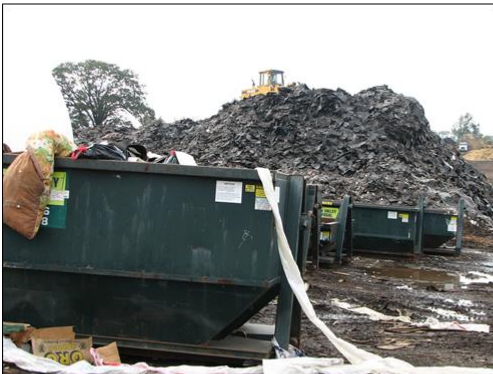
Figure 5-4 Roofing shingles sorted in the background with metal dumpsters for any rejects to be sent to landfill (Photo taken from Grefe, 2007)
