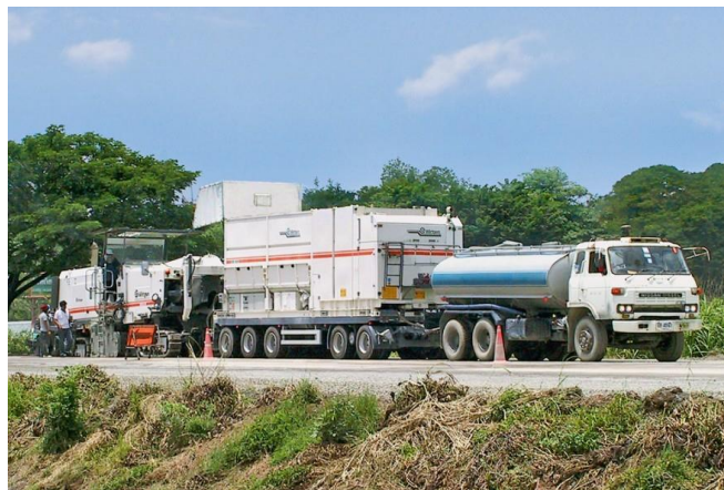
Figure 3-1 Cold recycling train using foamed bitumen (from Wirtgen 2015)
