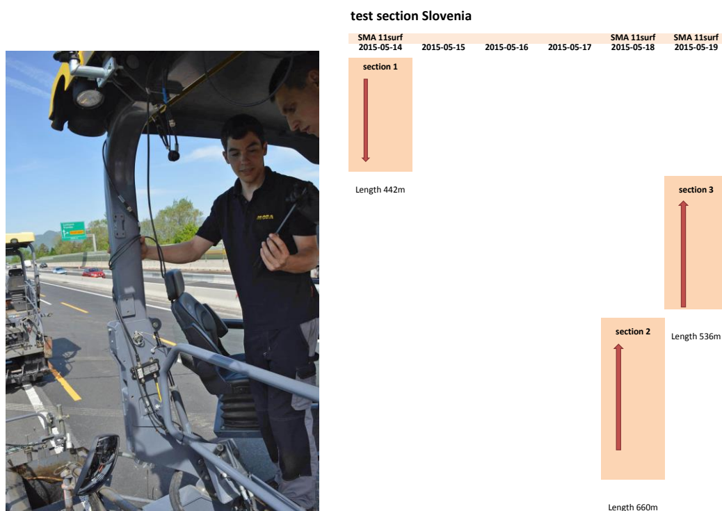
Figure 1: Time schedule and directions of paving of surface layers
