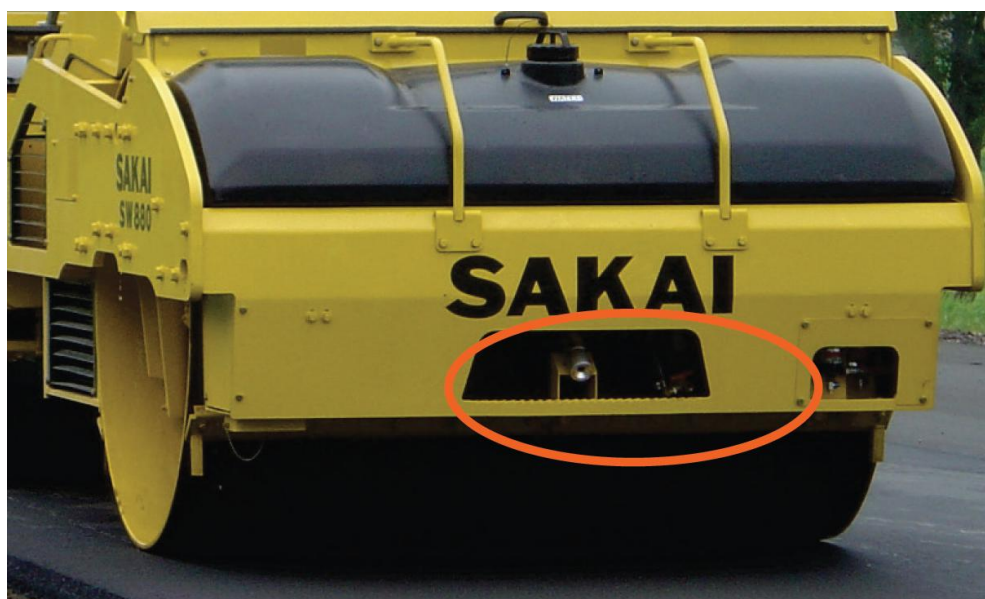
Figure 13. Infrared temperature sensor on a roller (Chang et al. 2011).
