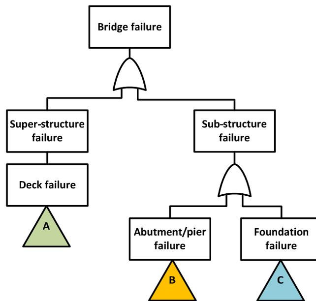
**Figure 5. Bridge failure fault tree.**
