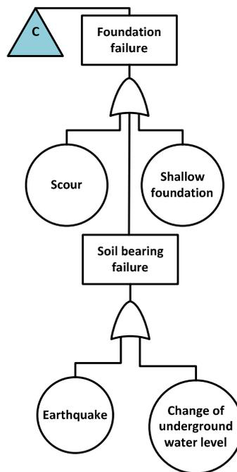
Figure 8. Fault tree analysis of foundation.
