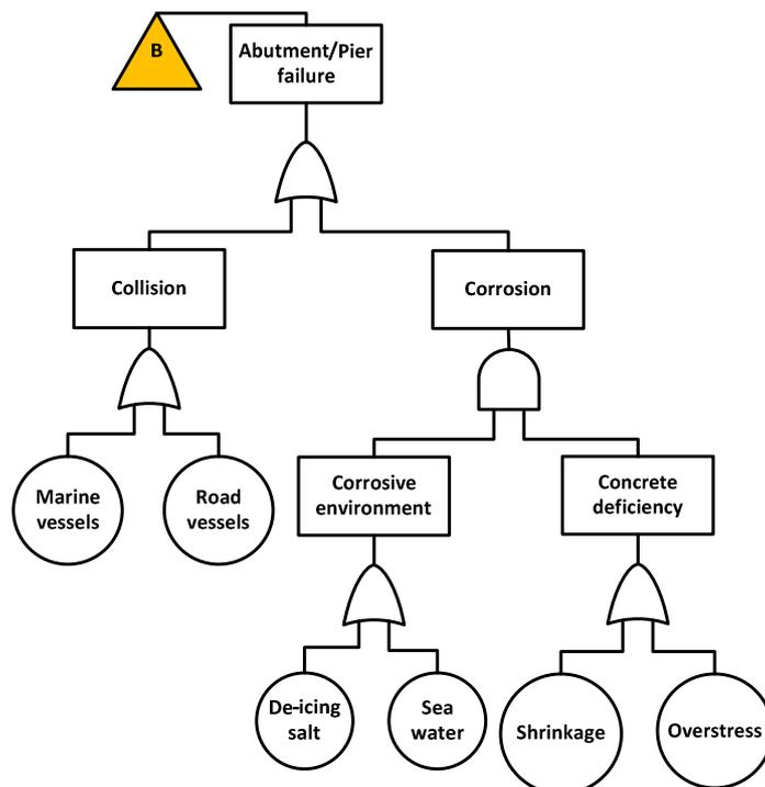
Figure 7. Fault tree analysis of abutments/piers.
