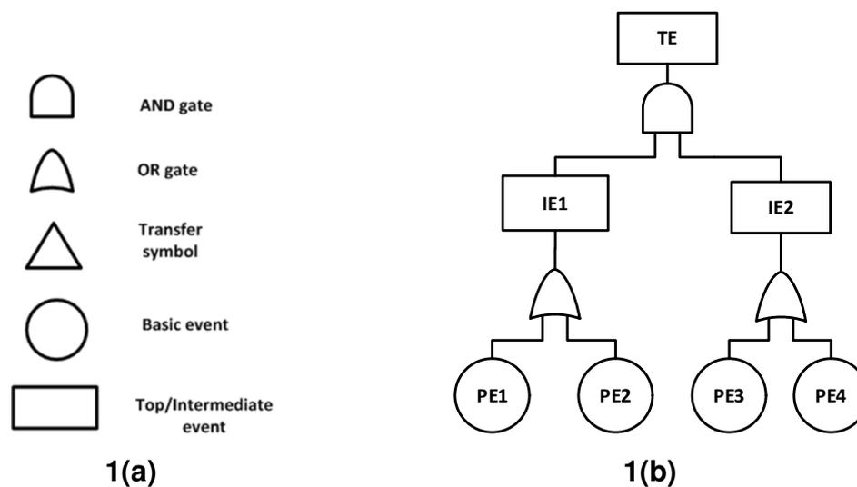
**Figure 1. Schematic representation of fault tree and its typical symbols.**
