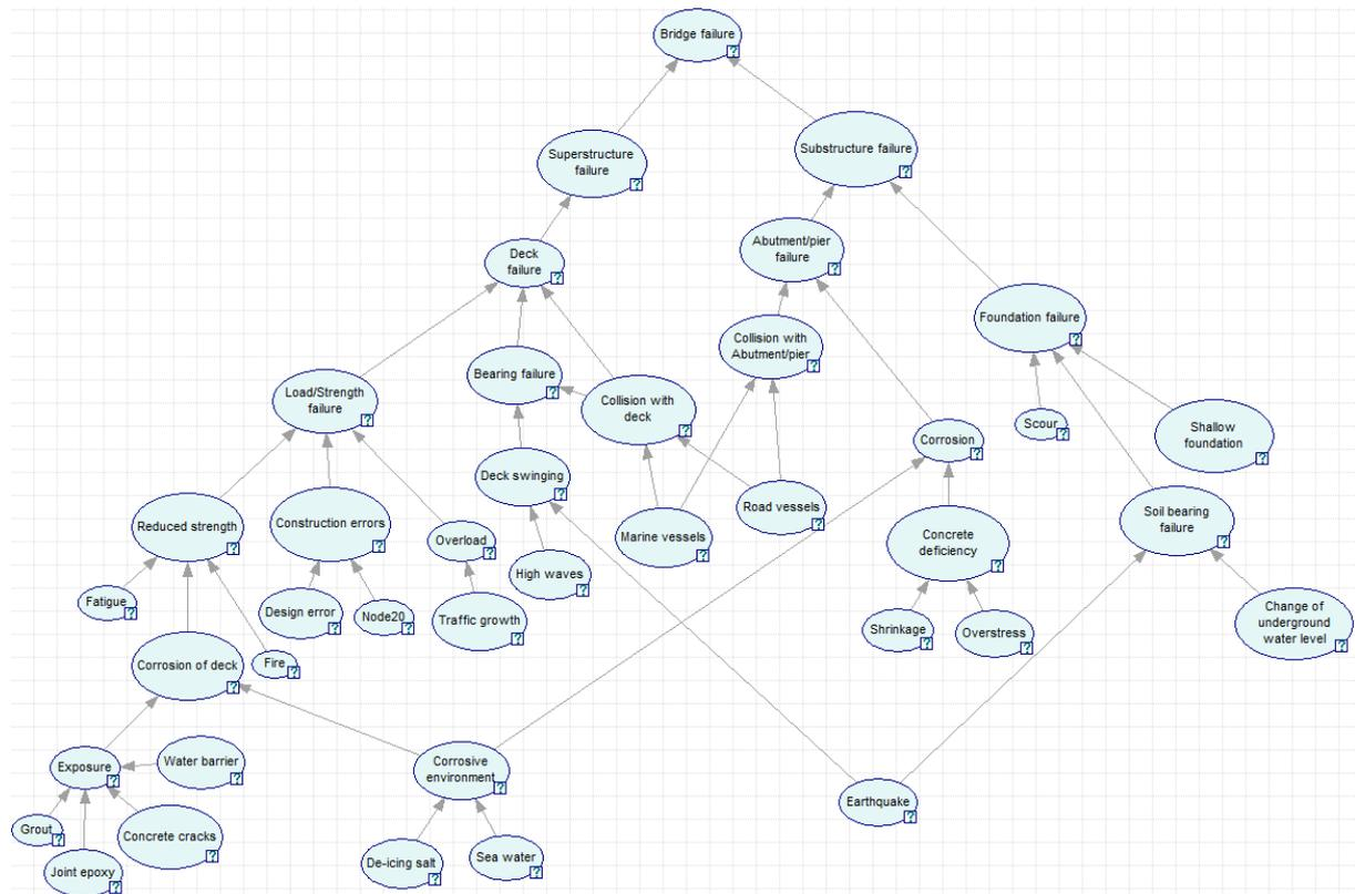
**Figure 13. Failure assessment of bridges using Bayesian network**
