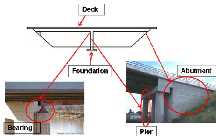
**Figure 2. Main structural elements of a bridge.**
