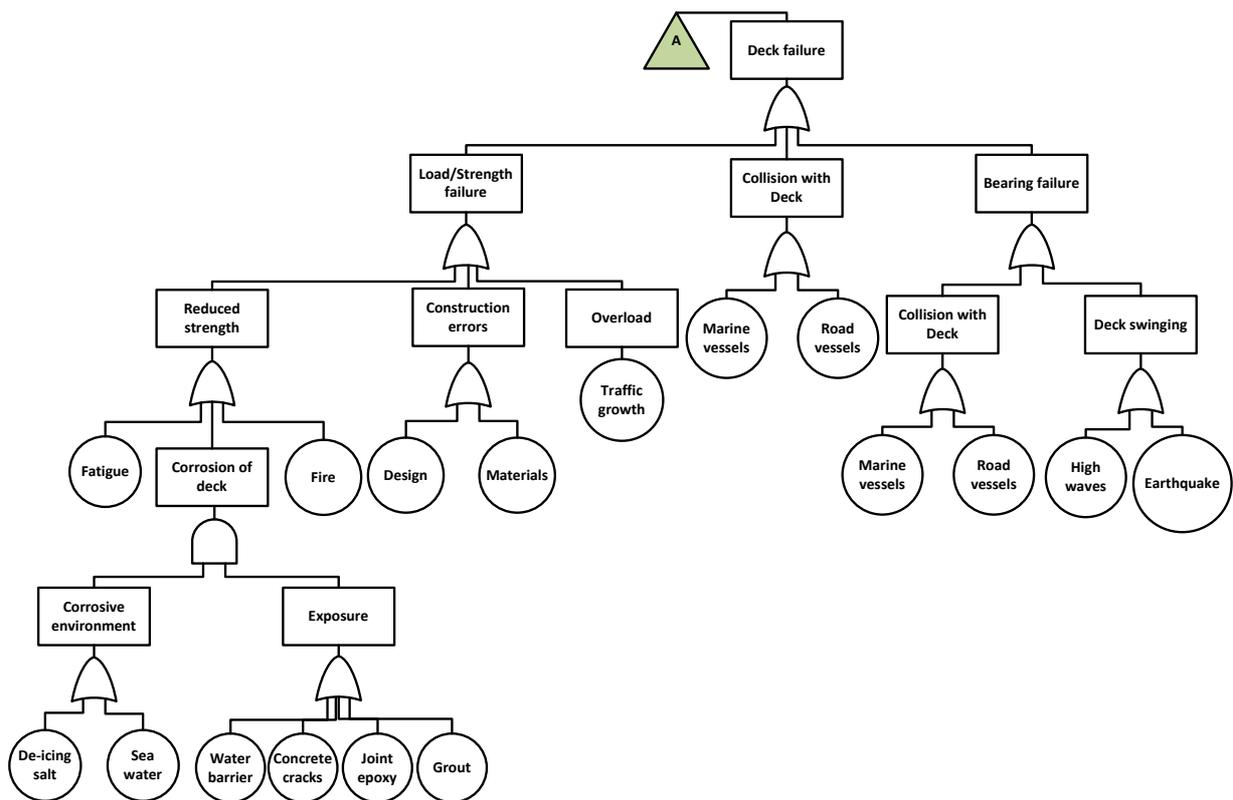
Figure 6. Fault tree analysis of deck failure.
