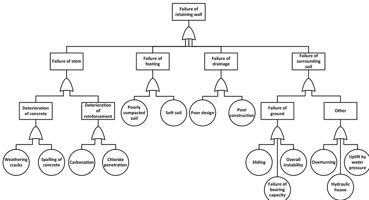
Figure 9. Fault tree analysis of retaining wall.
