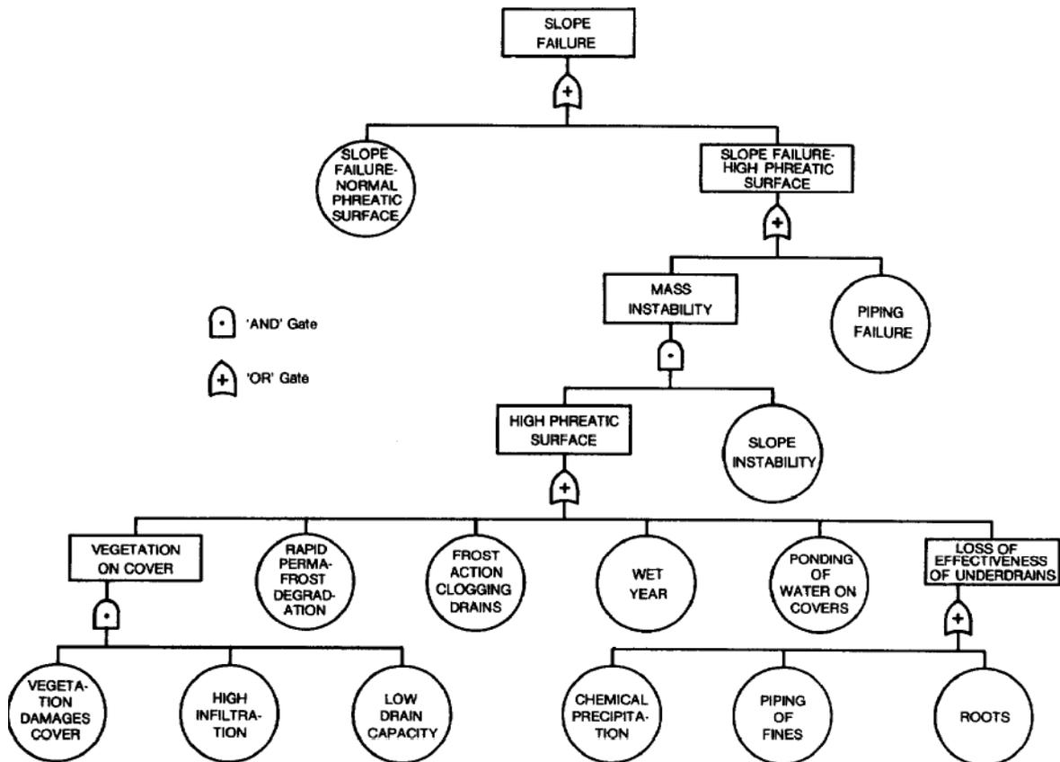
Figure 10. Fault tree analysis for slope failure (Van Zyl and Robertson, 1987).
