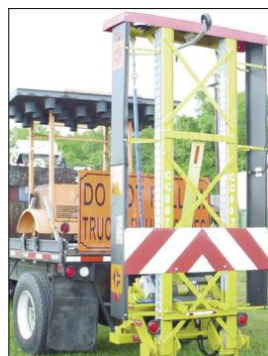
Figure 74 – Truck mounted attenuator. Photo by (Trinity highway products).
