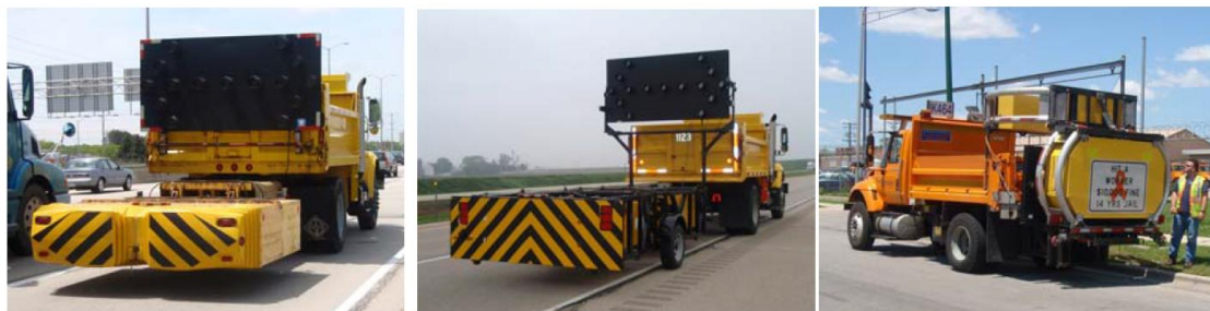
Figure 73 - Truck-mounted attenuator, trailer-mounted attenuator and attenuator in folded transport position (Steele & Vavrik 2009).
