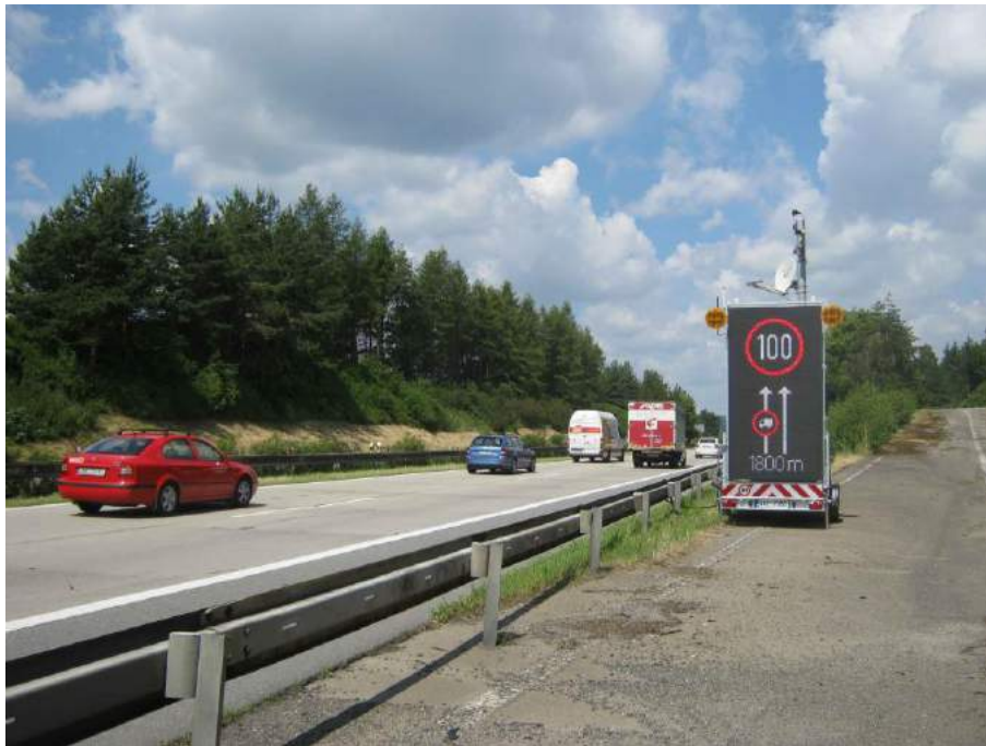
Figure 18: Deployment of the LED advance warning trailer
