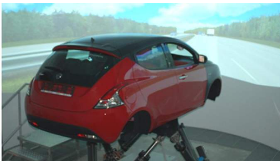
Figure 41: The dynamic driving simulator at the University of Florence
