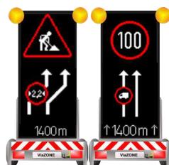
Figure 53: Advanced warning trailer scheme A and B
