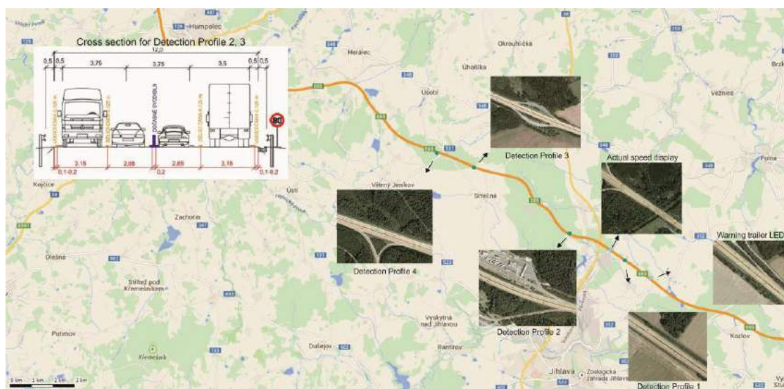
Figure 9: Road works cross section and location of the detectors
