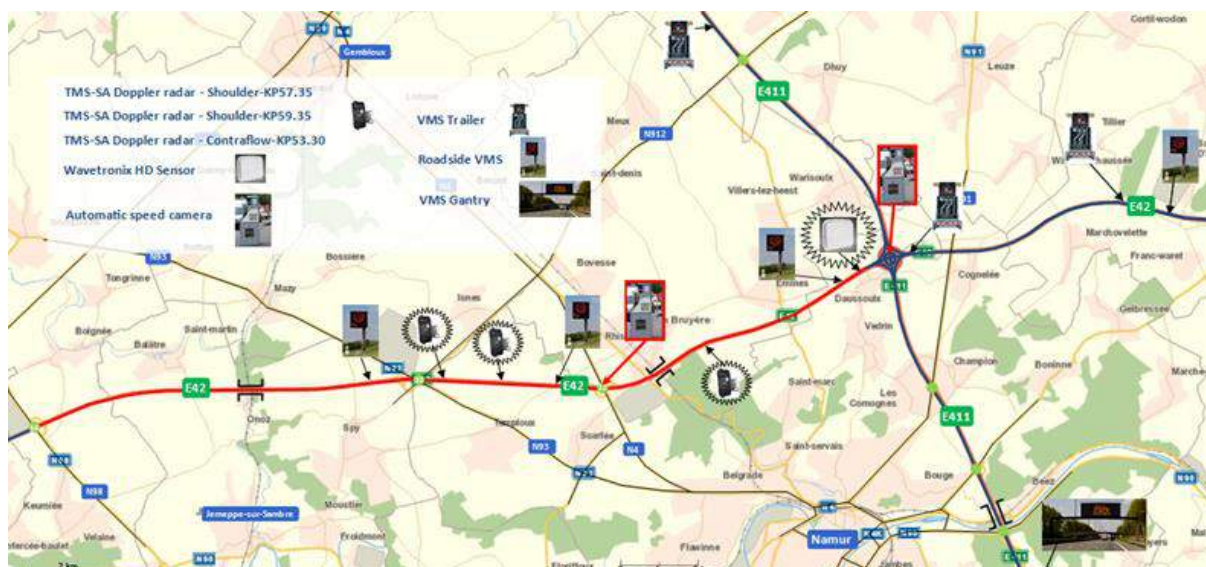
Figure 32: A15/E42 Road works - Equipment location scheme
