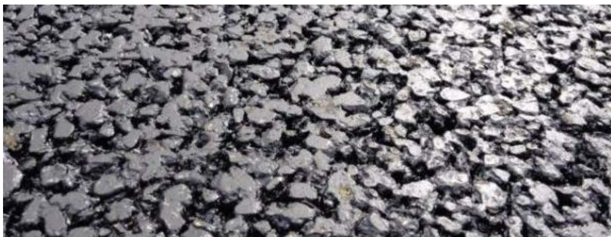
Figure 3.12: Close up of a newly laid SMA pavement with 8 mm maximum aggregate size.
