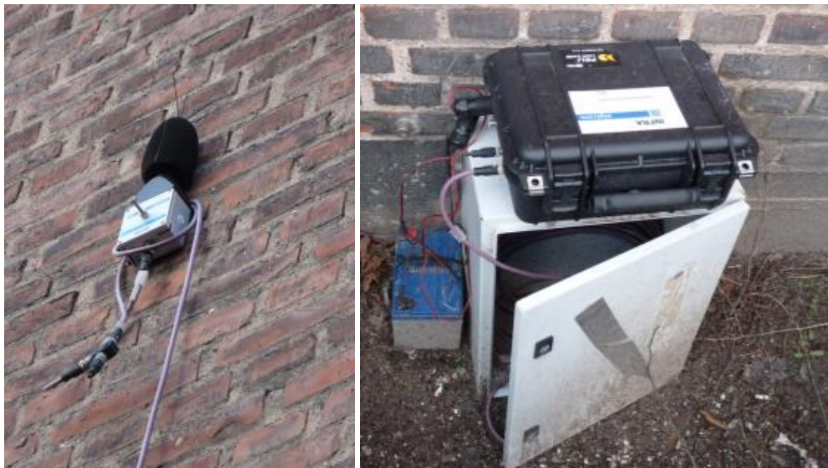
Figure 6.7: A permanent, continuous noise-monitoring station at a residential building close to a construction site. The microphone is shown on the left and the data-collecting equipment and power supply are visible on the right.
