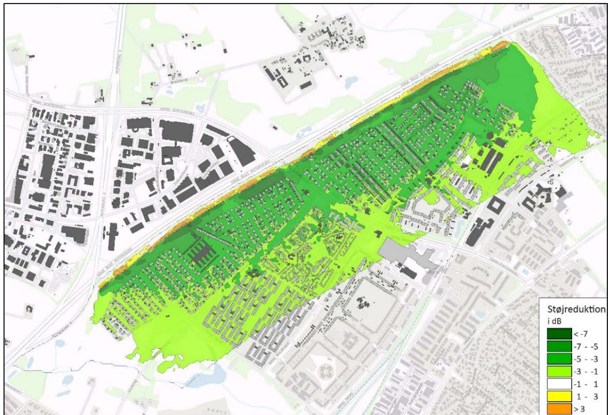
Figure 3.2: Differential noise map showing the noise reduction due to increasing a bank of earth from a height of 6 meters to 12 meters. The map shows the predicted noise reduction.
