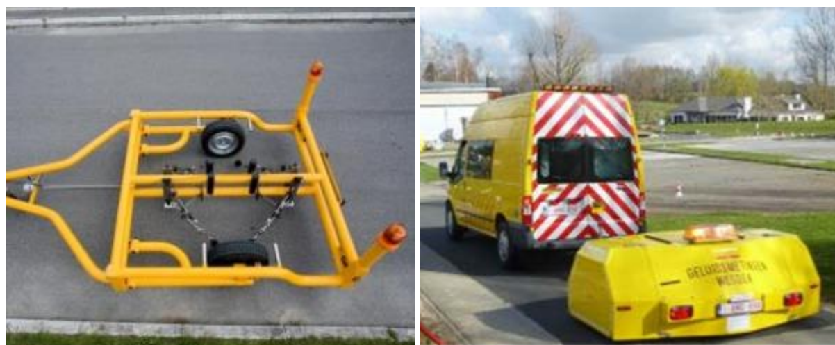
Figure 5.2: Open (to the left) and closed (to the right) CPX trailers for noise measurements on roads.
