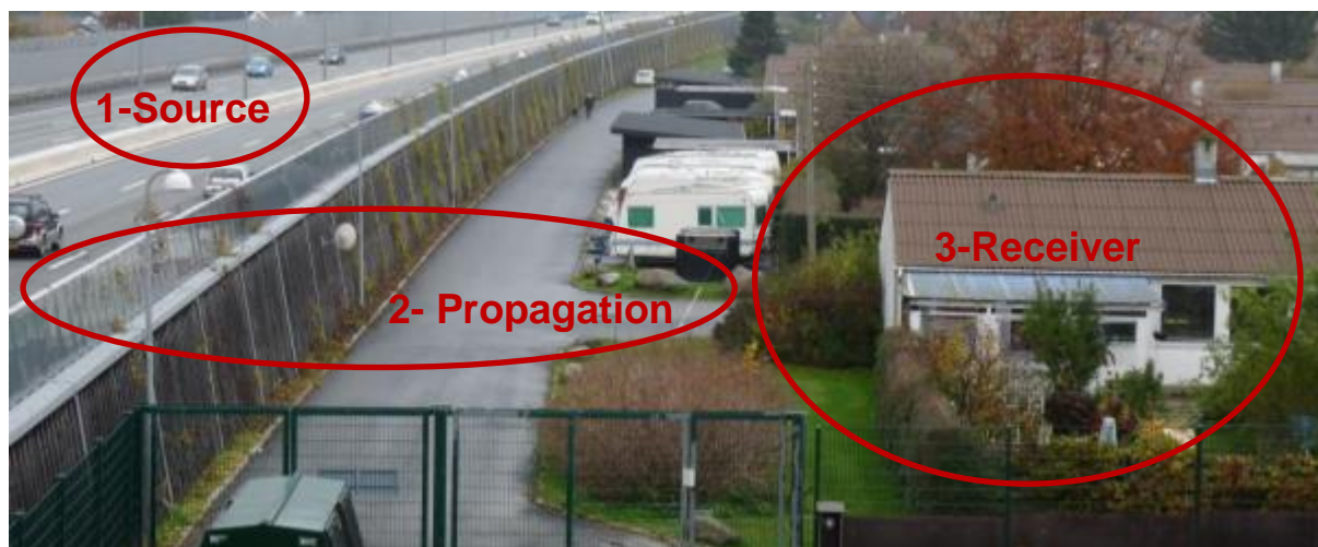
Figure 3.10: The three stages in the 'noise chain'.
