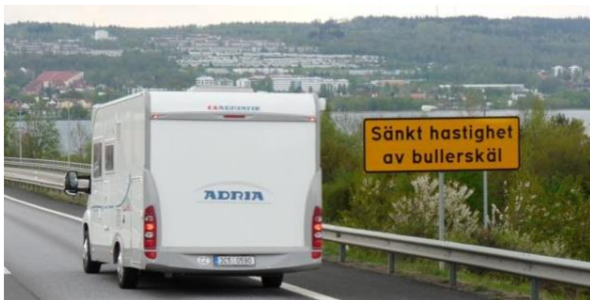
Figure 4.16: A speed reduction from 110 to 90 km/h was part of a noise reduction project along 3 km of Highway E4 passing a residential area near Husqvarna, Sweden with a traffic volume of 22 000 vehicles per day. The sign at the roadside states 'Reduced speed because of noise' (see example in Annex C for more details).
