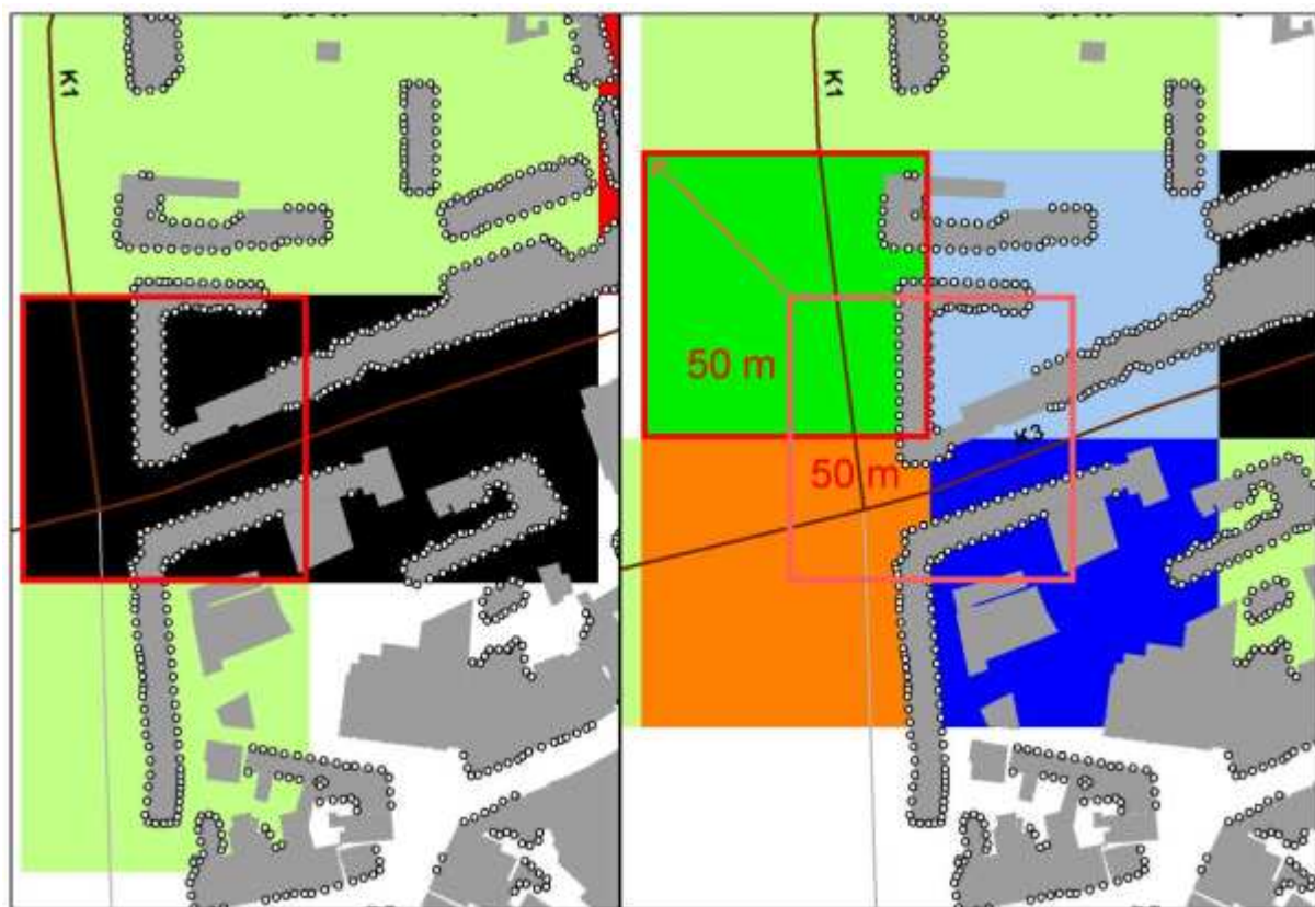
Figure 6.1: Shift of raster origin by 50 metres in x and y directions.
