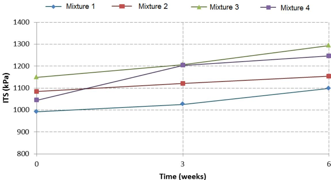
Figure 2. Effect of age hardening on indirect tensile strength
