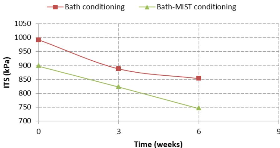
**Figure 4. Indirect tensile strength of Mixture 1 (Control; 0 % RA)**
