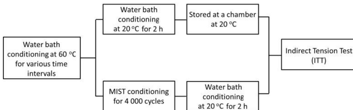
**Figure 1. Schematic of the applied moisture conditioning protocols**
