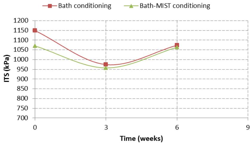
Figure 6. Indirect tensile strength of Mixture 3 (40 % RA; WMA additive)
