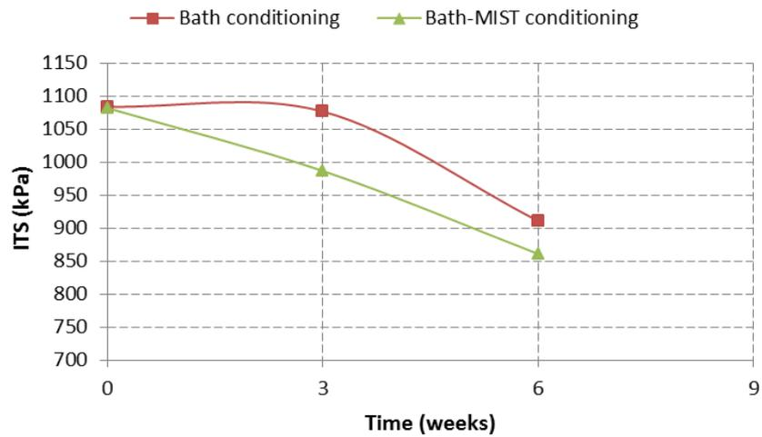
Figure 5. Indirect tensile strength of Mixture 2 (30 % RA; no WMA additive)
