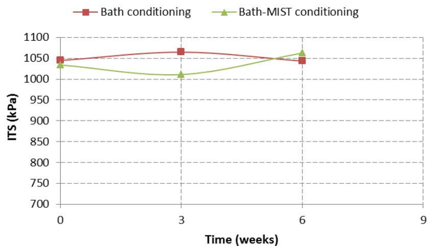
Figure 7. Indirect tensile strength of Mixture 4 (30 % RA; WMA additive)
