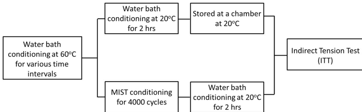
**Figure 5. Schematic of the applied moisture conditioning protocols.**
