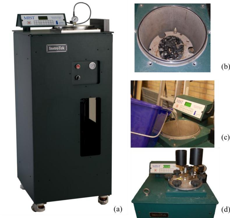
**Figure 6. Moisture induced sensitivity tester.**
