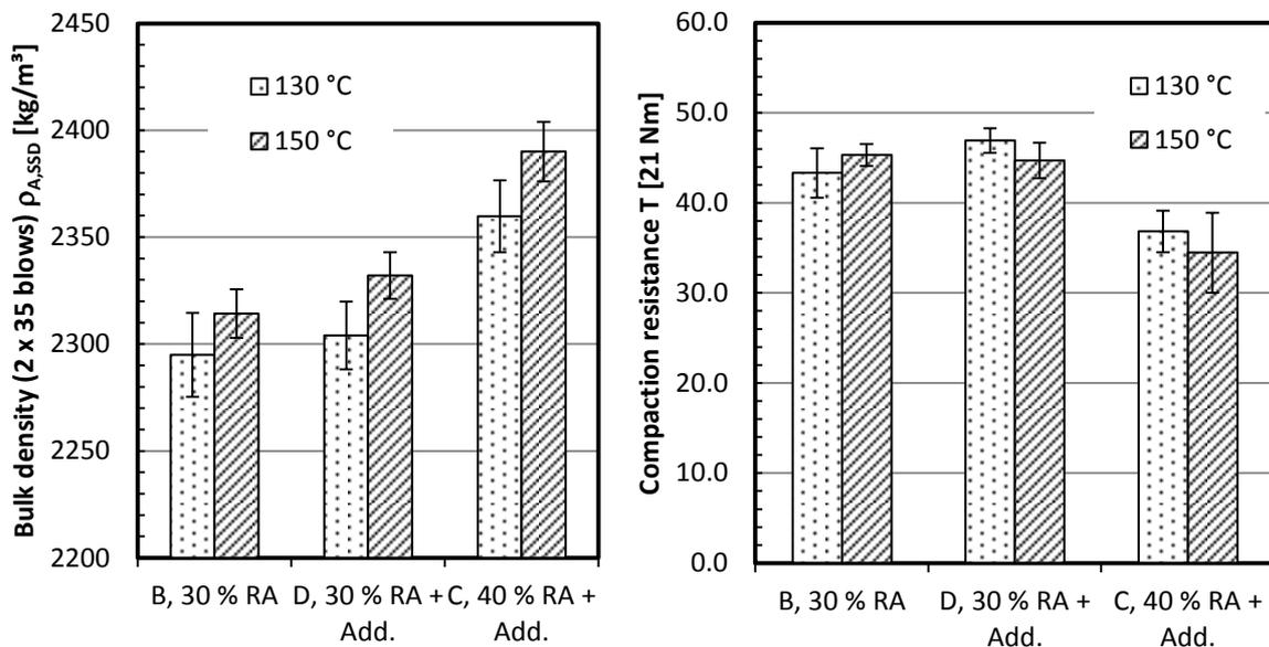
**Figure 16. bulk density of water sensitivity test specimen (left) and compaction resistance (right)**
