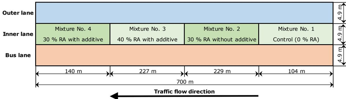
Figure 1. Schematic representation of the trail section
