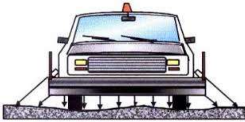
Figure 1 Example HiSPEQ recommendations for specifying transverse profile measurement
