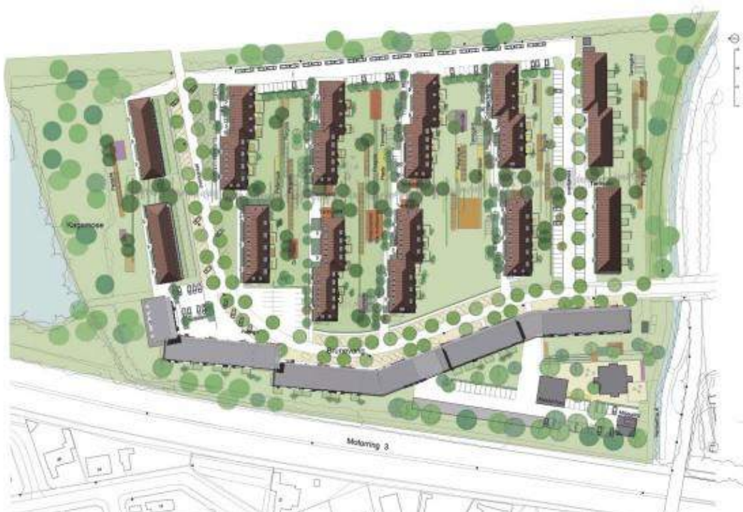
Figure 5.14: A new 'building snake' (grey blocks) will form a noise barrier between the motorway and the existing residential housing [62].
