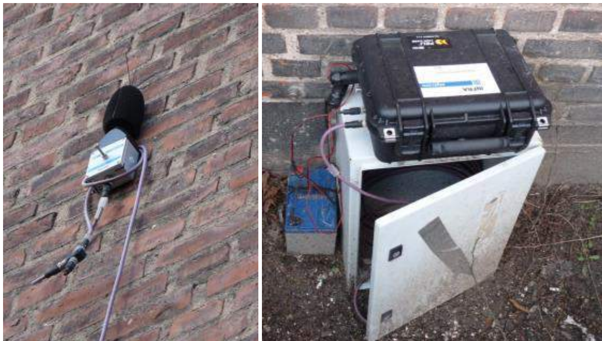
Figure 6.7: A permanent, continuous noise-monitoring station at a residential building close to a construction site. The microphone is shown above and the data-collecting equipment and power supply are visible below.
