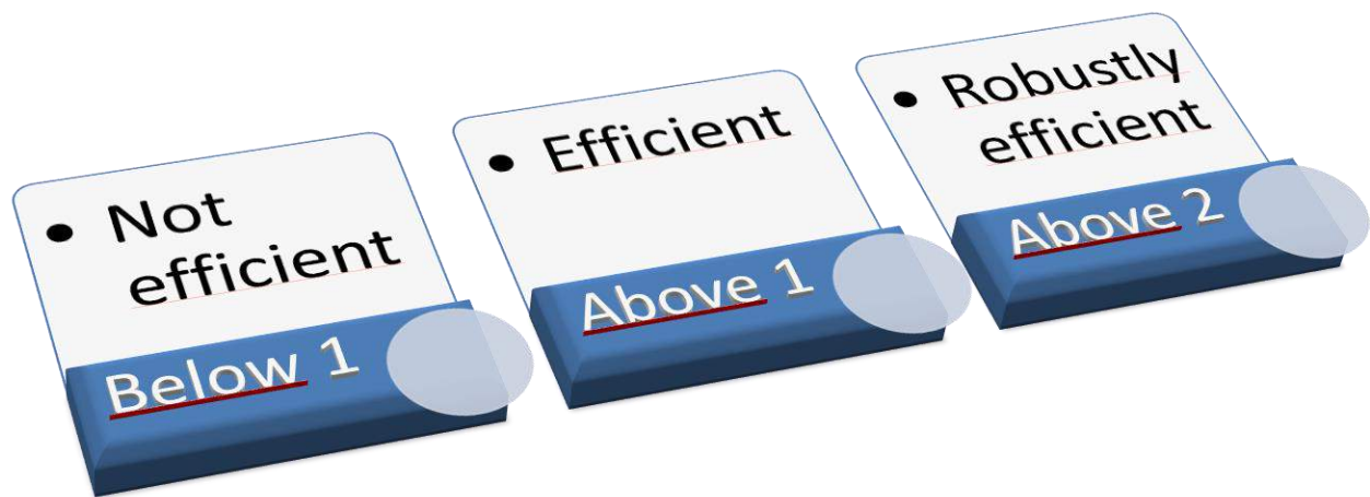
Figure A.1: The results of a CBA are often expressed in the form of a Benefit to Cost Ratio (BCR). Values above one ( BCR > 1 ) are cost efficient. However, to be competitive, projects should be robustly efficient ( BCR > 2 ).
