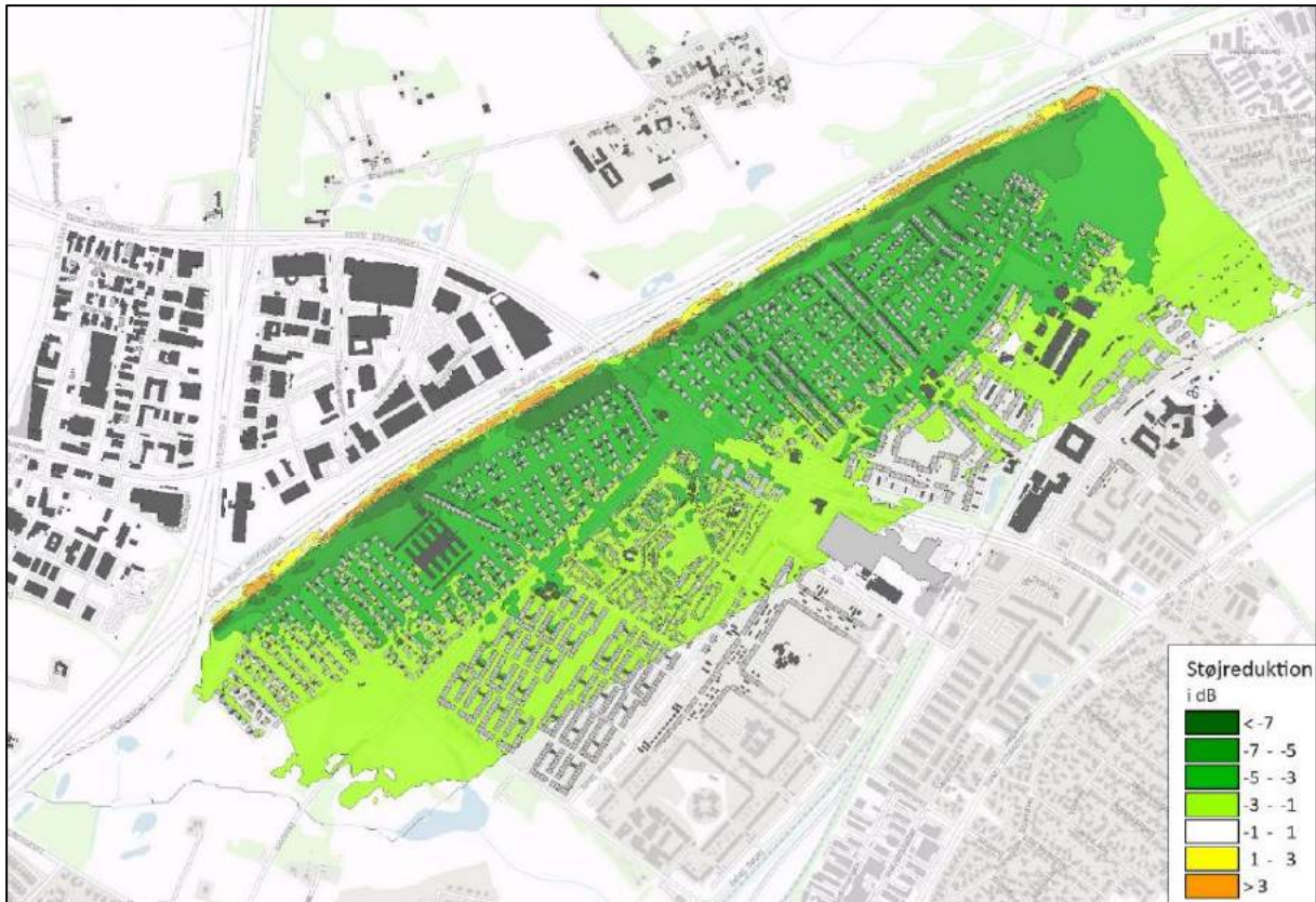
Figure 3.2: Differential noise map showing the noise reduction due to increasing a bank of earth from a height of 6m to 12m. The map displays the predicted noise reduction.
