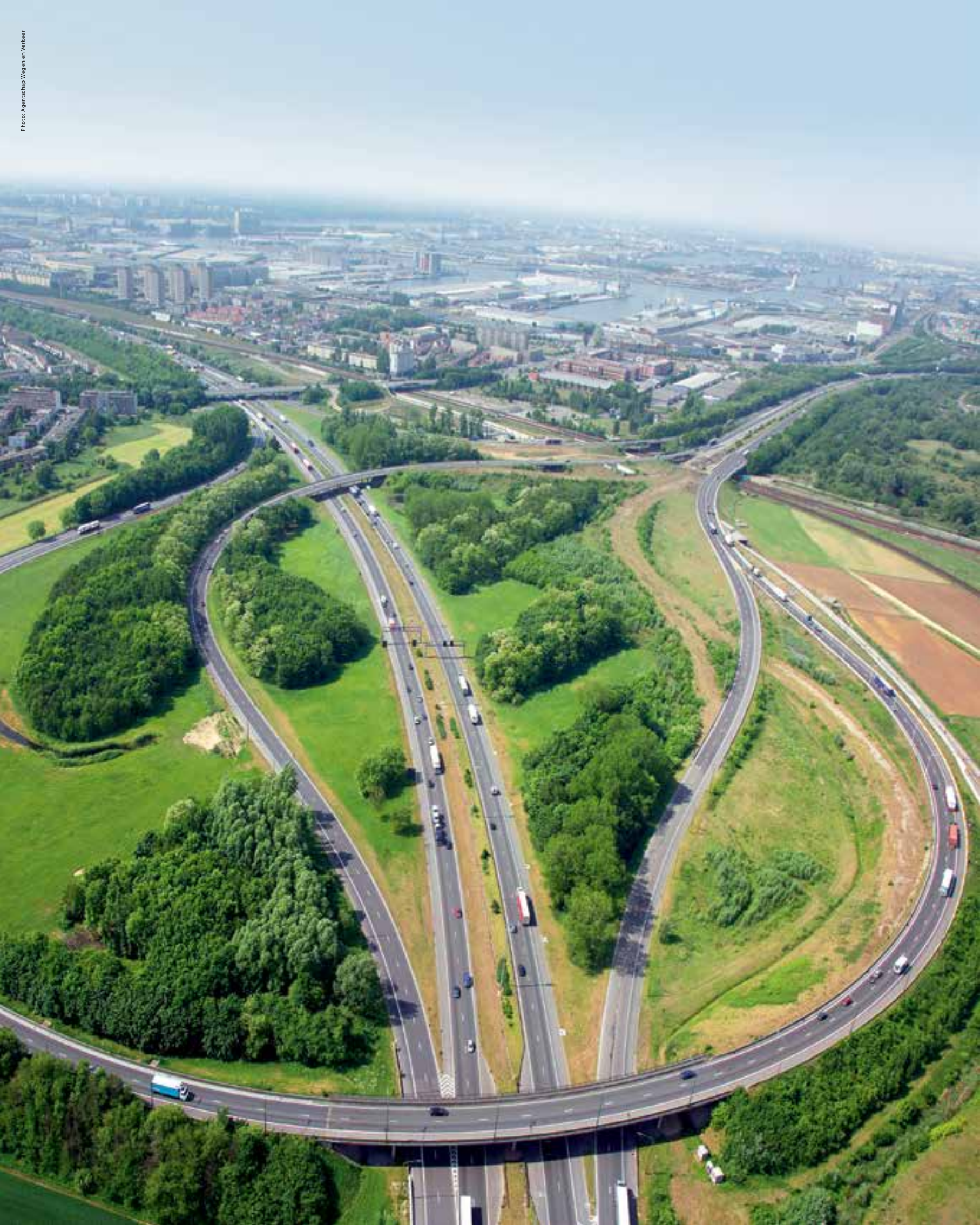
The intersection Antwerp-North is a traffic junction on the ring road around Antwerp. The shape of the Antwerp-North node is a half turbine hub.
