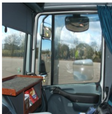
Fig. 19: Fresnel lens on LGV cab window
