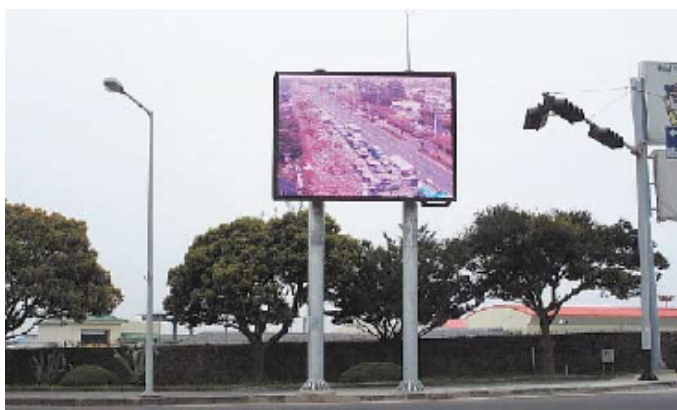
Fig. 13: South Korea : the use of dynamic image-type VMS can provide a certain amount of traffic information, including, as illustrated here, the current status of traffic a few kilometres ahead
