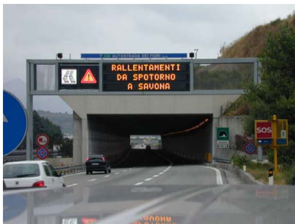
Fig. 15: Combined use of text and pictograms in Italy
