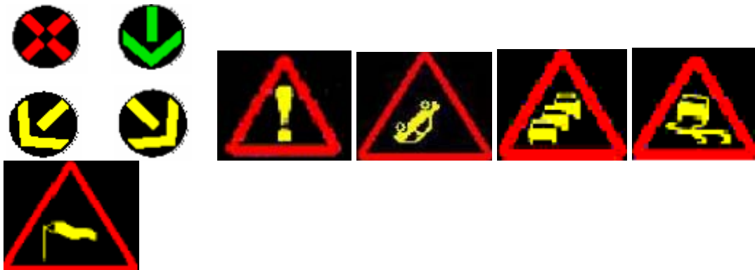
Fig. 4: Pictograms recommended by FIVE for use on VMS (the lane allocation signals have been considered here as part of the VMS set)
