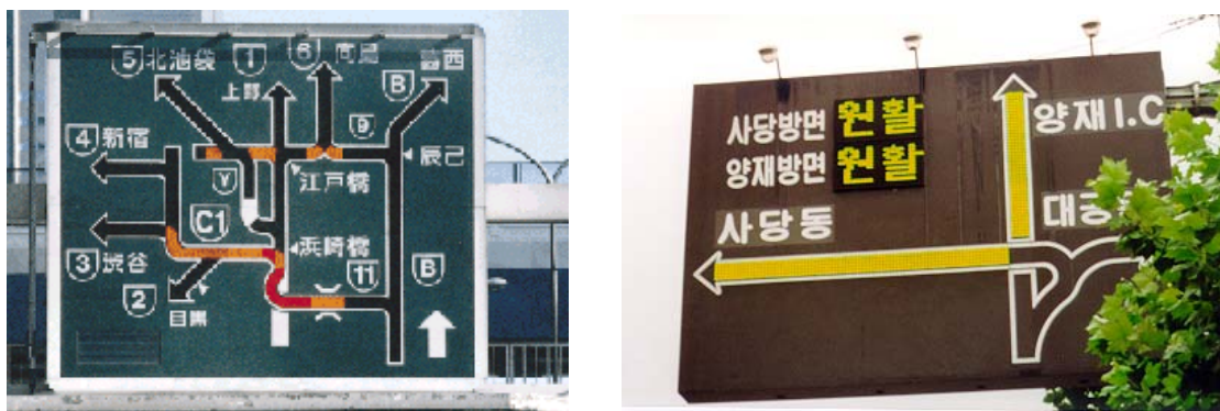
Fig. 6: Japan and South Korea have spearheaded the development of dedicated travel time and traffic status signs that provide network information
