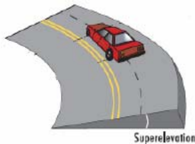
Figure 3.4. Superelevation on horizontal curves (PIARC 2003)
