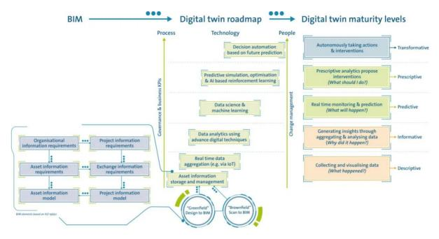
Figure 12: Process of transition from BIM to Digital twin (©2020 Royal HaskoningDHV)
