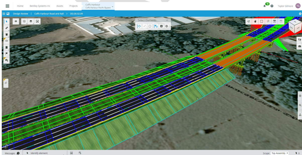
Figure 7: Digital twin built with bentley i-twin platform and azure environment (Dubey P., 2020)
