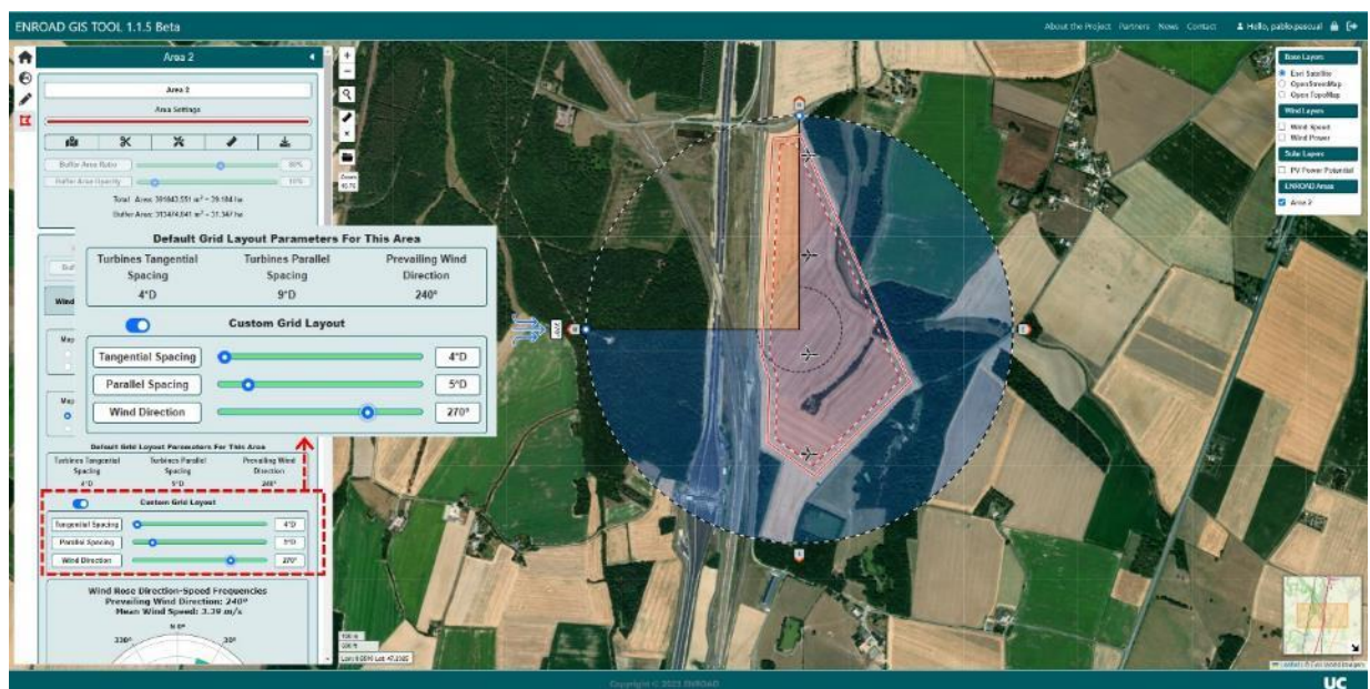
Figure 65.- Recalculation of the number of wind turbines after adjusting spacing and wind direction.
