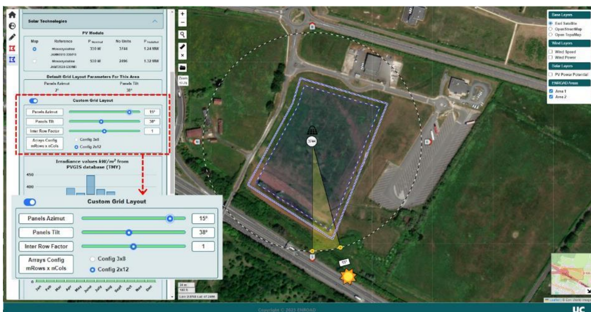
Figure 71.- Recalculation of the number of PV modules after adjusting azimuth and tilt.
