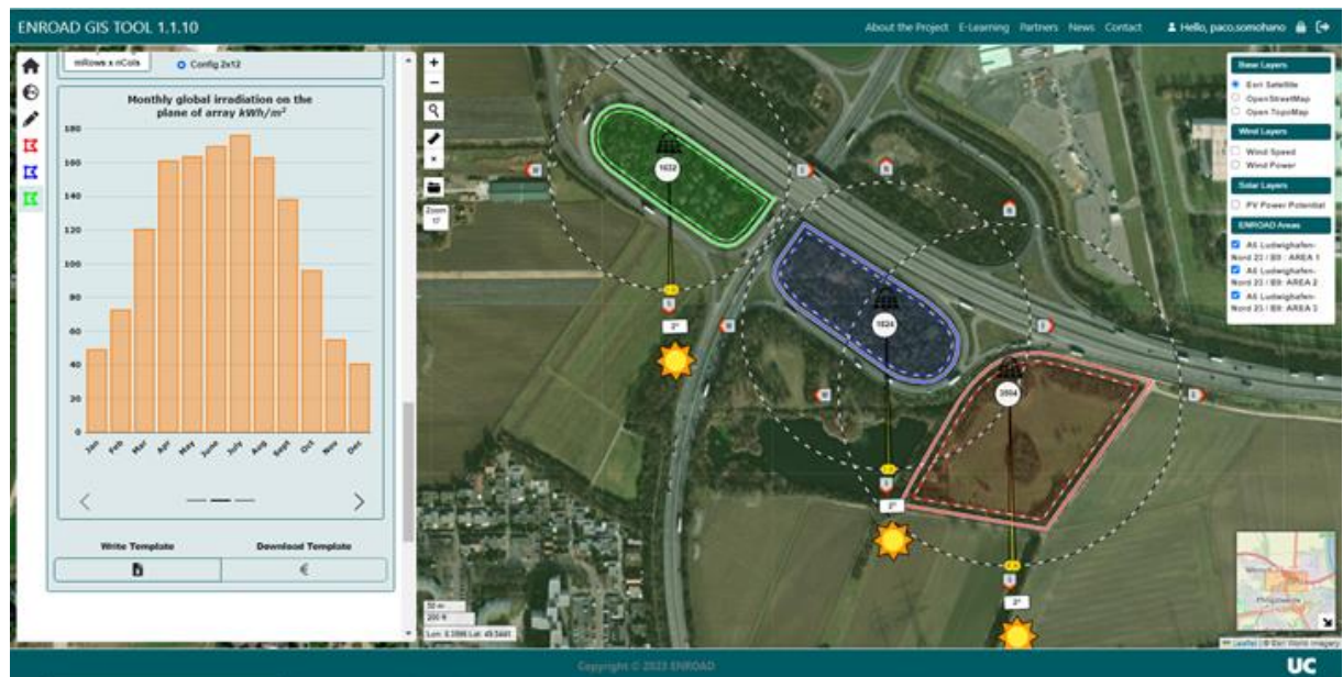
Figure 85.- Configuration of the areas and amount of solar PV panels
