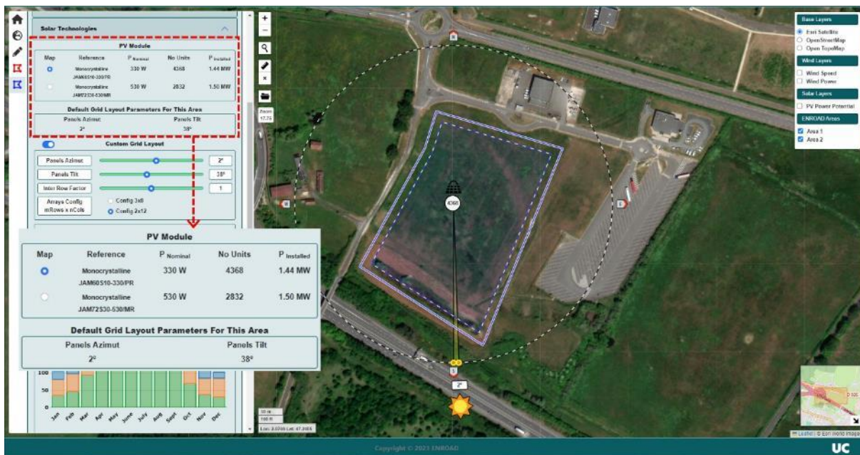
Figure 70.- Calculation by the ENROAD tool of the number of PV modules in the area defined.
