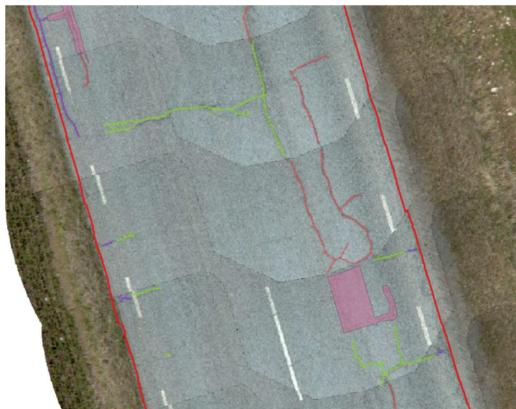
Figure 5: Identification of road defects using AI.
