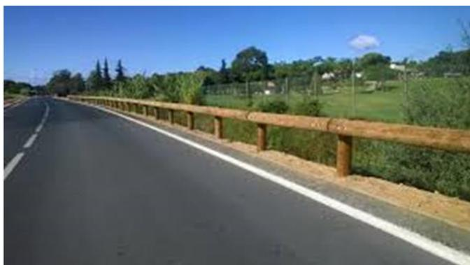
**Description:** timber used for safety barrier.
