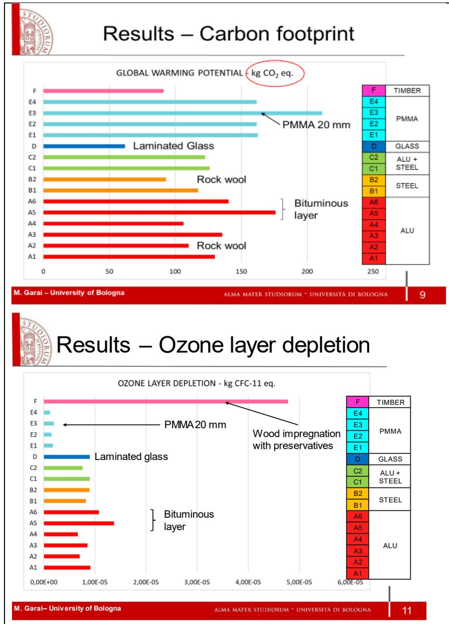
Figure 6: Exemplary results showing how timber and transparent acryl sheets reach opposite scores for carbon footprint and ozone layer depletion.
