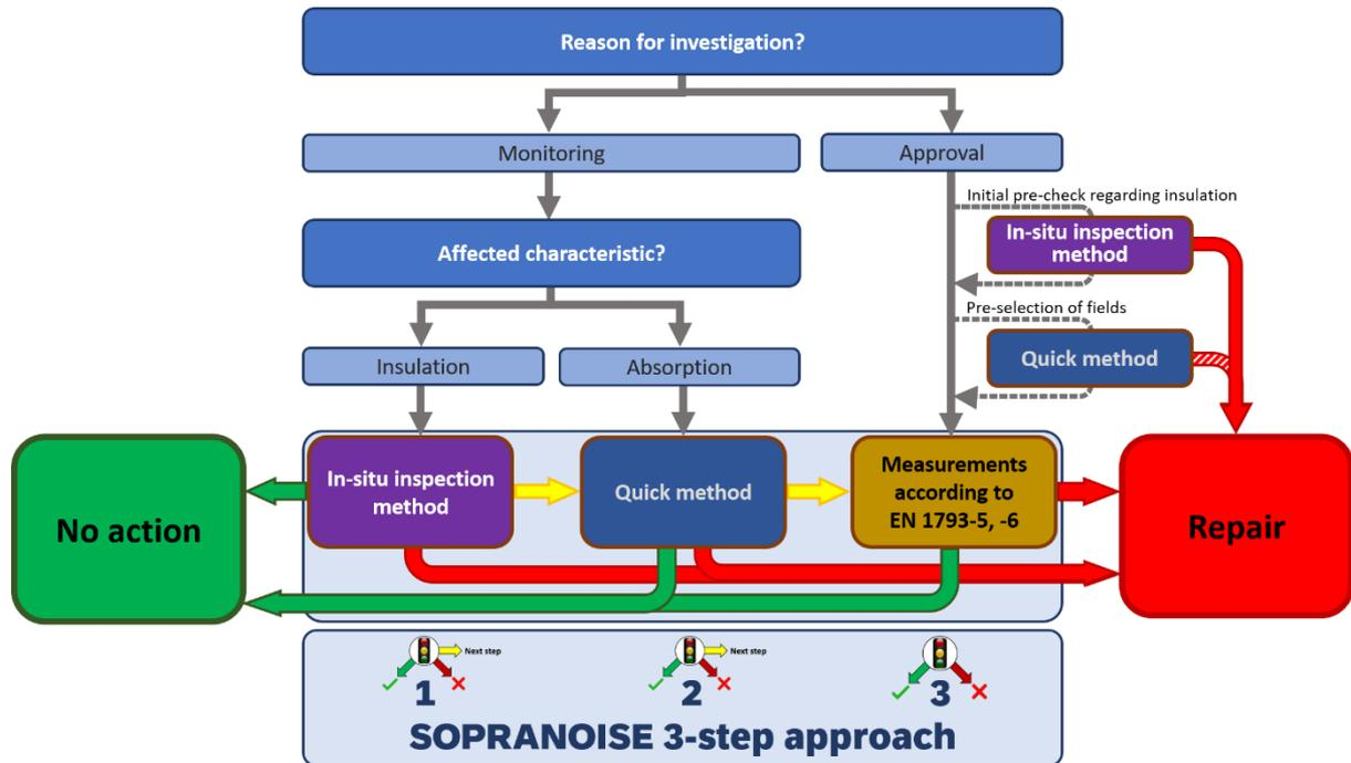
Figure 7: Flow chart visualizing the scope of the SOPRANOISE 3-step approach (see report D5.2 and D3.1 of SOPRANOISE).
