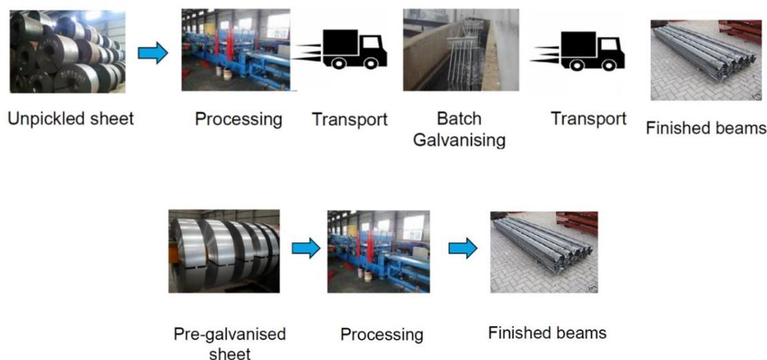
Figure 1: Example of an improved industrial process using pre-galvanized steel (bottom) instead of batch galvanized steel for guard rails (top).
