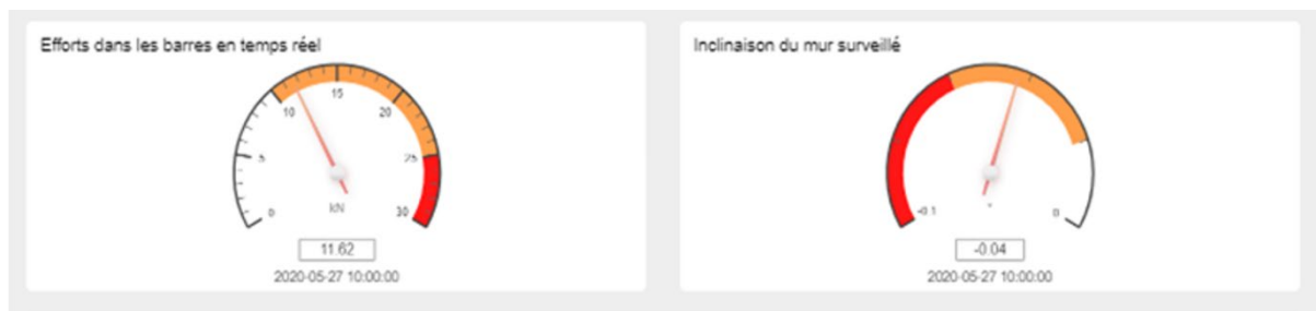
Figure 17 Two alarms set based on the monitored data: (left) alarm on the strain of the rod and (right) alarm on the inclination of the wall.
