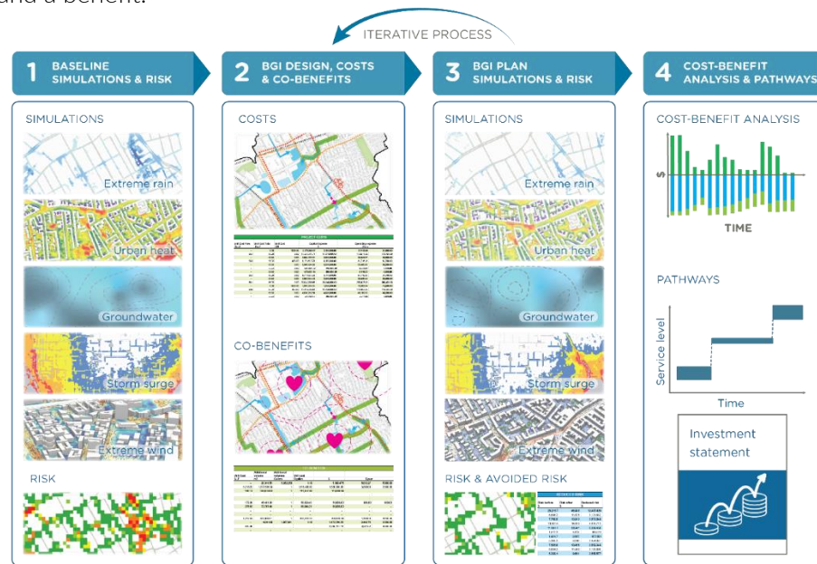
Figure 27. Resilience Planning Approach: an iterative process takes place between the design of Blue-Green Infrastructure (BGI), appraisal of costs, benefits, and co-benefits, leading to a range of investment statements that can guide the decision-making process (Ramboll, 2019).
