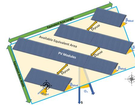
Simulation of relative sun position and self-shading of PV modules
