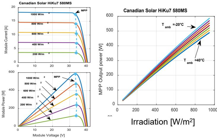
PV module output power as function of PV Irradiance and ambient temperature.
