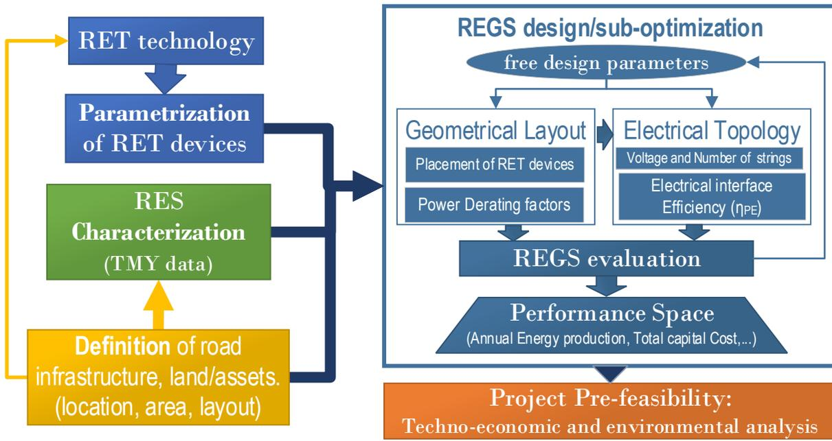
Simplified approach for REGS design and sub-optimization considering geometrical layout and power derating factors ( $\xi_{DF}$ ) related to relative device placement
