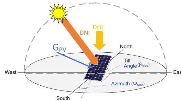
Total PV module irradiation: direct + diffuse
