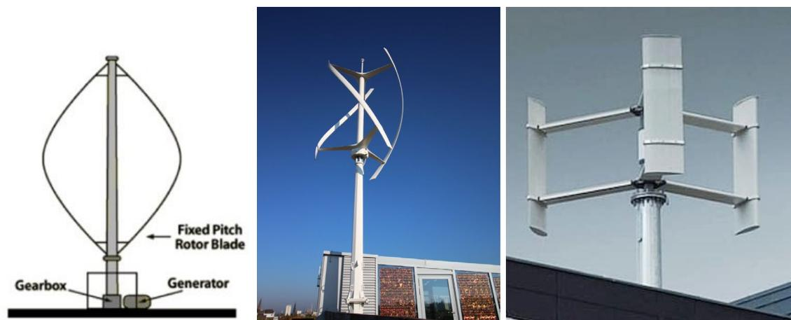
**Figure 3-4 Darrieus VAWT: a) Main components schematic troposkien-type; b) QR6 quiet revolution, a 7kW helical-type darrieus turbine from VWT Power manufacturer (source: <https://vwtpower.com/>); c) Ropatec Maxi 6kW straight-type darrieus turbine from Ropatec manufacturer (source: [www.ropatec.it](http://www.ropatec.it))**
