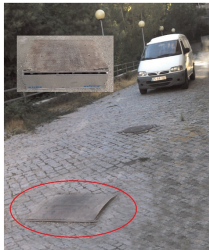
Figure 68.- Field test of electromagnetic harvester prototype by Ferreira y Duarte (2014)
