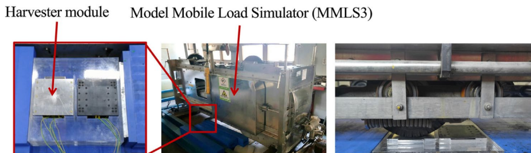
Figure 64.- PEH module tested in the MMLS3. Source: Jung et al. (2017)
