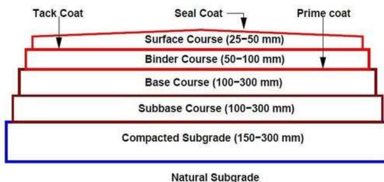
Figure 3 Road material layers from cross section of an Asphalt pavement road 2 .
