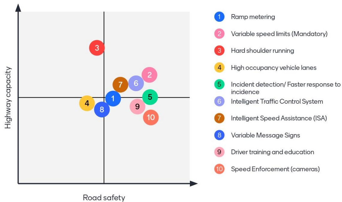
Figure 3: Average voted score representing the effectiveness of various measure in increasing highway capacity and improving traffic safety (Phase 2 workshop)
